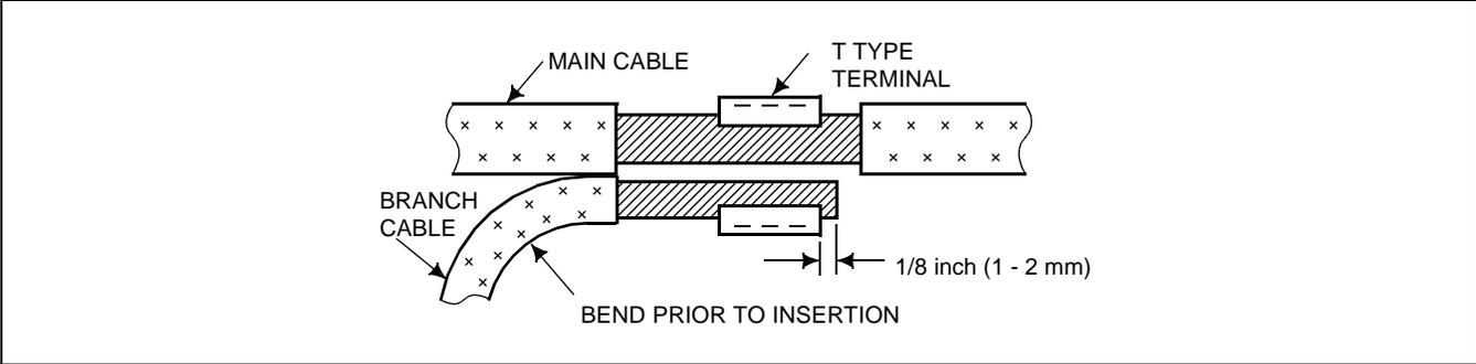
**Figure 008-8 Inserting of Cables into Terminal**
