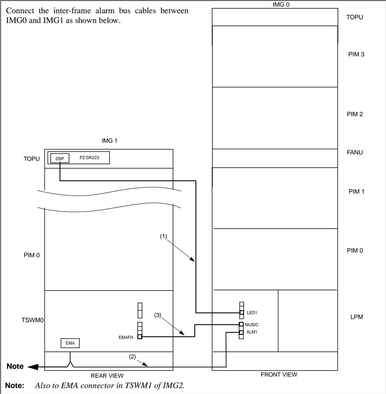
**Figure 010-20 Inter-frame Alarm Bus Cable Connection for IMG0-IMG1**
