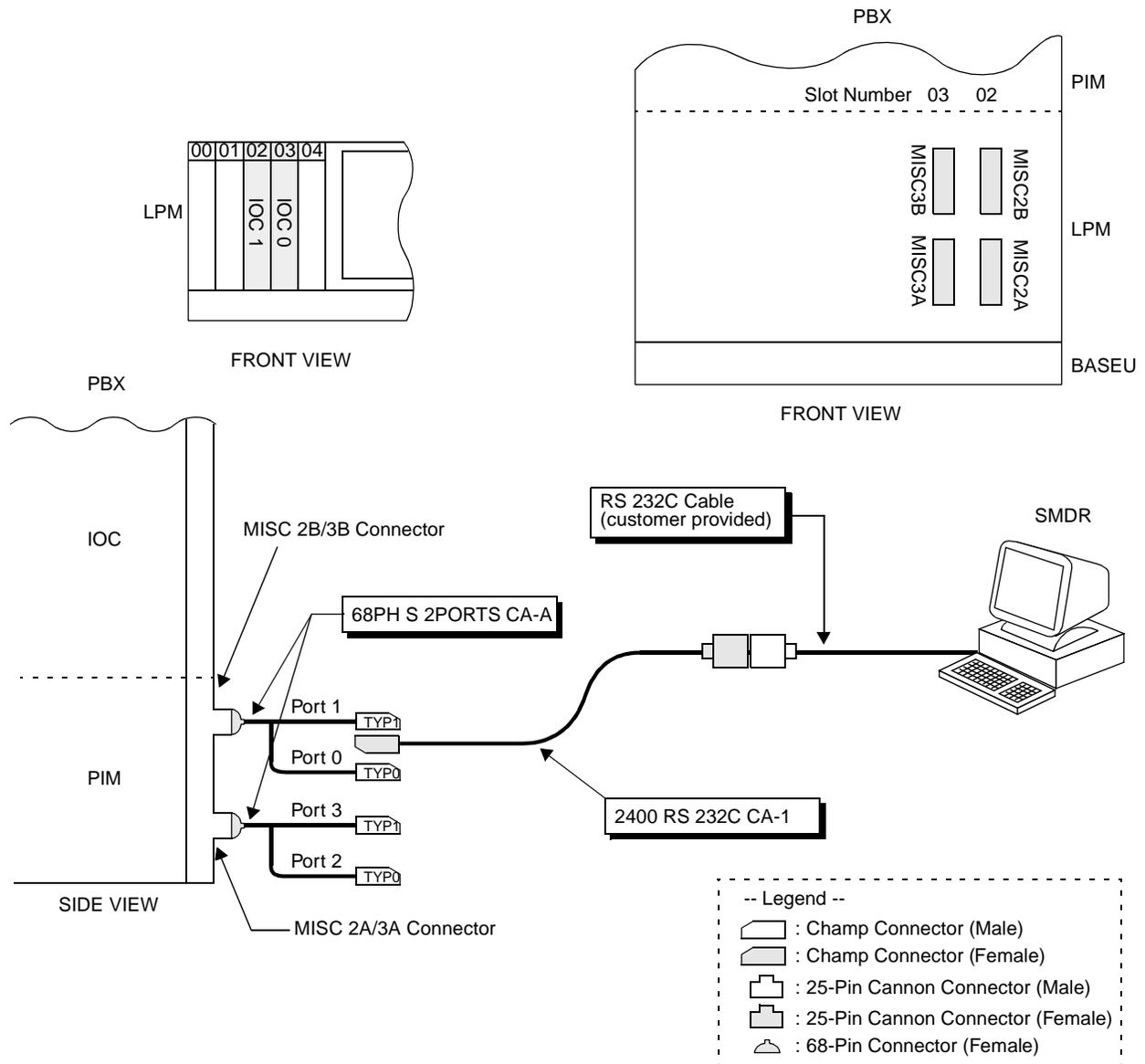
Figure 017-2 Cable Connection Diagram for the SMDR Equipment
