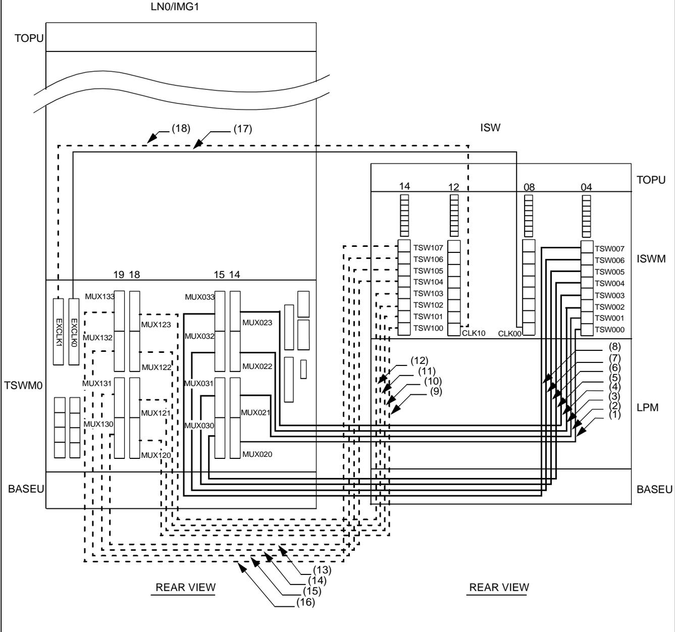
Figure 010-30 Inter-frame Bus Cable Connection for ISW-LN0, IMG1
