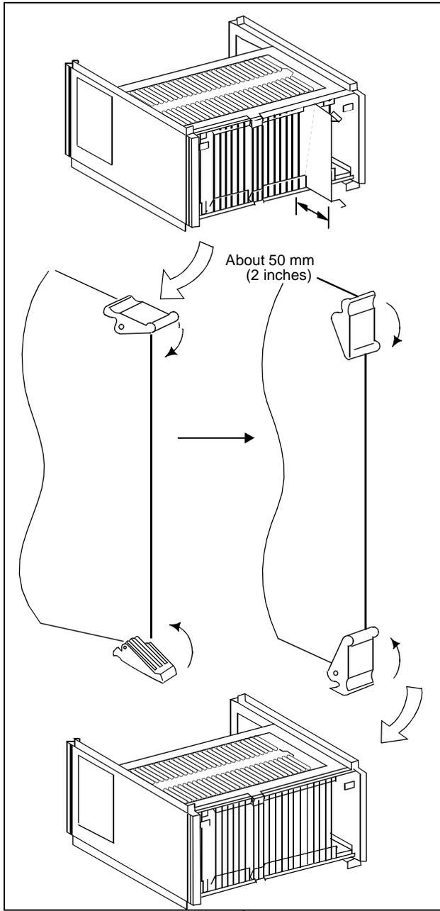
Figure 009-3 Circuit Card Mounting (Partial Insertion)
