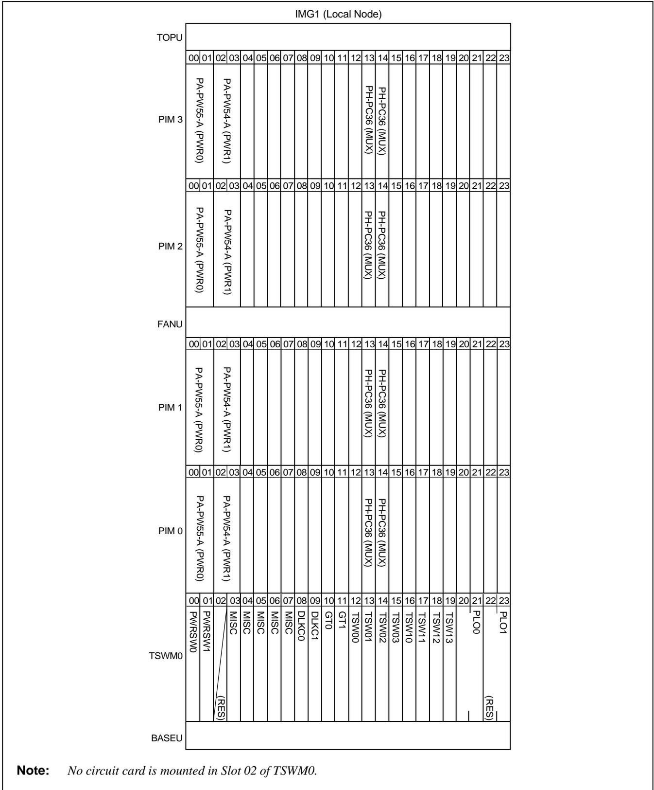
Figure 2-11 Face Layout of IMG1 (Local Node)
