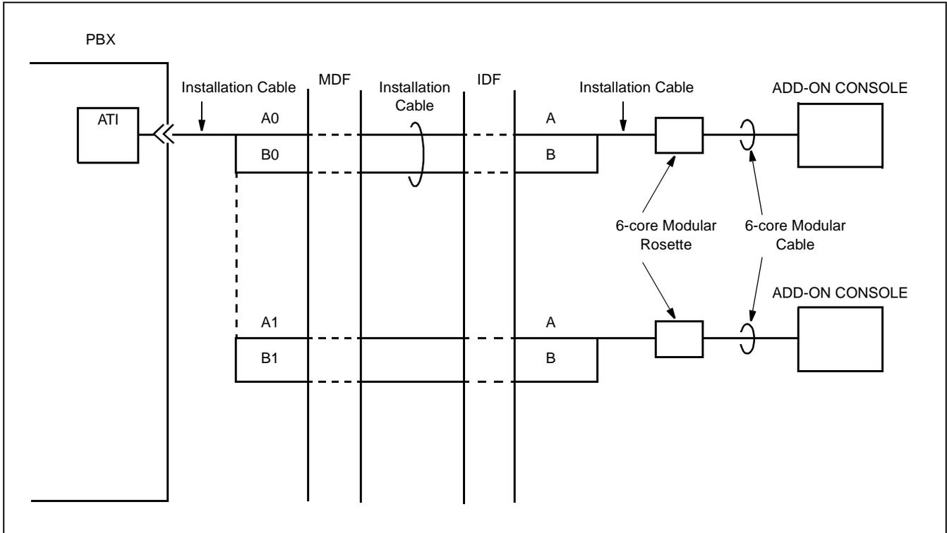
Figure 015-14 Add-On Console Cable Connection Diagram (When using Local Power Supply)
