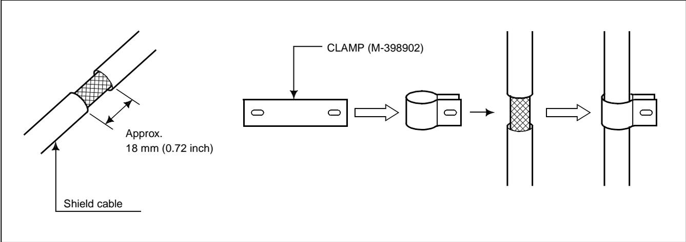
Figure 012-5 Clamp Winding
