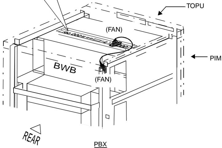
Figure 005-6 Connection of "FAN" Connector Cable (TOPU-PIM)
