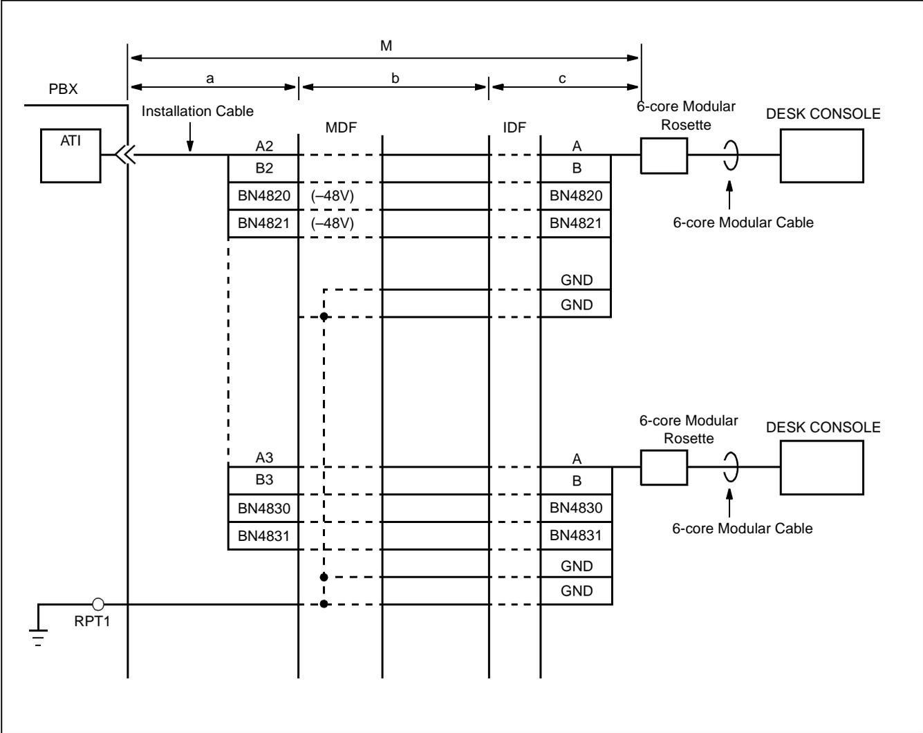
**Figure 015-3 Cable Connection Diagram (When the power is supplied from the PBX)**
