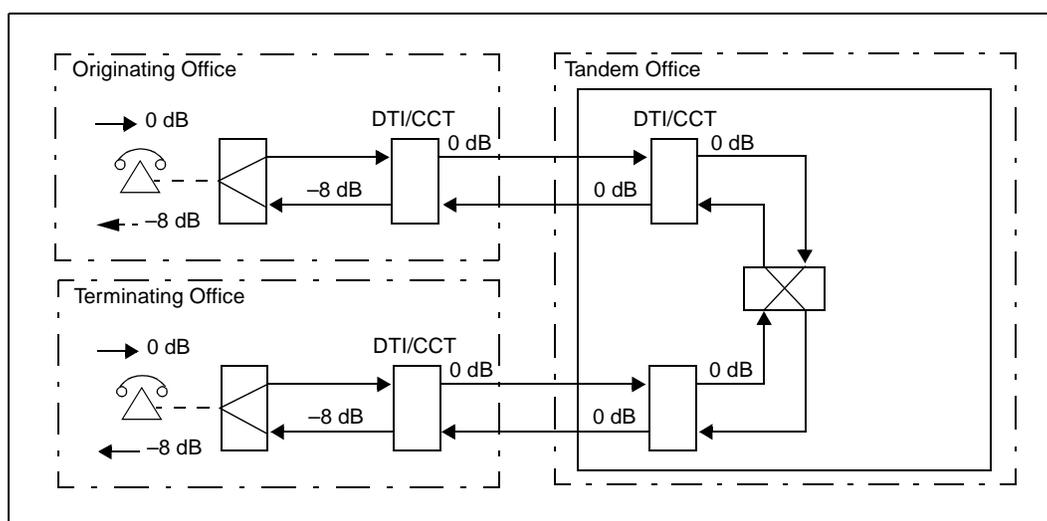
**Figure 049-2 Example of PAD Setting (Digital)**
