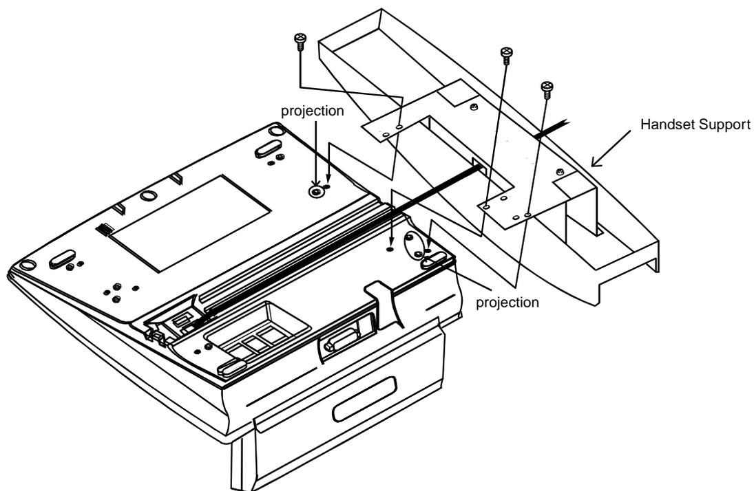
Figure 015-8 Mounting of Handset (Right side of DESK CONSOLE) (Continued)
