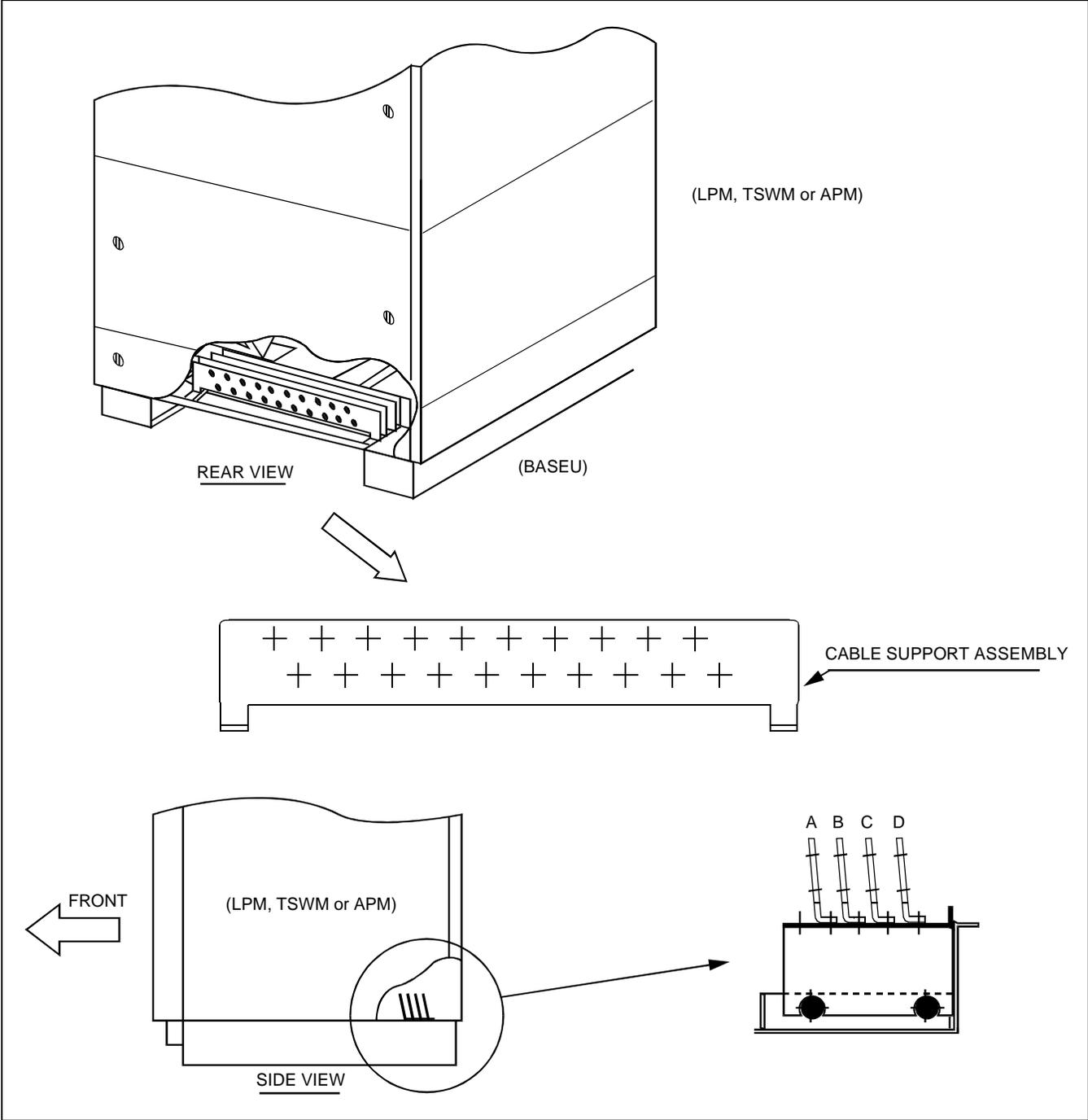
Figure 012-4 Cable Support Assembly
