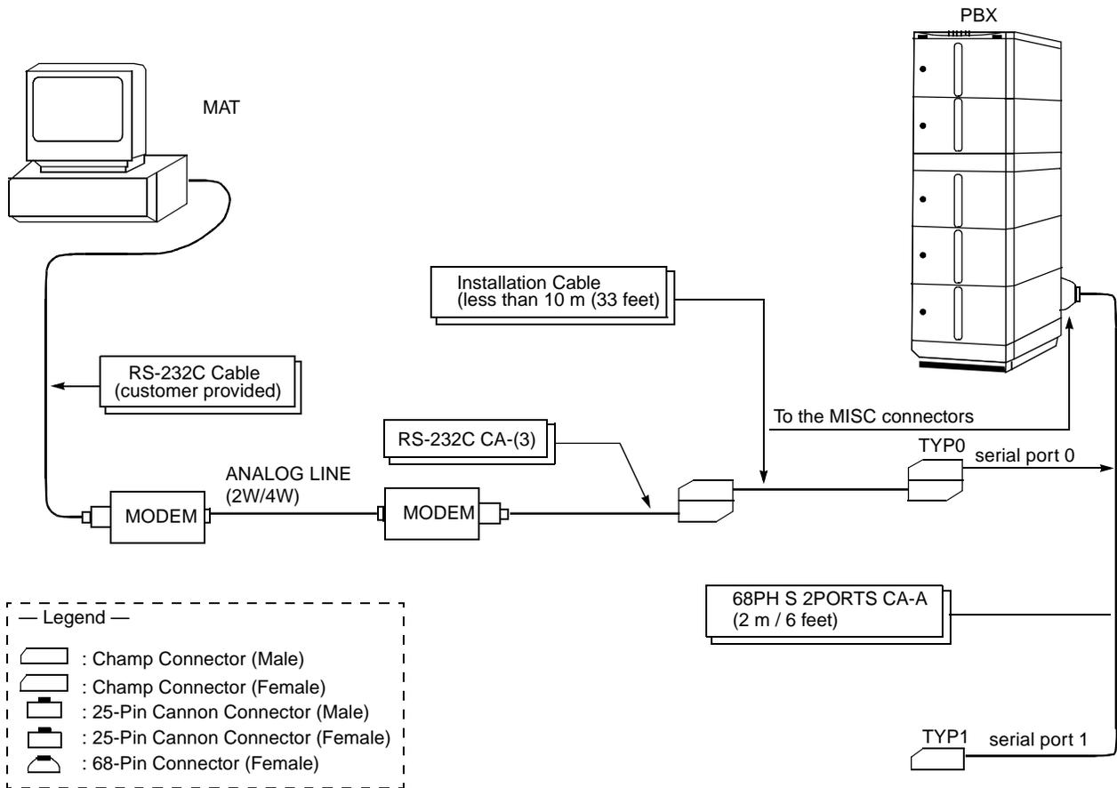
Figure 016-3 Cabling of MAT Using Modems
