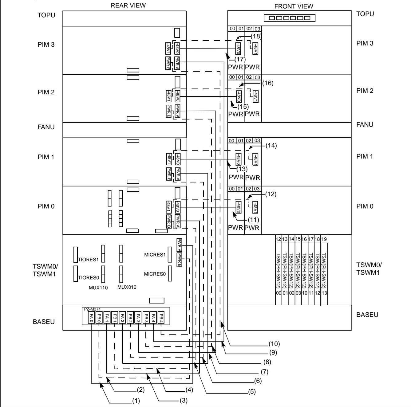
Figure 010-11 Internal Power Cable Connection for IMG1/2
