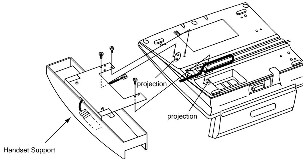
**Figure 015-7 Mounting of Handset (Left side of DESK CONSOLE) (Continued)**
