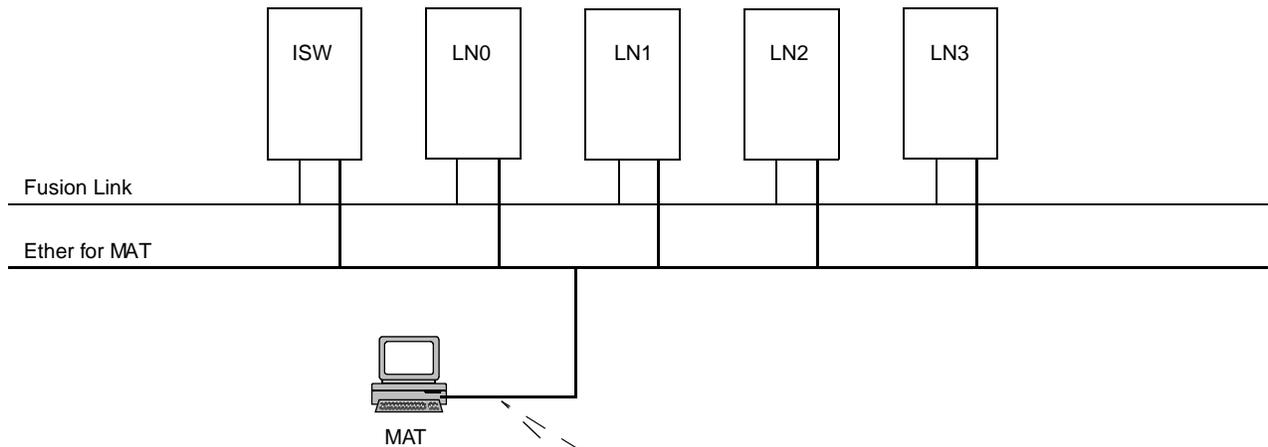
This figure is an example where a MAT is connected to LN1 via the 10 BASE-T cables (Ethernet). As seen from this, the MAT, a single terminal connected to the Ether, can control the whole system status, thus capable of a single-point entry to each LN and ISW.
