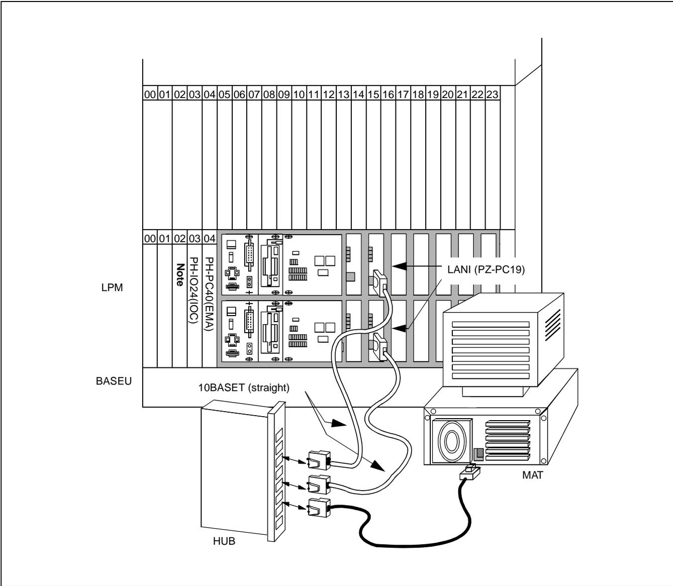
Figure 016-1 Cabling of MAT when Using Ethernet
