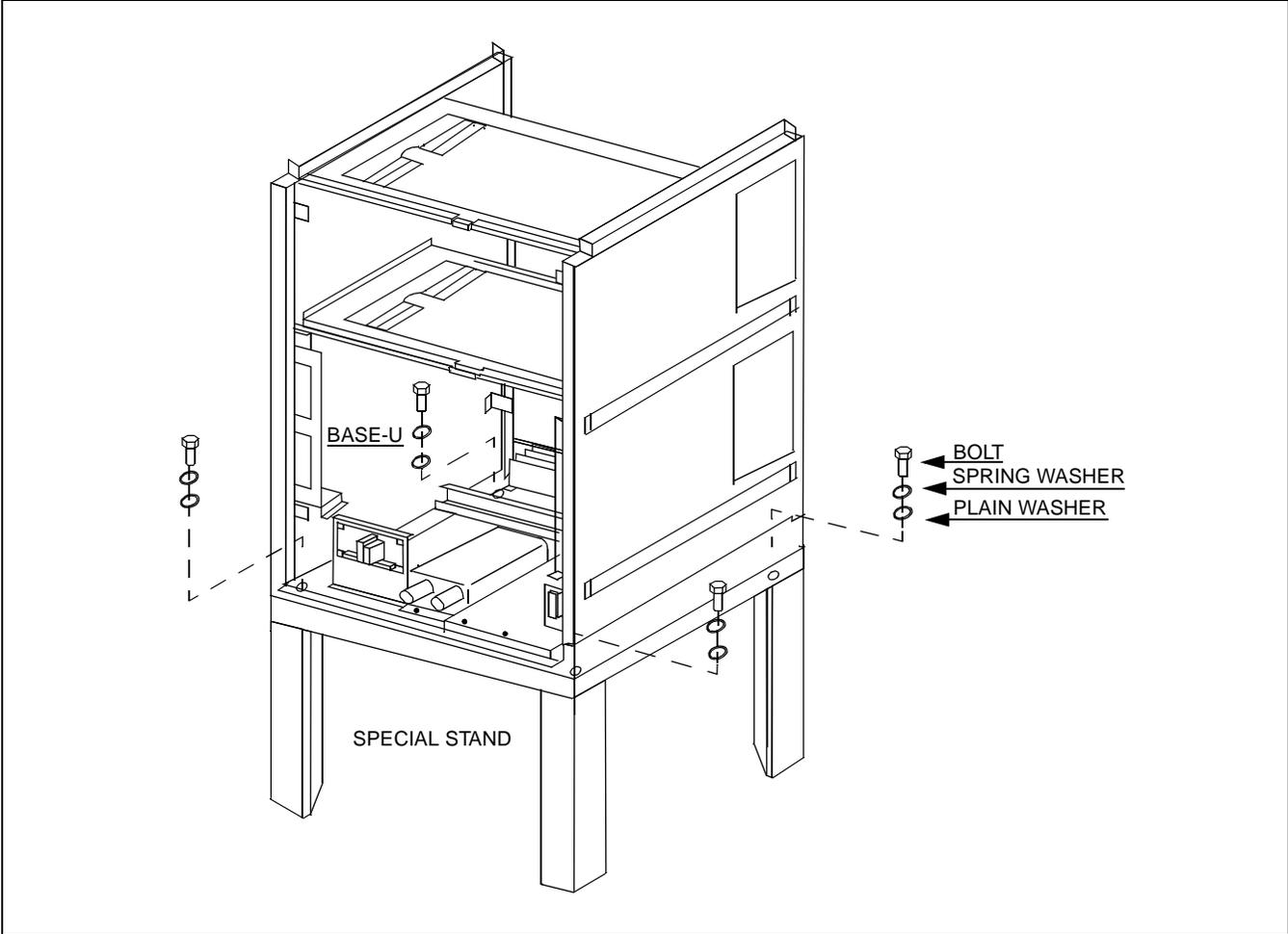
**Figure 004-4 Setting the BASEU via Special Stand**
