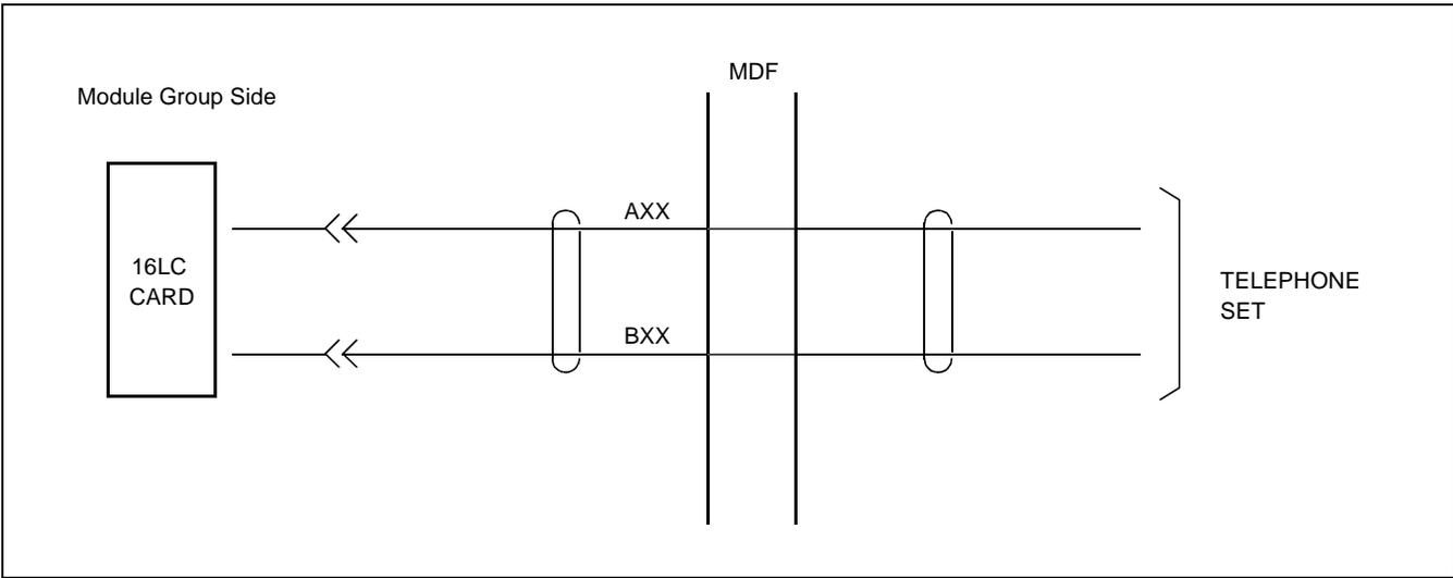
**Figure 014-1 Cross Connection of Stations**
