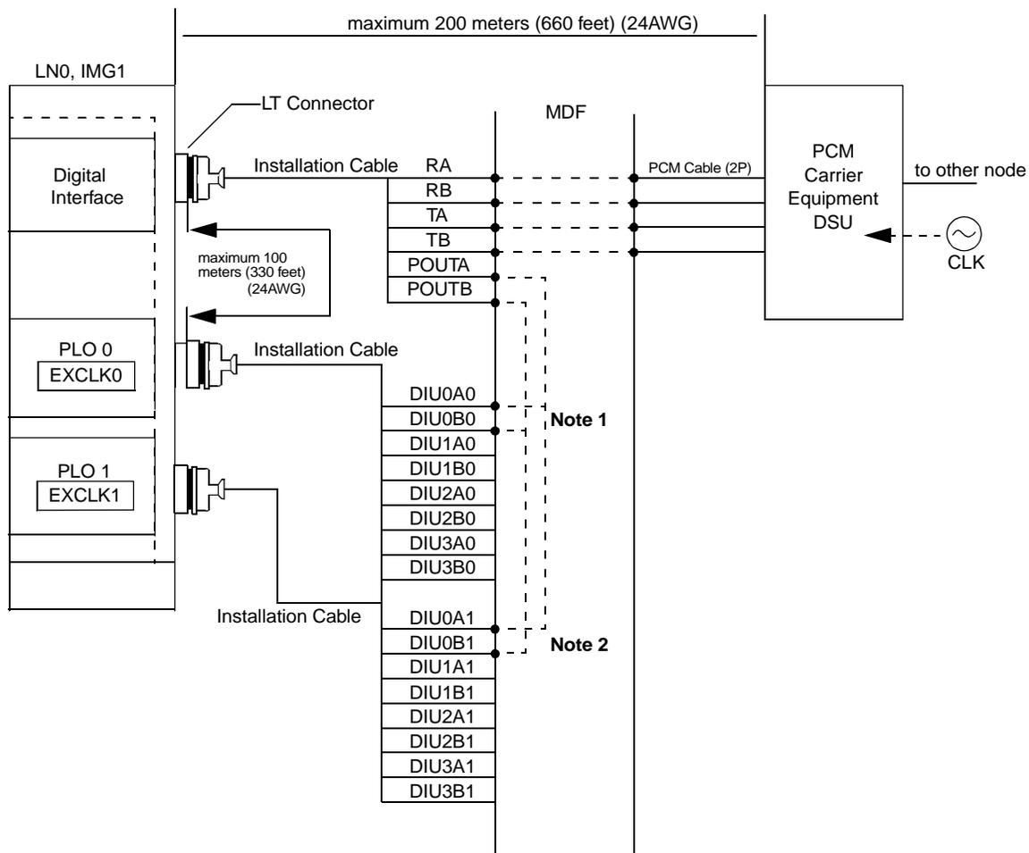
**Note 1:** PLO has a maximum of four inputs. DIU0xx leads are used for the 1st clock distribution routes. Thus, DIU3xx leads are used for the 4th. The first input has the highest priority.
