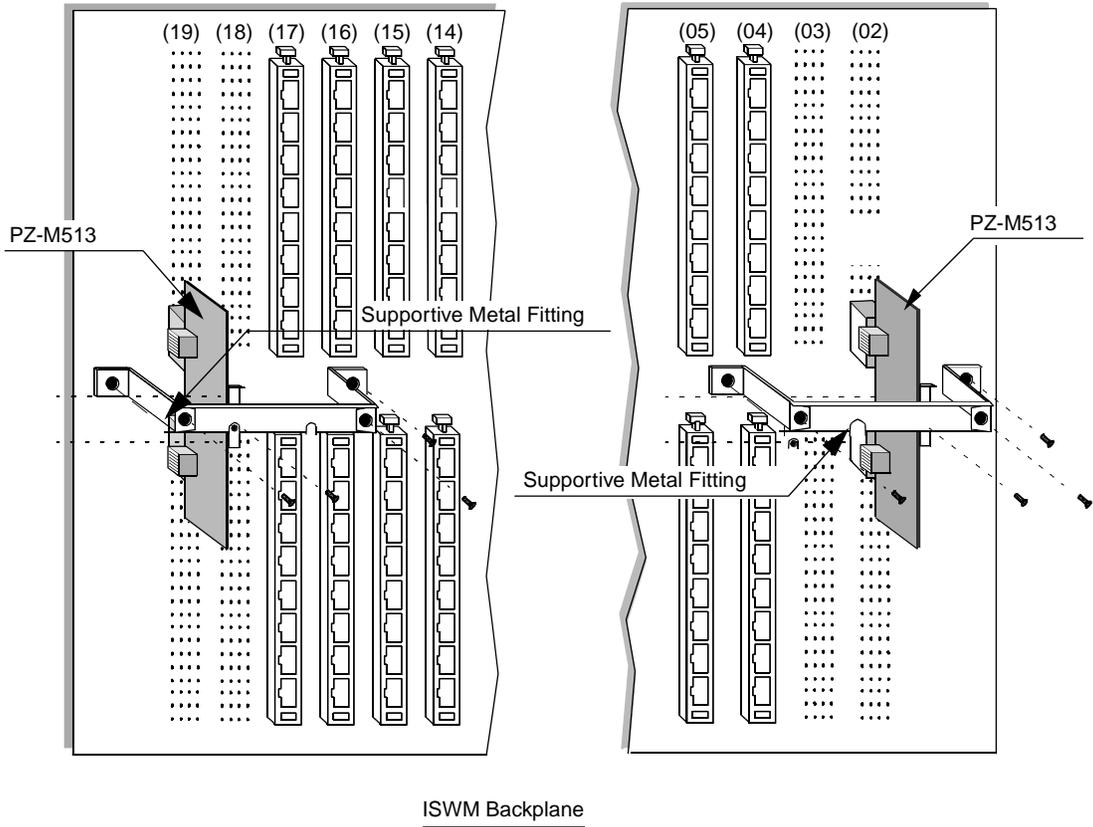
**Figure 010-3 Details on Fastening PZ-M513 by Metal Fittings (ISWM Backplane)**
