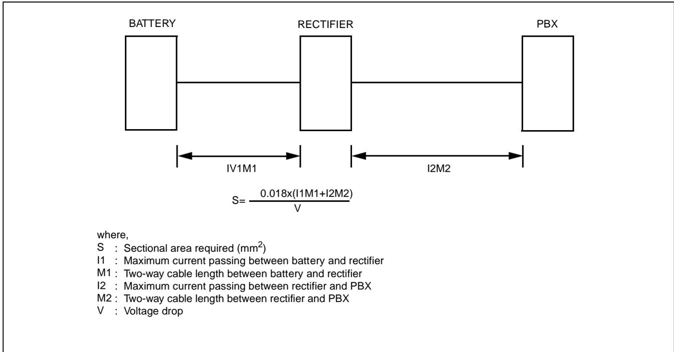
**Figure 2-22 Calculation Method for Sectional Area**
