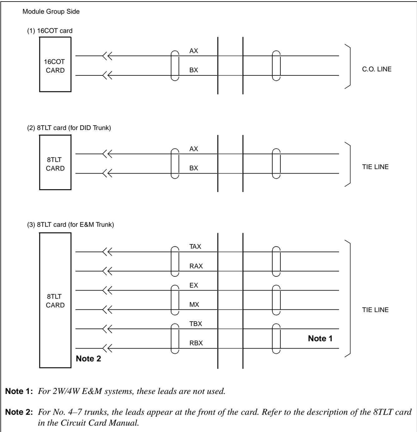
Figure 014-2 Cross Connection of Trunks (C.O. Lines and Tie Lines)
