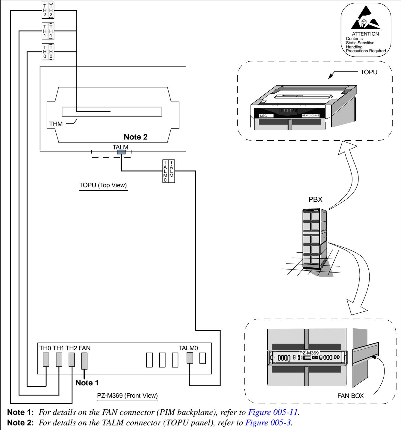
**Figure 005-10 Cable Connections for FANU in FAN BOX**
