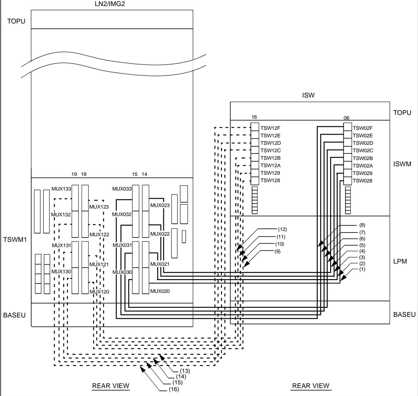
Figure 010-35 Inter-frame Bus Cable Connection for ISW-LN2, IMG2
