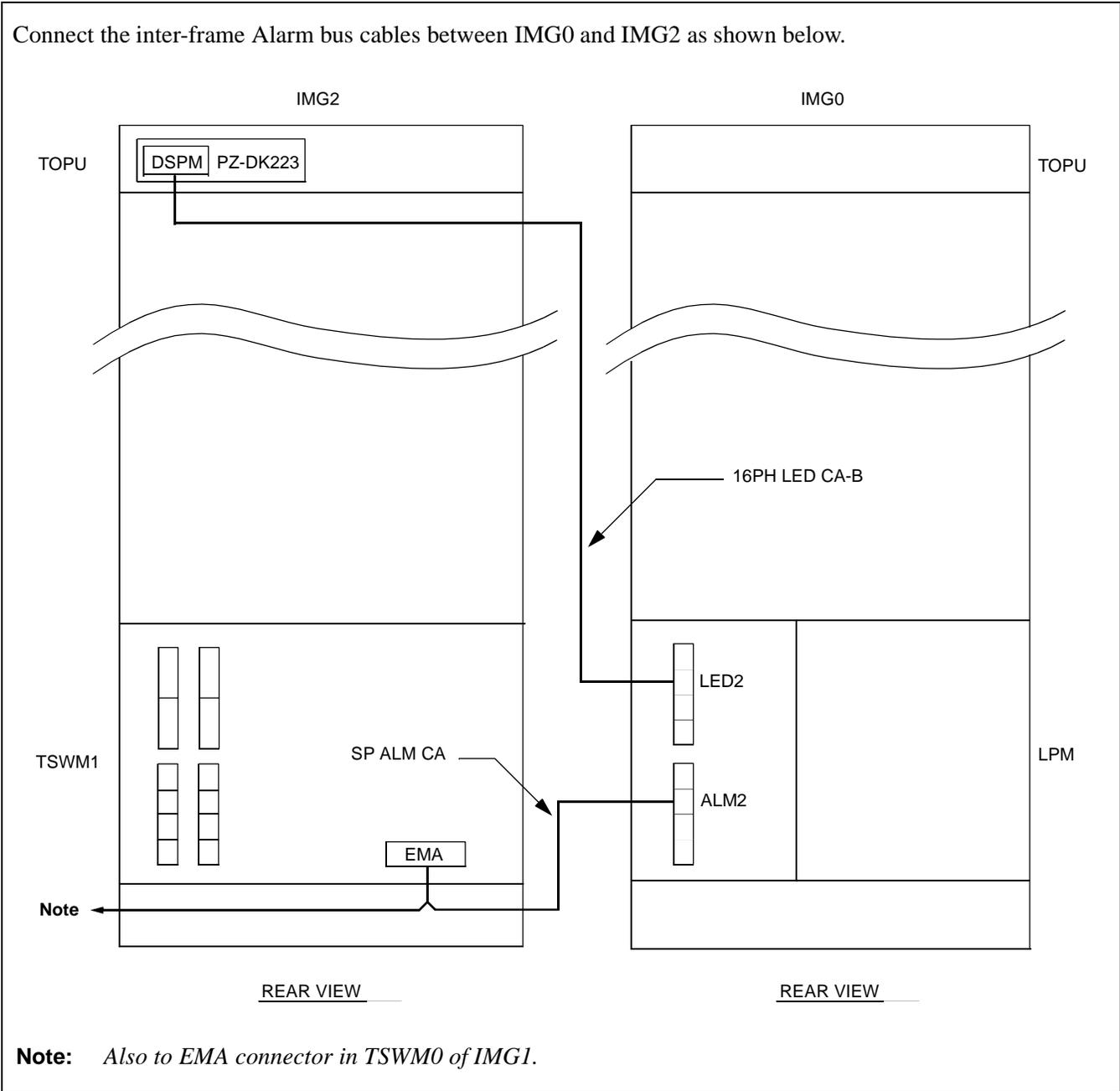
Figure 010-22 Inter-frame Alarm Bus Cable Connection for IMG0-IMG2
