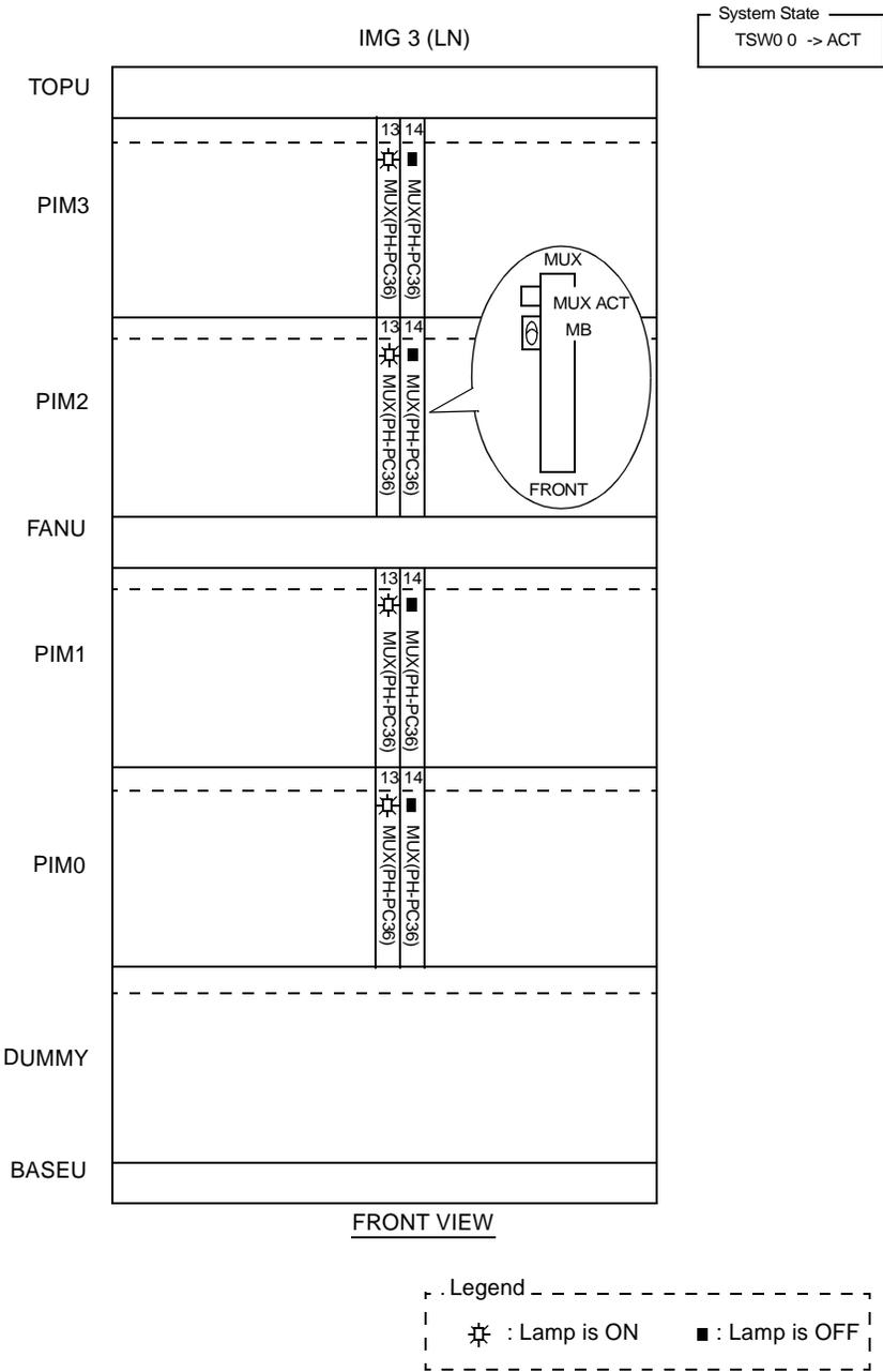
Figure 021-4 LED Indications of IMG3 in Normal Operation (example)
