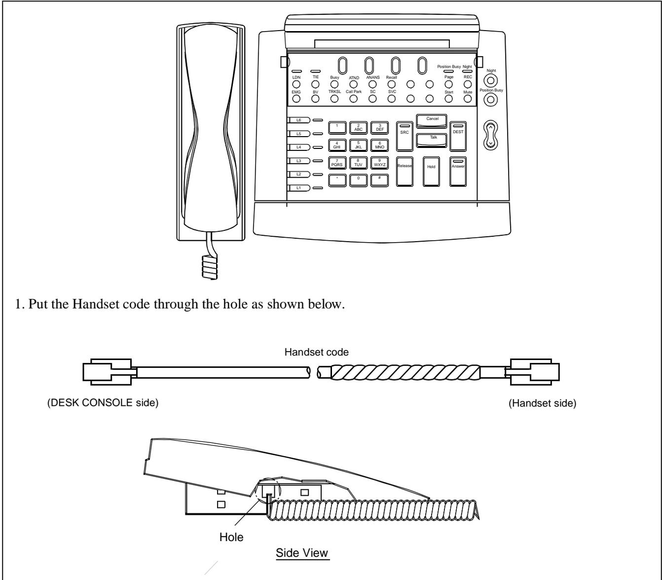
**Figure 015-7 Mounting of Handset (Left side of DESK CONSOLE)**
