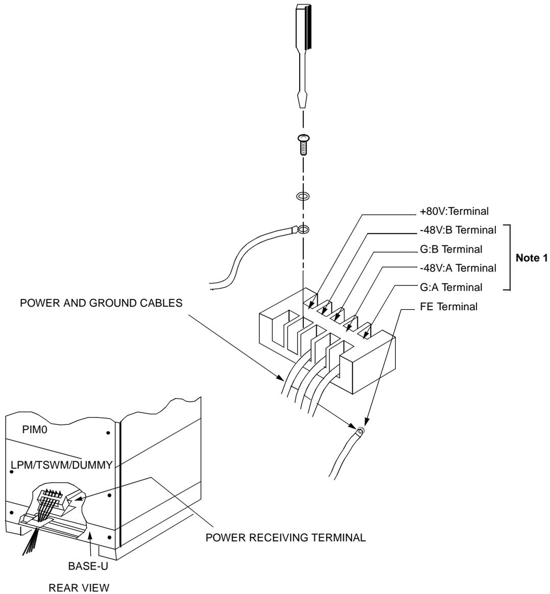
**Note 1:** For 1/2 PIM configuration, connect the cable only to the A terminal.
