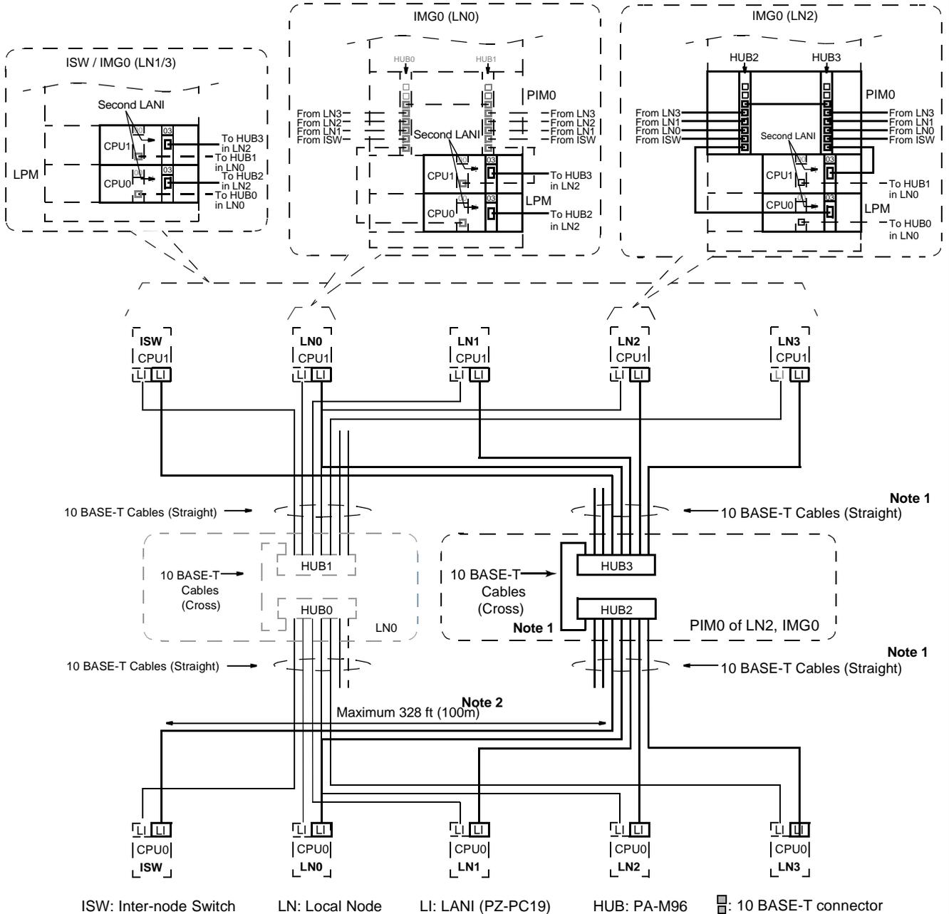
**Figure 2-6 Details on Ether Cable Connections (Establishment of Fusion Link) (2/2)**
