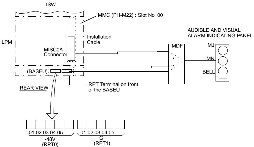
**Figure 014-5 Connection of Alarm Indicating Panel**
