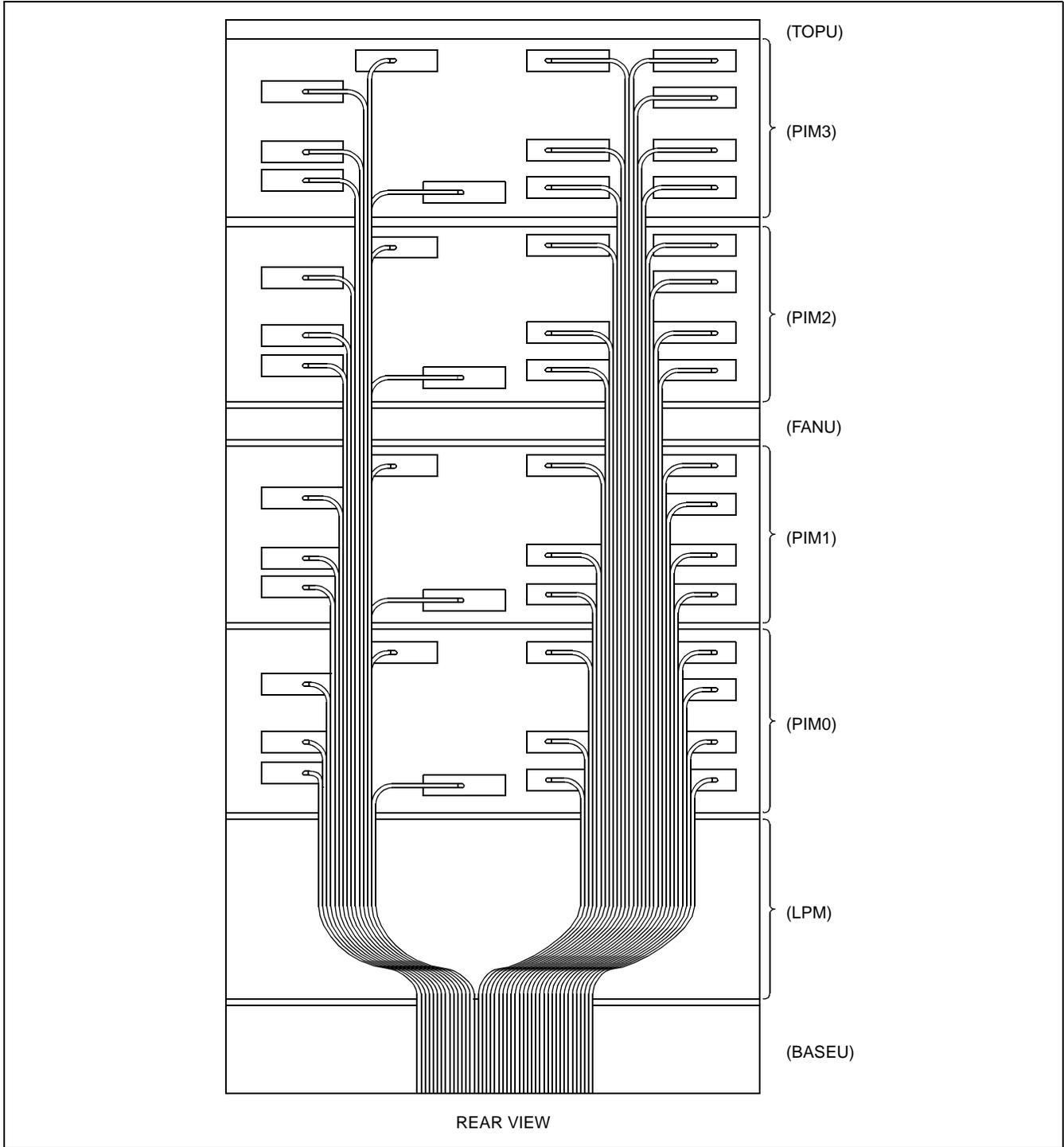
**Figure 012-1 LT Cable Routing**
