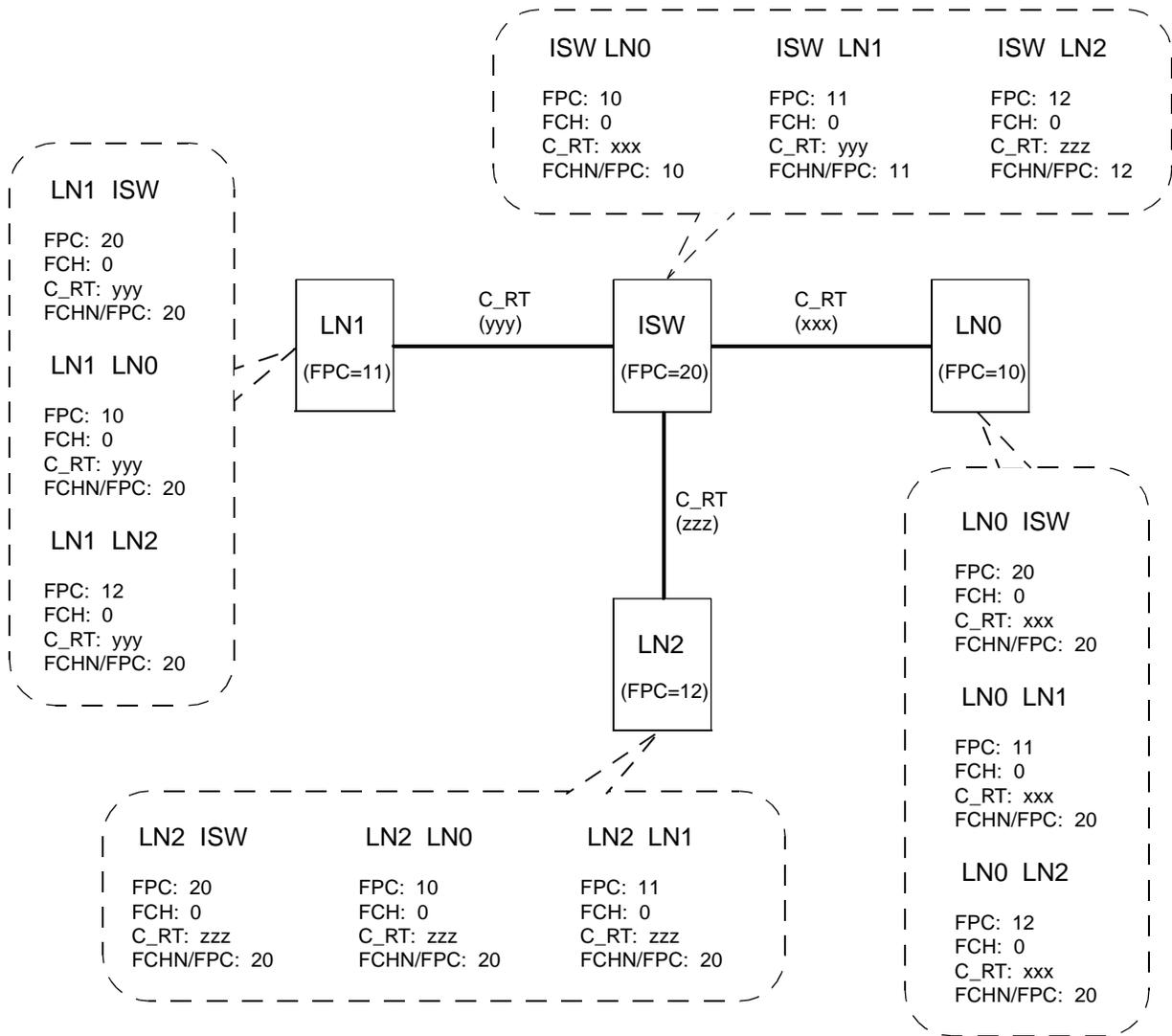
**Figure 020-1 Example of Connection Route Data Assignment (AFPC Command)**
