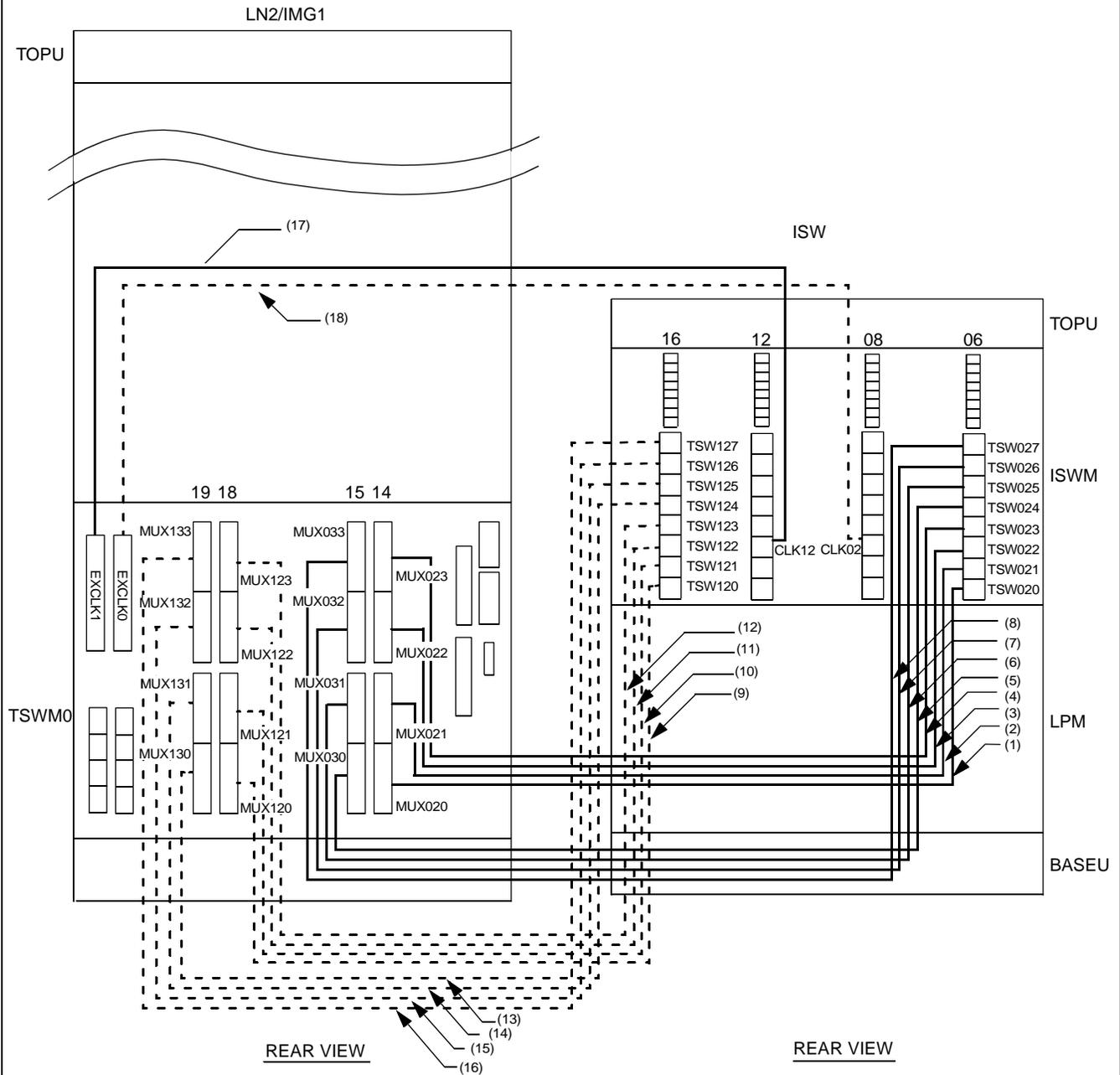
Figure 010-34 Inter-Frame Bus Cable Connection for ISW-LN2, IMG1
