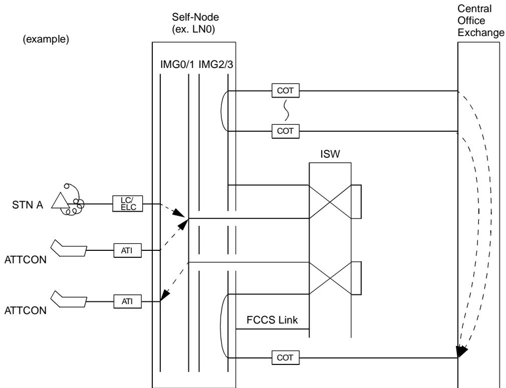
Figure 042-1 Overall Test for C.O. Line Outgoing Call (1/2)
