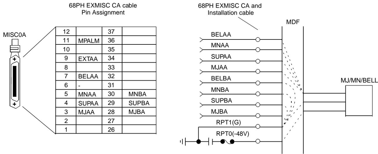
Figure 014-5 Connection of Alarm Indicating Panel (Continued)
