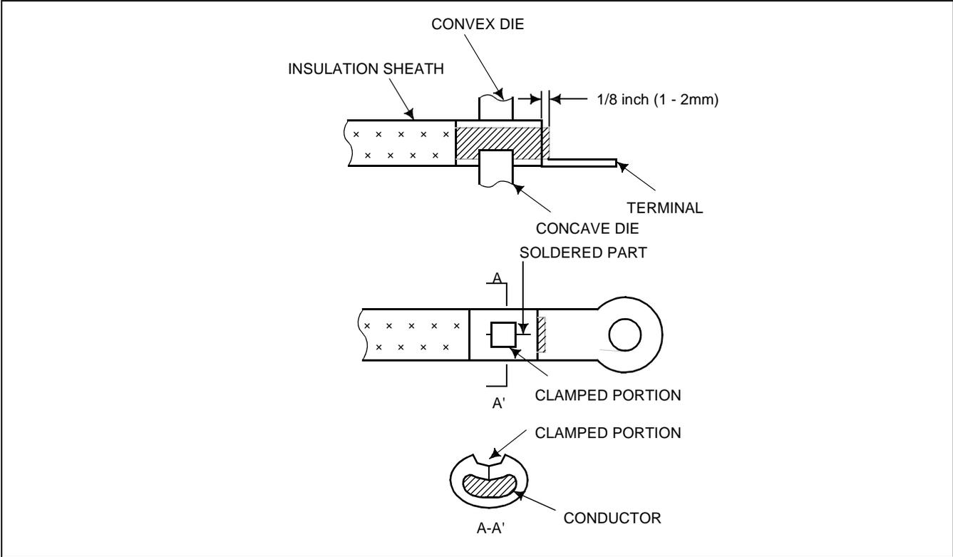
**Figure 008-6 Clamping Method**
