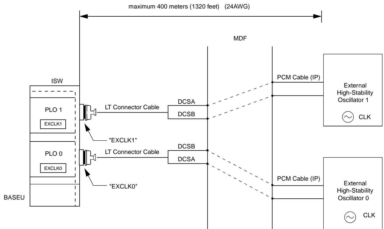
**Note:** This diagram shows connections for a system having dual PLOs.
