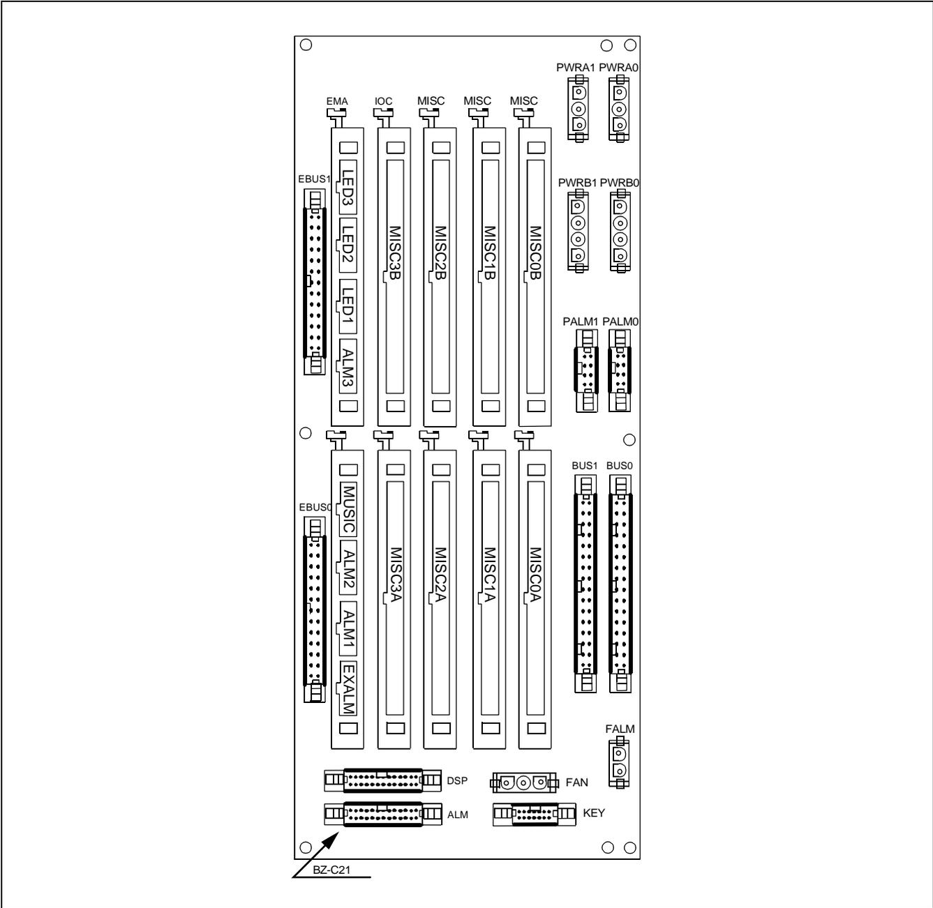
Figure 010-4 Location of Connectors on the LPM Backplane
