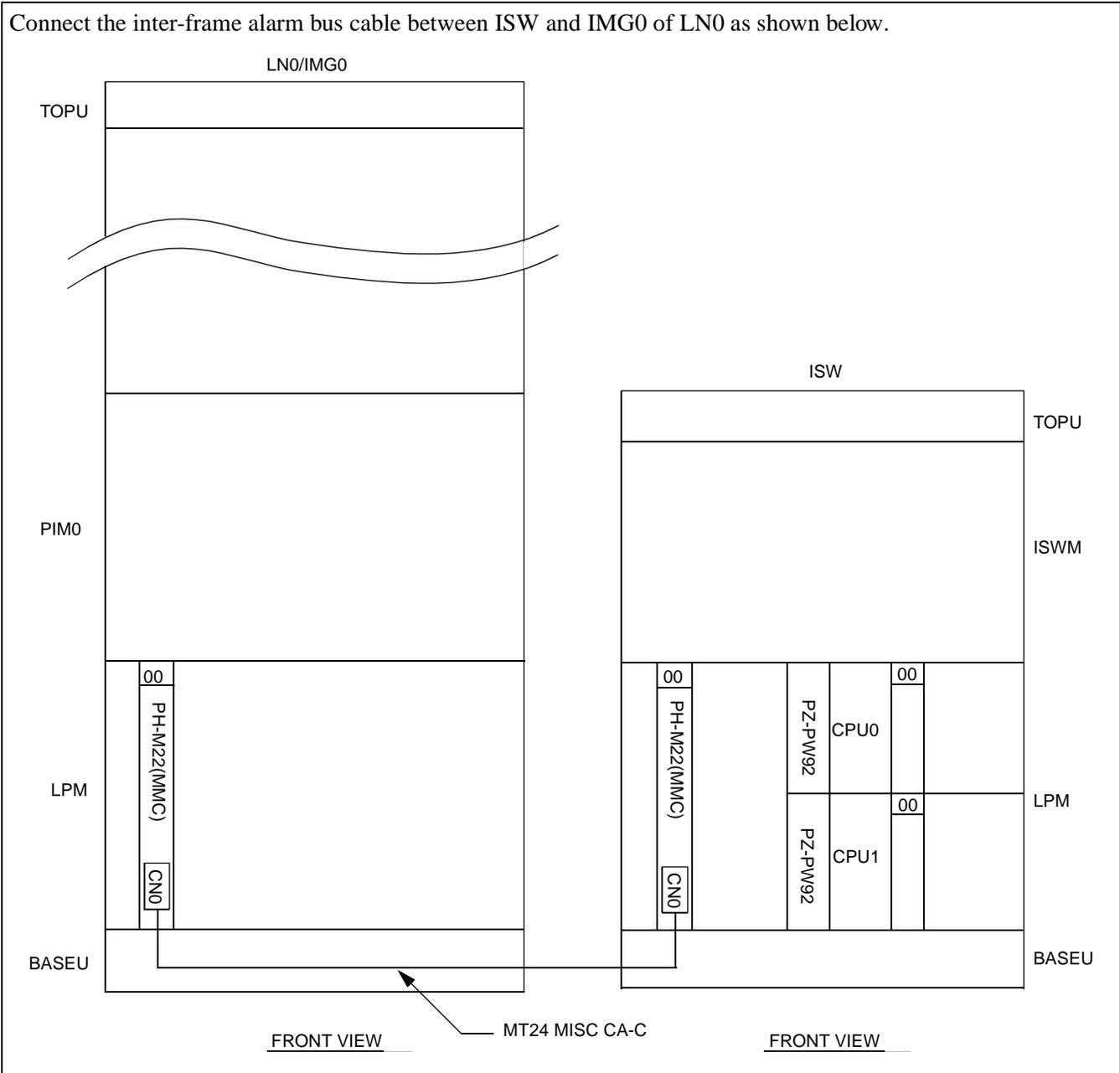
Figure 010-26 Inter-frame Cable Connection for ISW-LN0, IMG0
