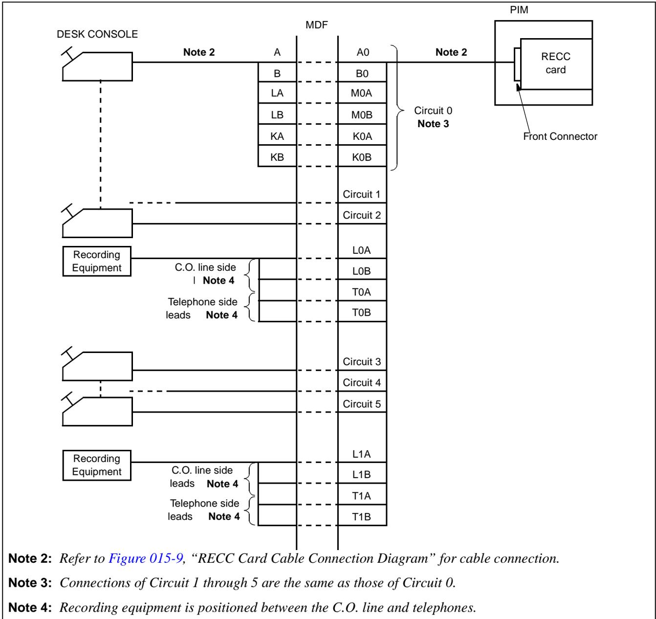
**Figure 015-10 Three DESK CONSOLES and One Recording Equipment**
