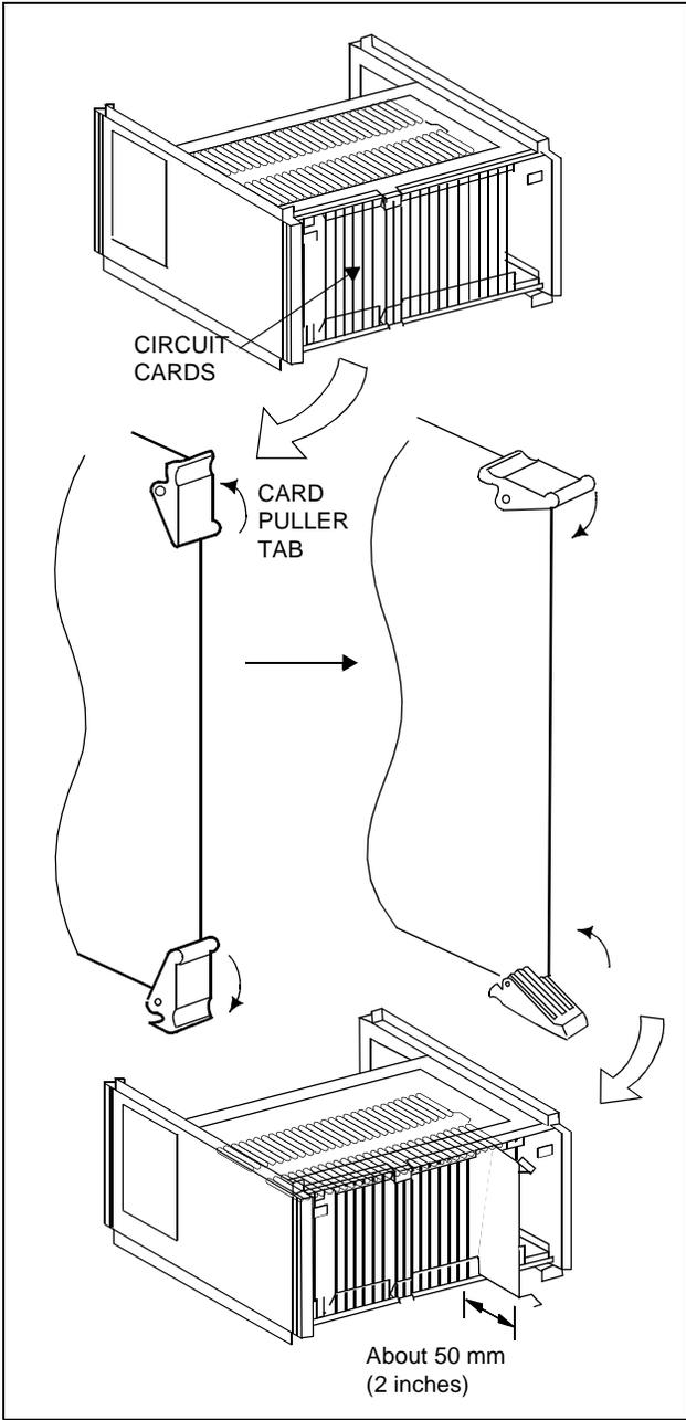
Figure 009-2 Extraction of Circuit Cards
