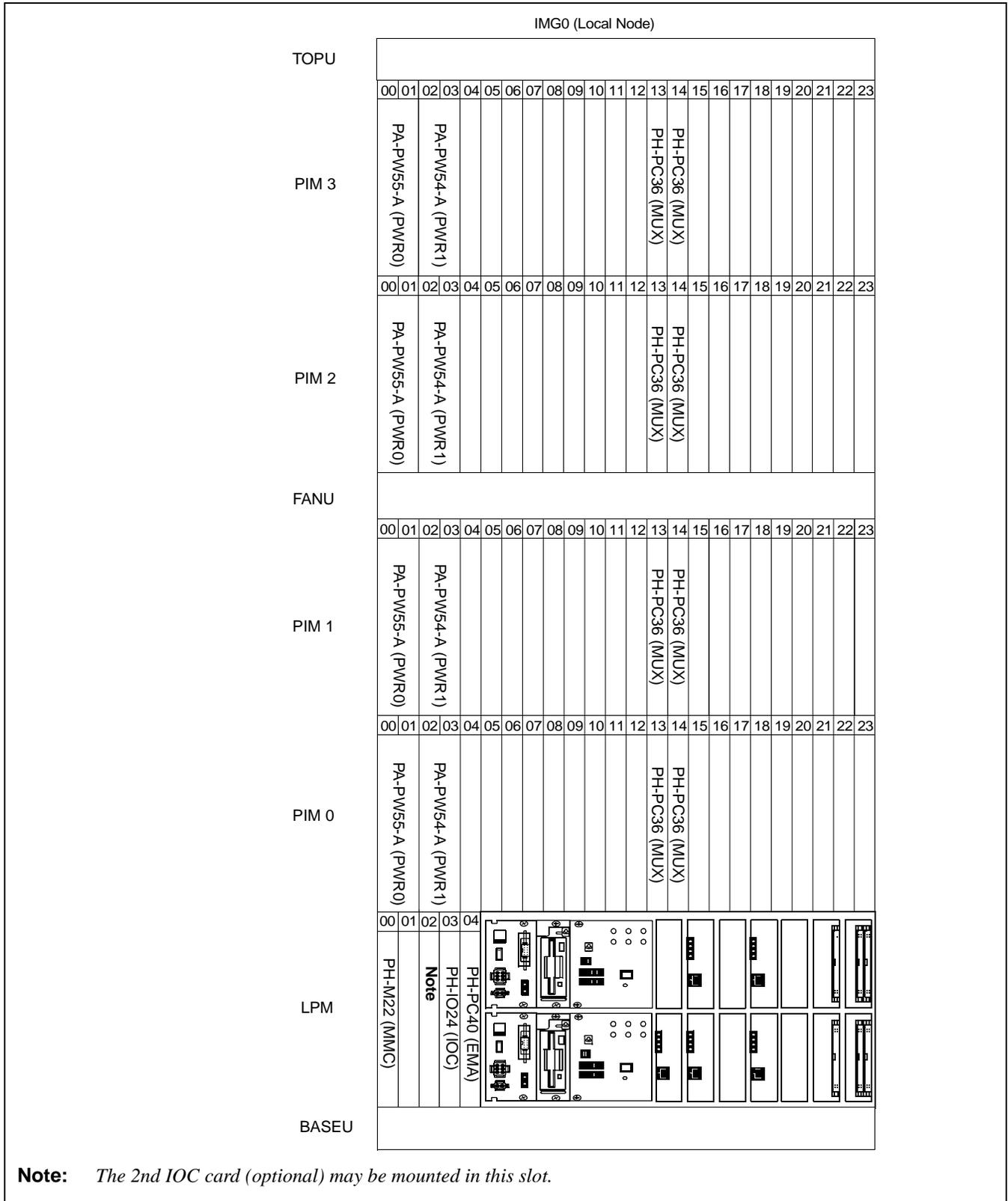
Figure 2-10 Face Layout of IMG0 (Local Node)
