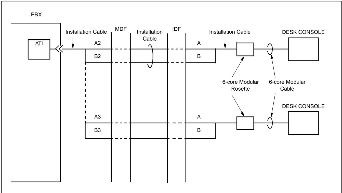
**Figure 015-4 Cable Connection Diagram (When using Local Power Supply)**
