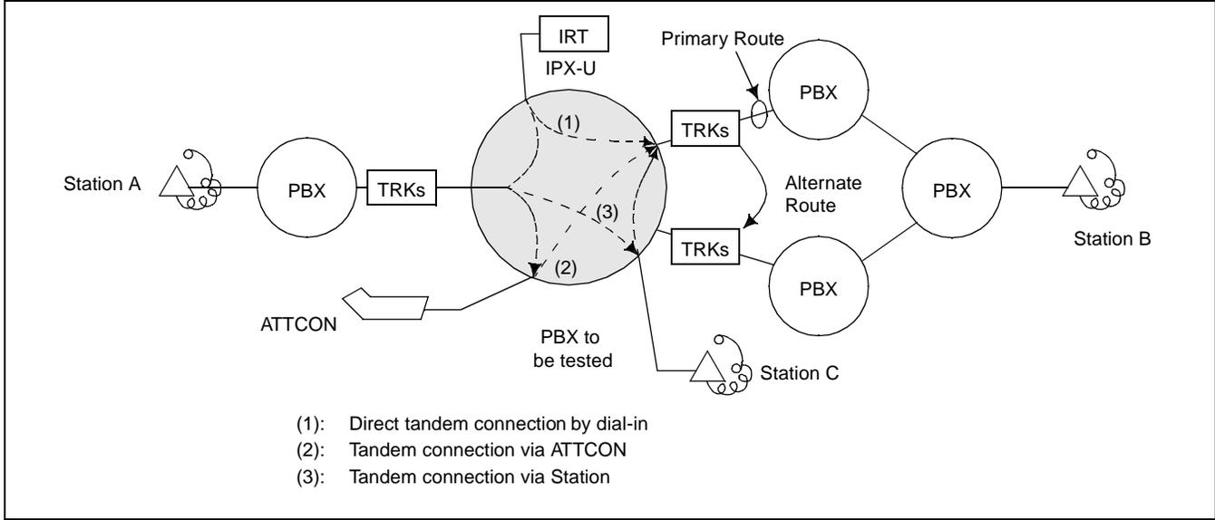
**Figure 048-1 Test of Tandem Connection to Tie Line**
