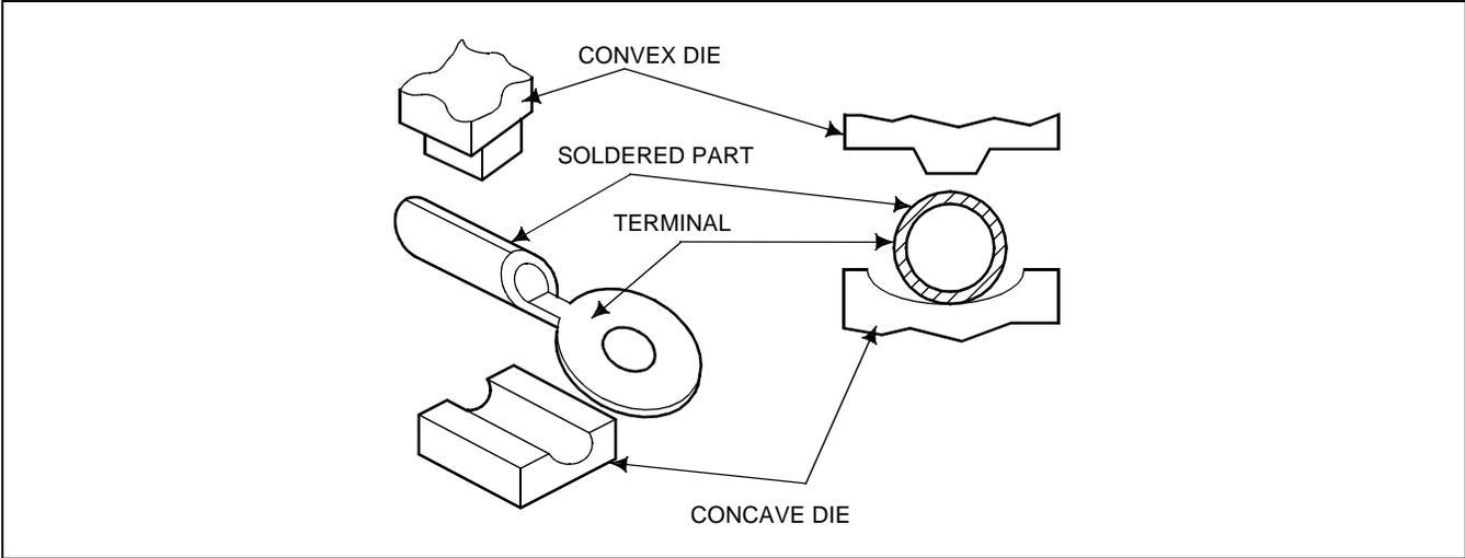
**Figure 008-5 Placing the Clamp Terminal on the Die**
