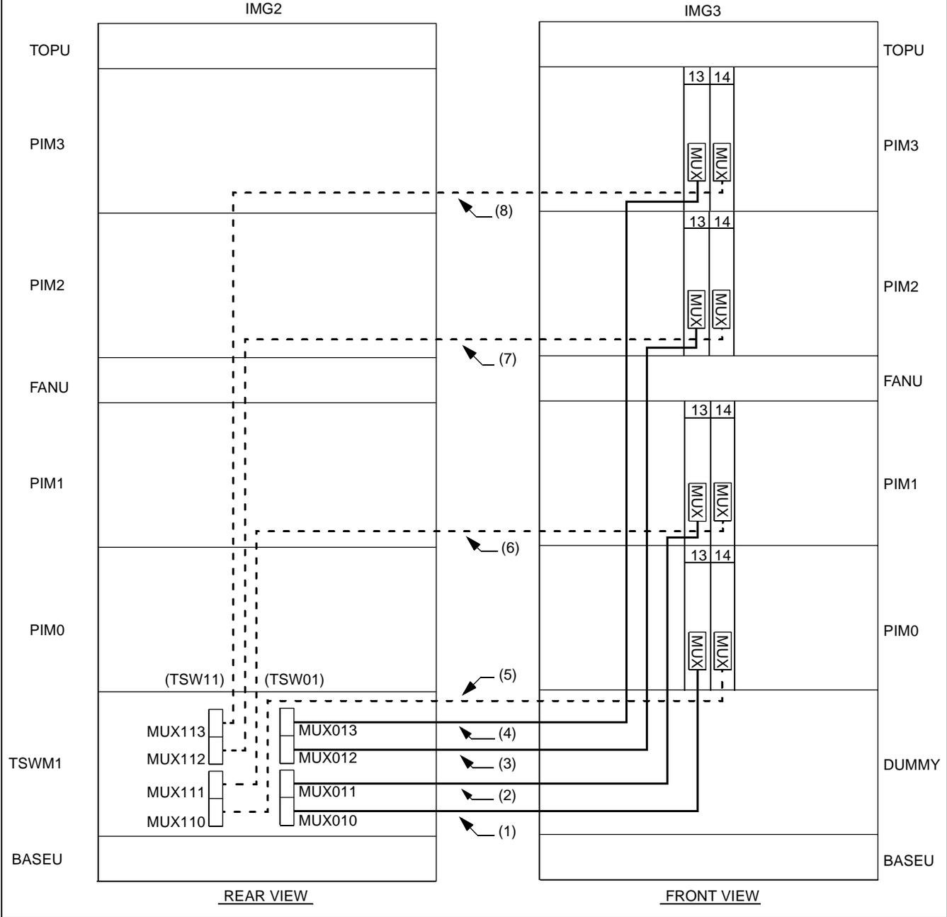
Figure 010-25 Inter-frame Bus Cable Connection for IMG2-IMG3
