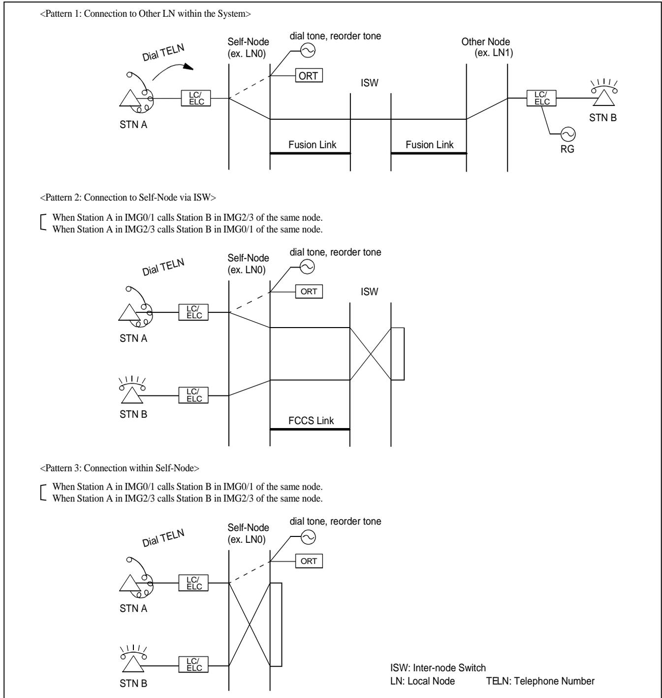
**Figure 024-1 Station-to-Station Connection Test**
