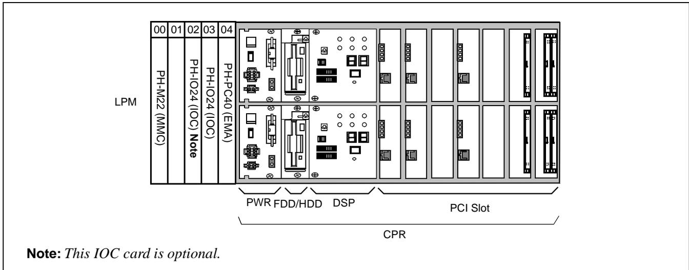
Figure 2-16 Controlling Circuit Cards in LPM (LN)
