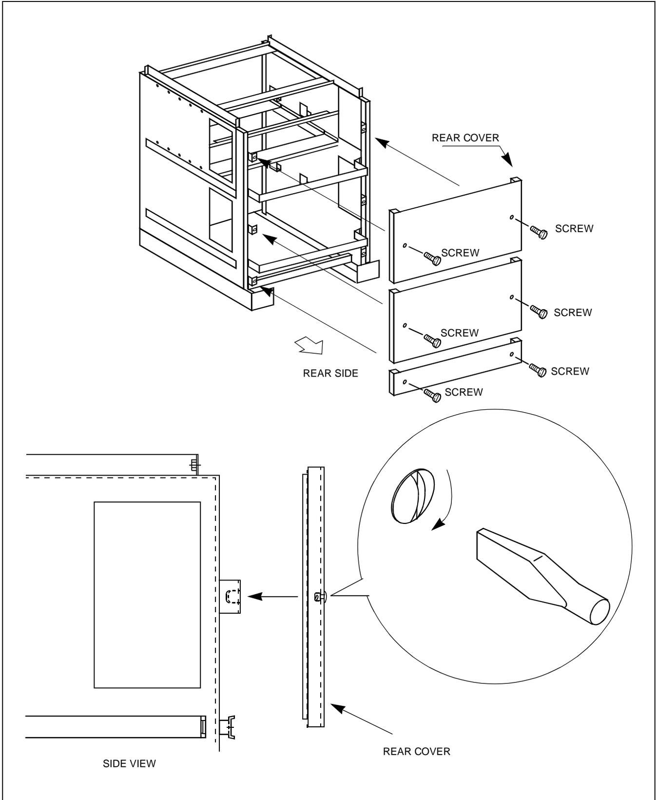
Figure 7-5 Rear Cover Mounting Method (BASEU+LPM+PIM0)
