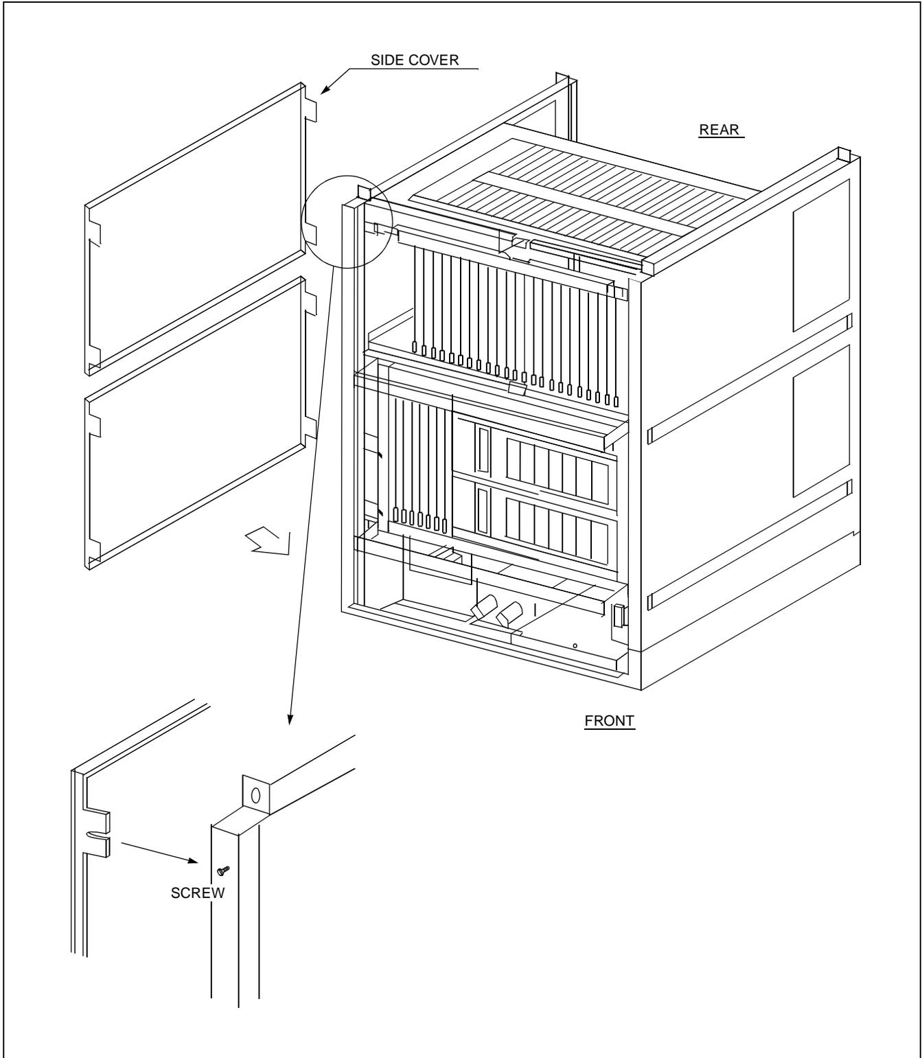
Figure 7-3 Side Cover Mounting Method (BASEU+LPM+PIM0)
