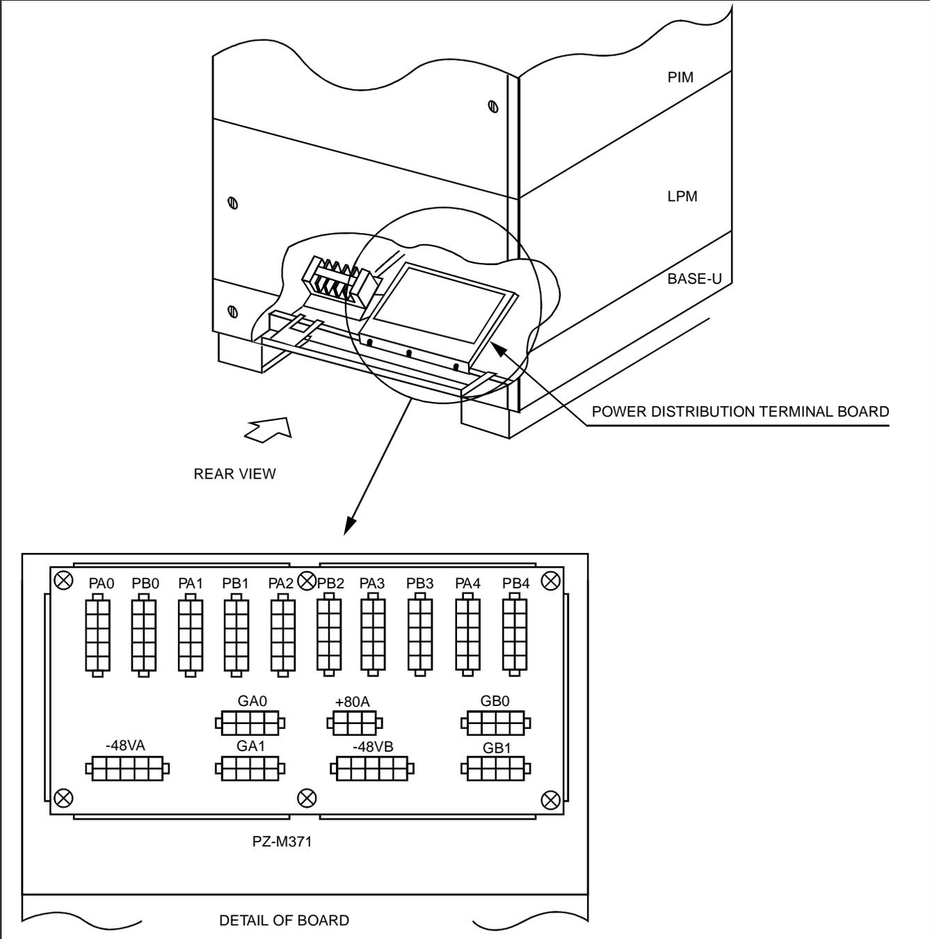
Figure 010-8 Location of Connectors on the Power Distribution Terminal Board (PZ-M371)
