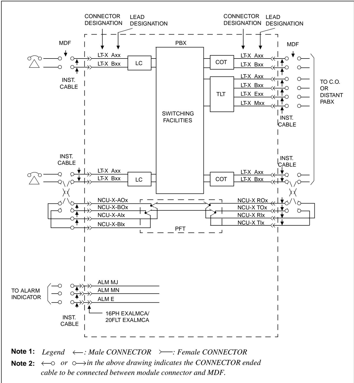
Figure 2-23 Outline of Cables from Module Group to the Outside
