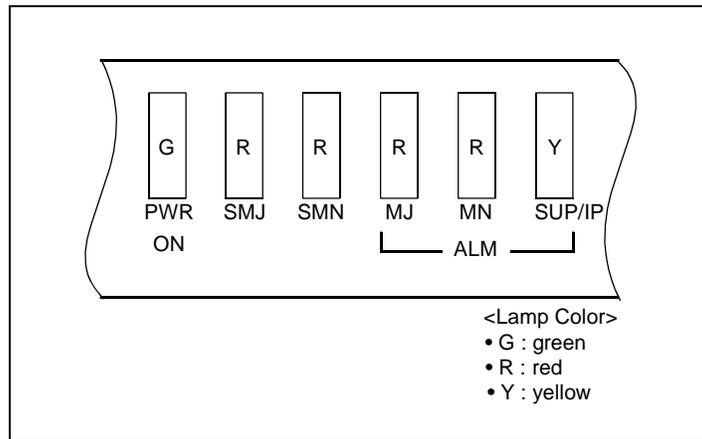
**Figure 022-1 Alarm Lamps on the TOPU**
