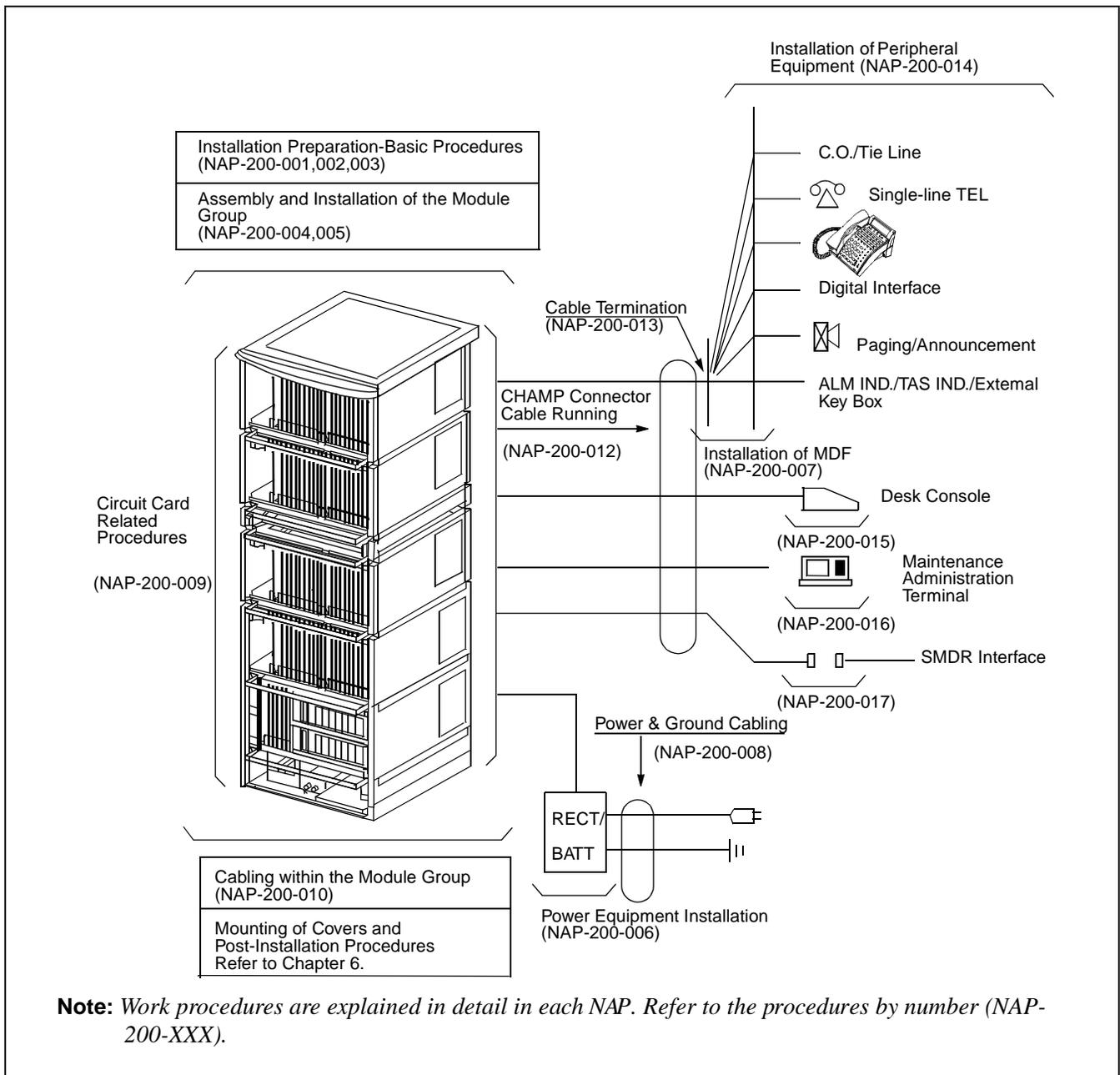
Figure 3-1 Scope of Installation Procedure
