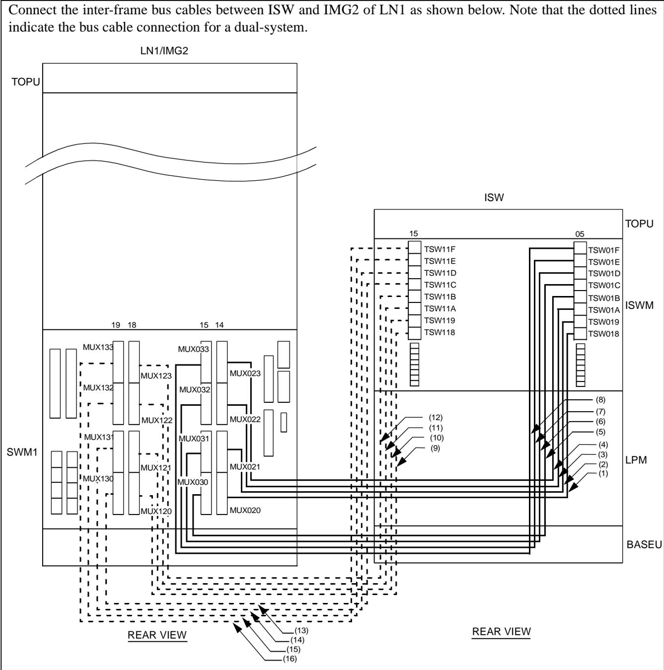
Figure 010-33 Inter-frame Bus Cable Connection for ISW-LN1, IMG2
