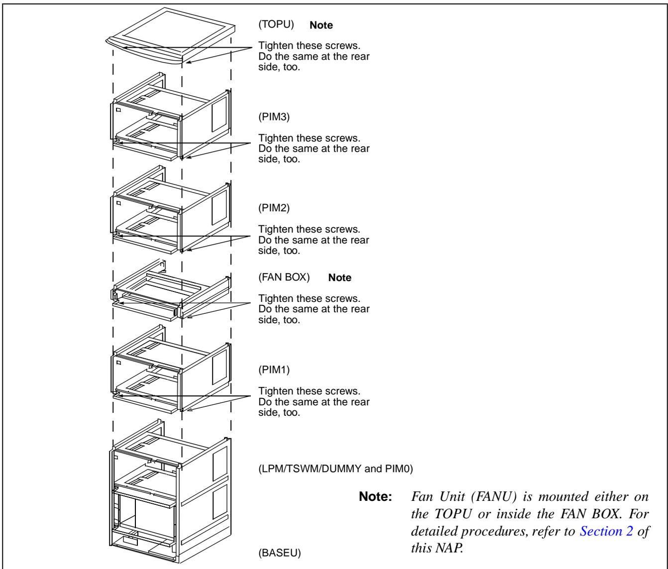
Figure 005-1 Procedure for Mounting Units and Modules
