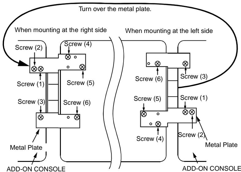
Figure 015-17 Mounting of Add-On Console (Left Side of DESK CONSOLE)
