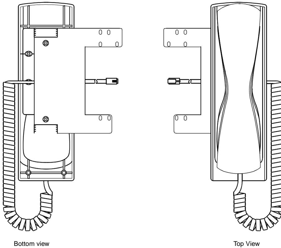
3. Connect the Handset code to HAND H/S0 connector as shown below (H/S1 is not used for the Handset).
