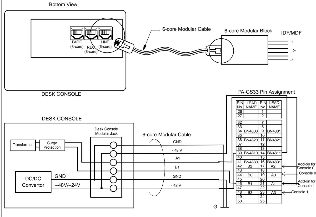
Figure 015-5 Cable Connection Diagram for DESK CONSOLE Modular Block
