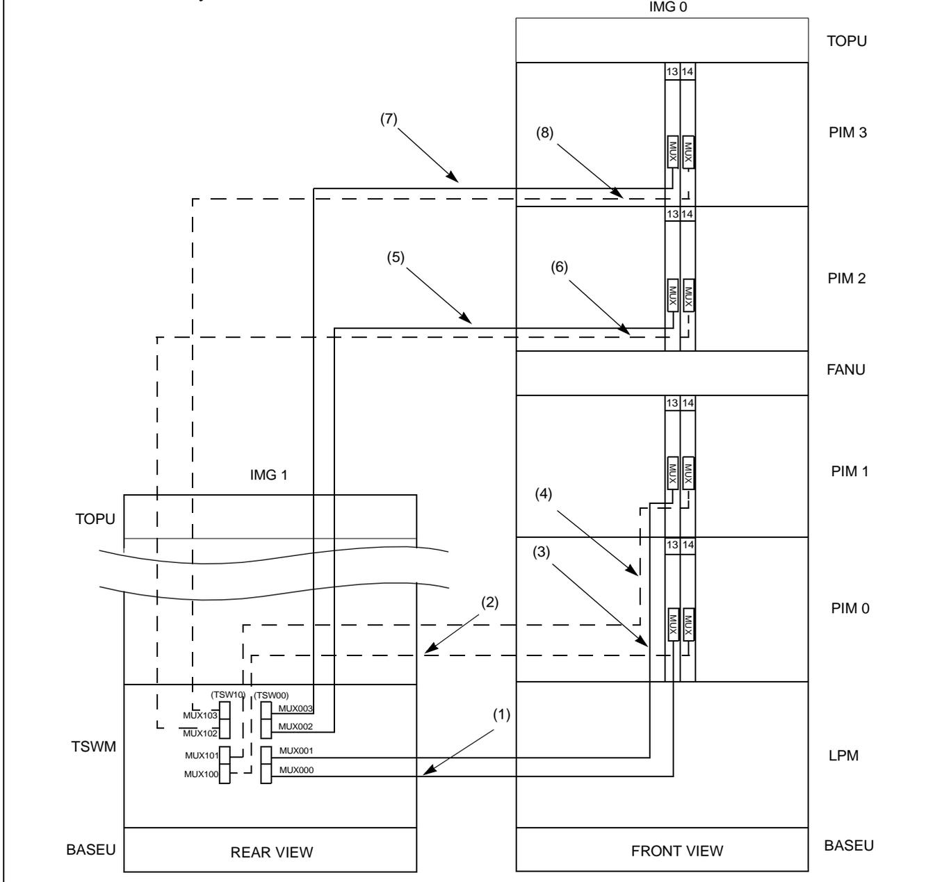
Figure 010-19 Inter-frame Bus Cable Connection for IMG0-IMG1
