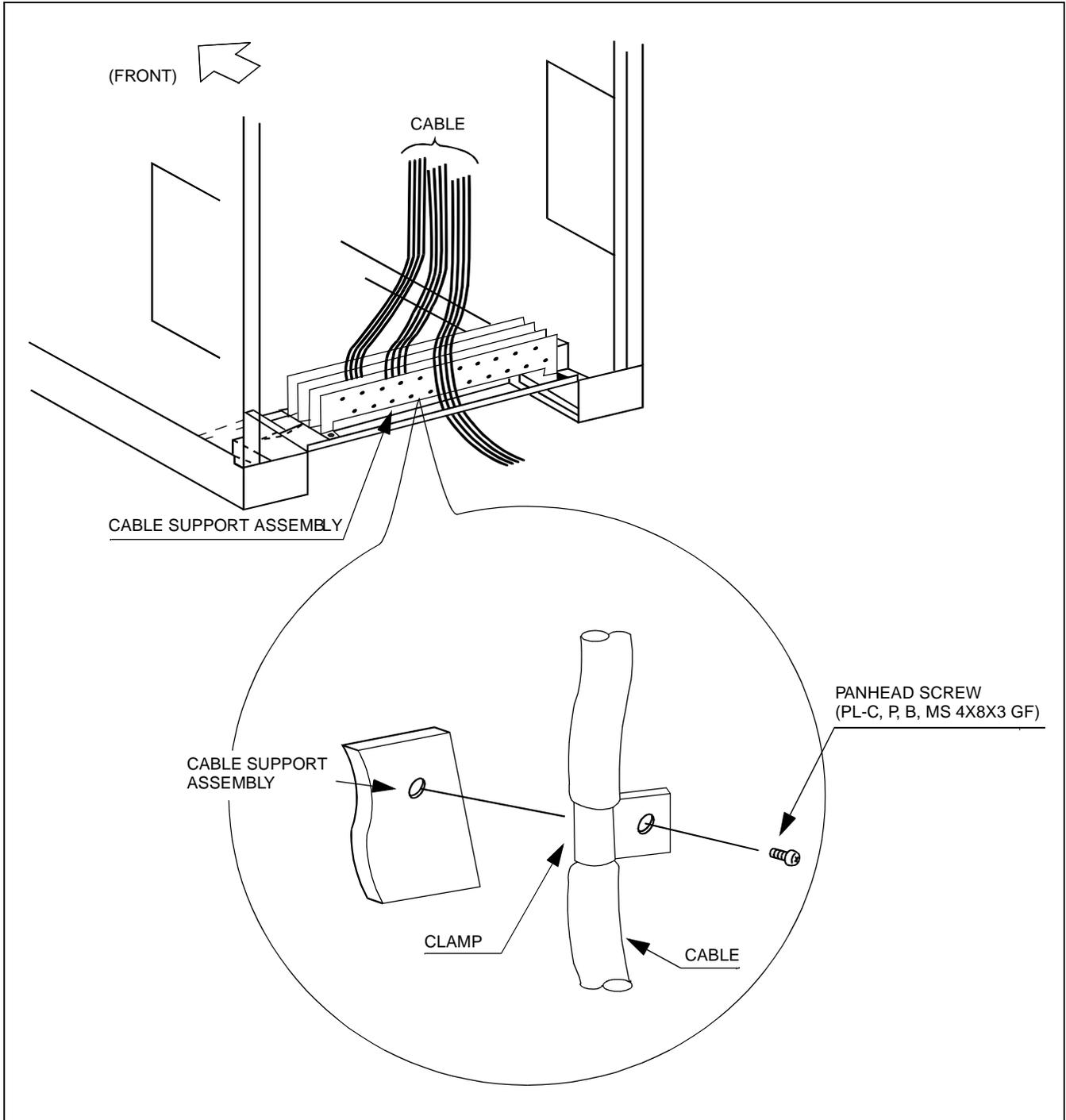
Figure 012-6 Termination of Installation Cables
