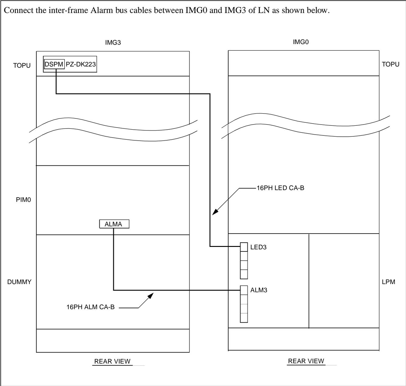
Figure 010-23 Inter-frame Alarm Bus Cable Connection for IMG0-IMG3
