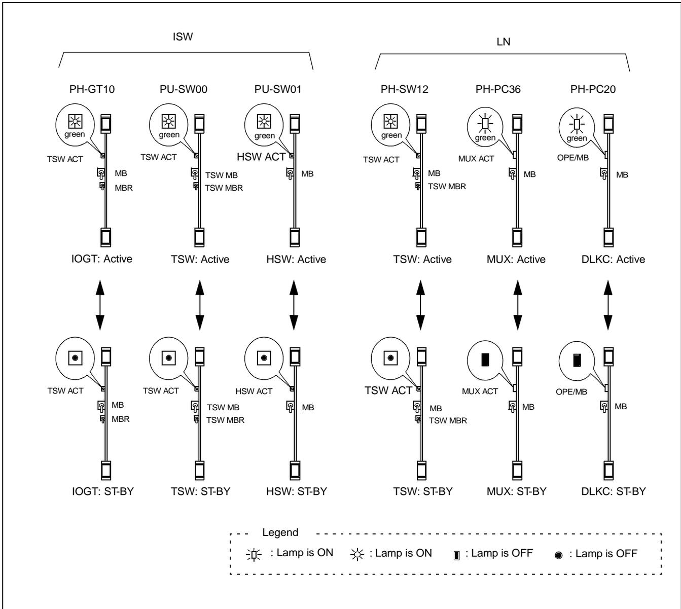
Figure 025-3 LEDs and Switches for Speech Path System Changeover
