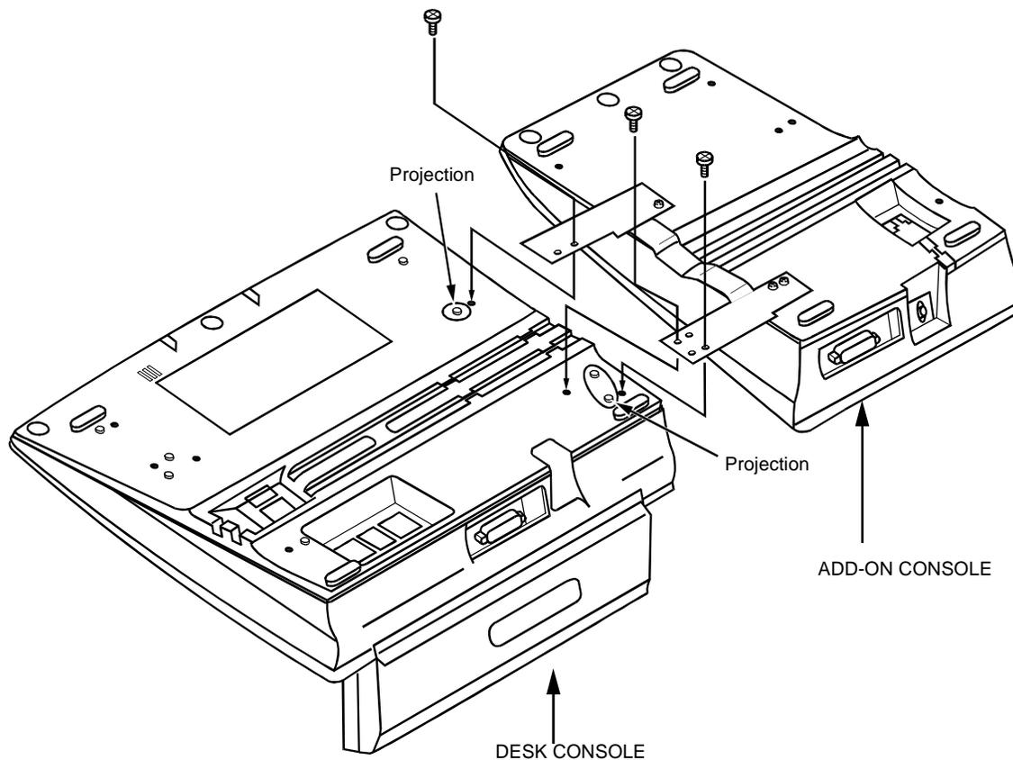
Figure 015-16 Mounting of Add-On Console (Right Side of DESK CONSOLE) (Continued)
