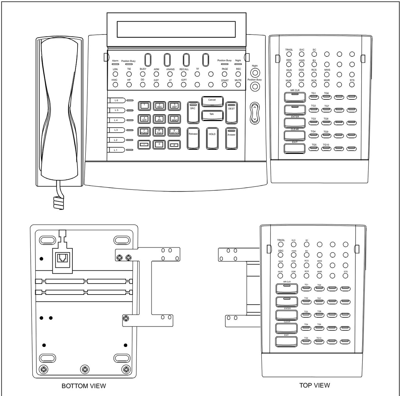
Figure 015-16 Mounting of Add-On Console (Right Side of DESK CONSOLE)
