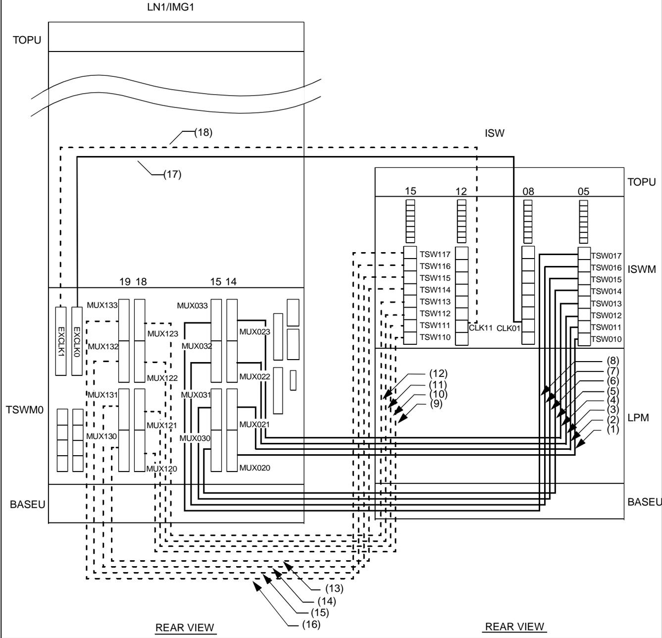
Figure 010-32 Inter-frame Bus Cable Connection for ISW-LN1, IMG1
