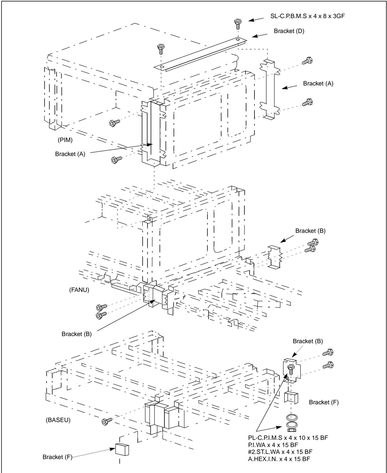
Figure 7-13 How to Attach Inter-frame Brackets (2 of 3)
