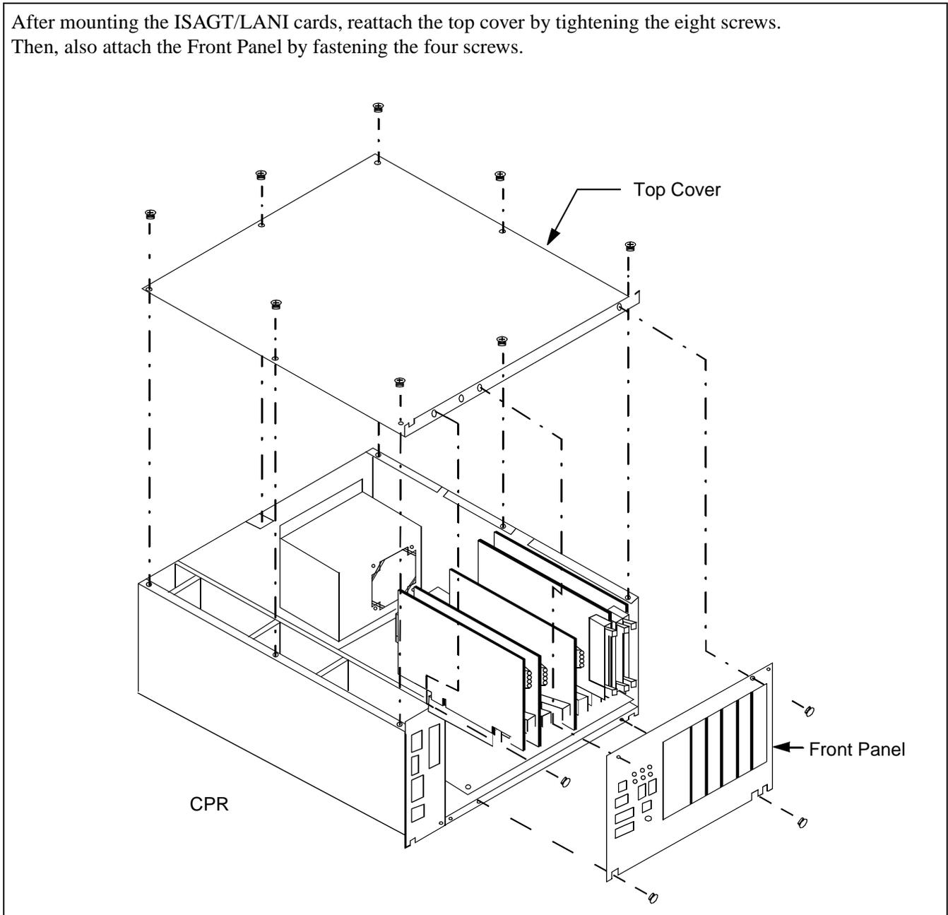
**Figure 009-6 Reattaching CPR Top Cover and Front Panel**
