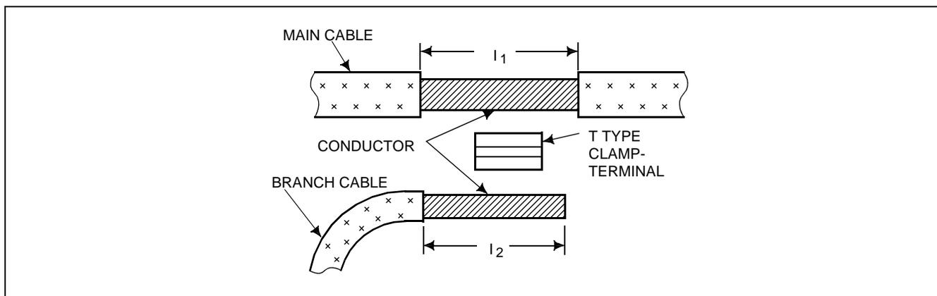
**Figure 008-7 Stripped Length of Main and Branch Cable**
