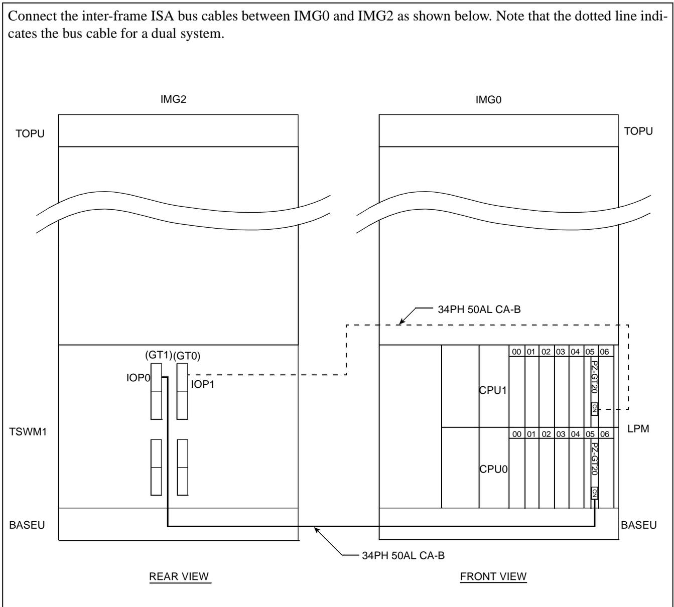
Figure 010-21 Inter-frame ISA Bus Cable Connection for IMG0-IMG2
