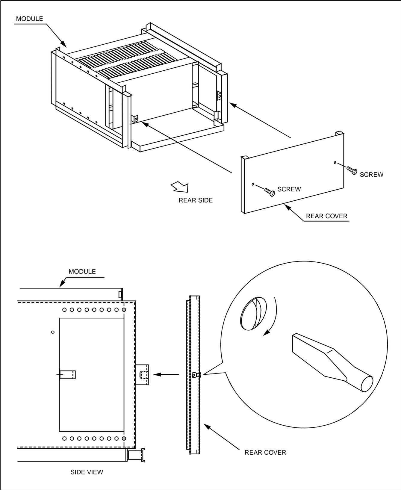
Figure 7-6 Rear Cover Mounting Method (PIM)
