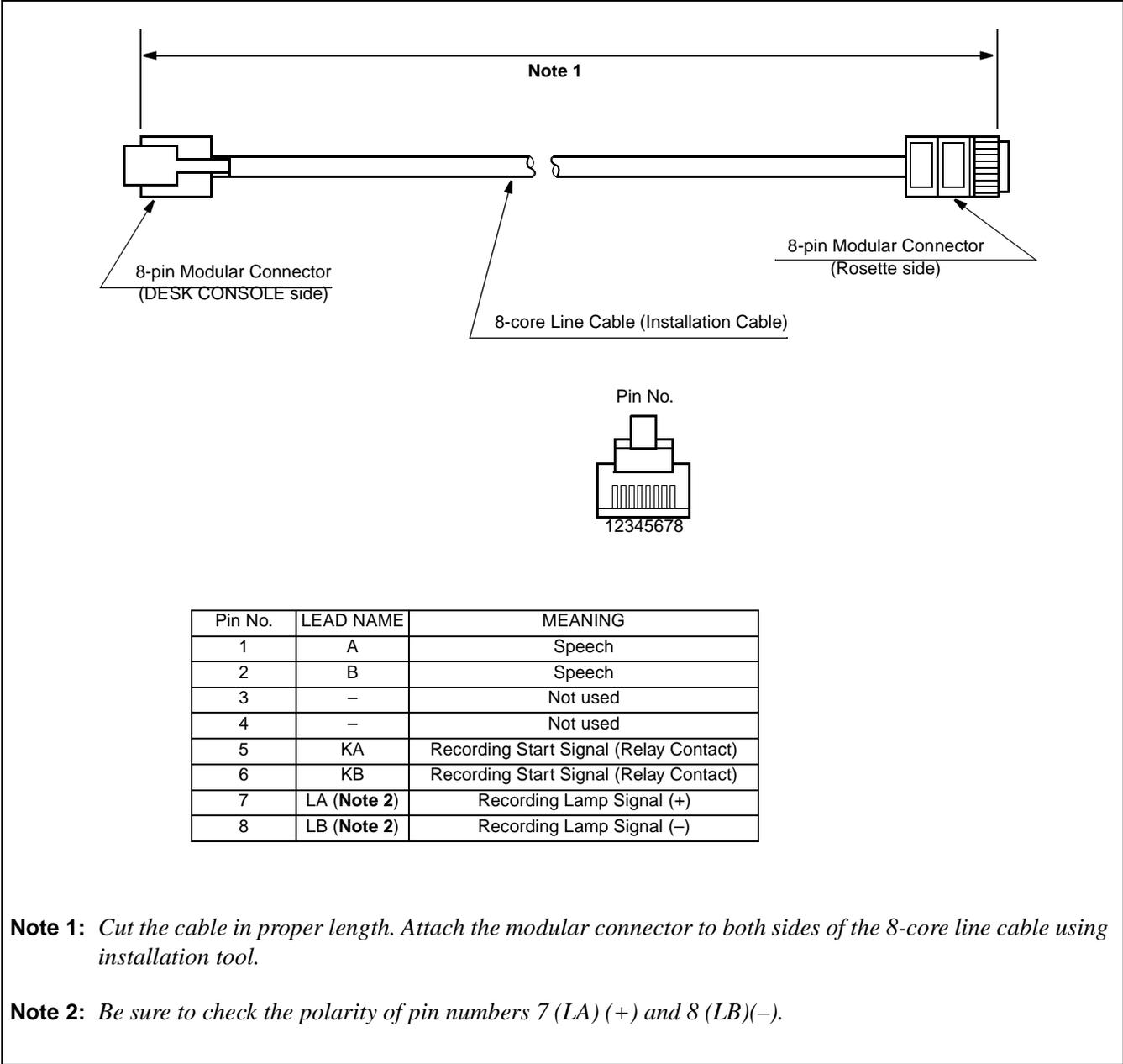
**Figure 015-12 8-core Line Cable**
