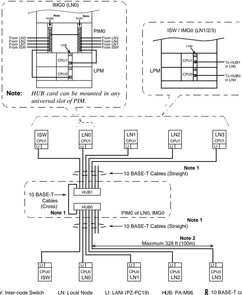
Figure 2-6 Details on Ether Cable Connections (Establishment of Fusion Link) (1/2)
