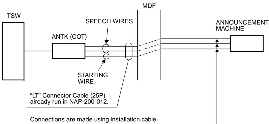
A total of three wires are required per line: two wires for speech and one starting wire.
