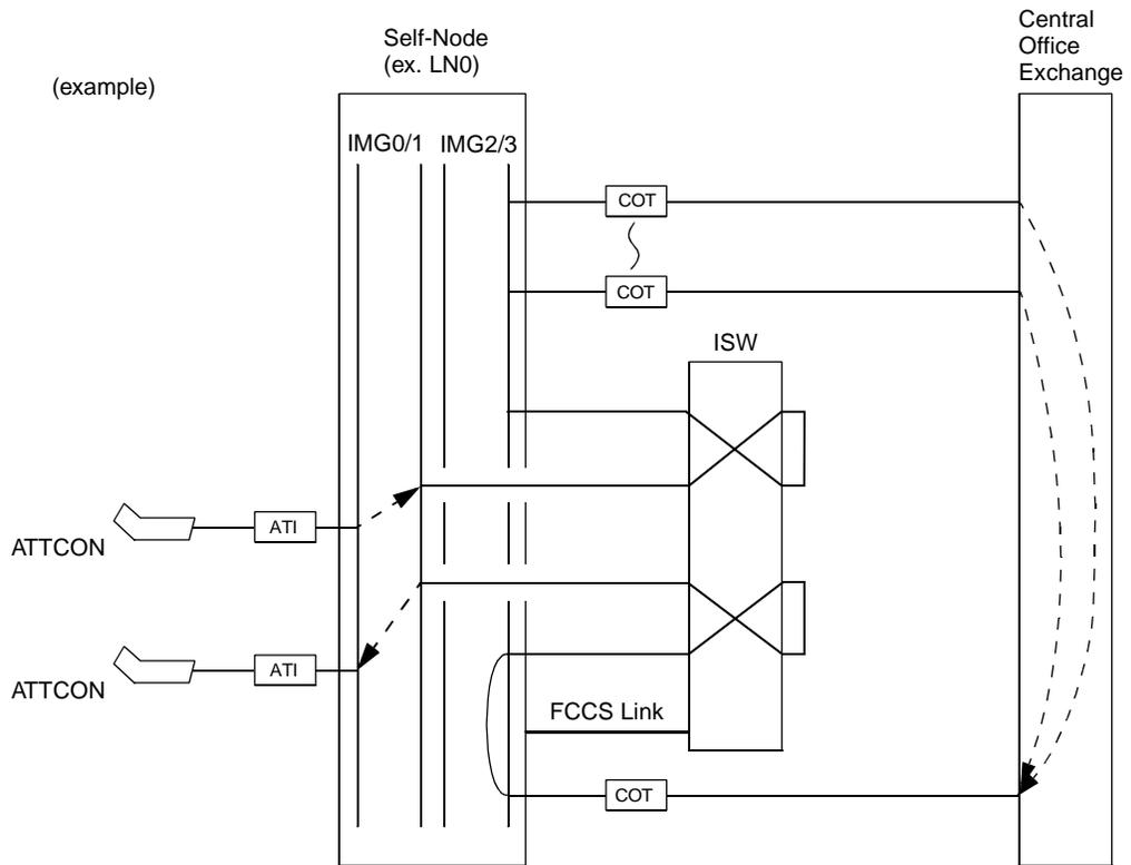
Figure 043-1 Overall Test for C.O. Line Incoming Call (1/2)
