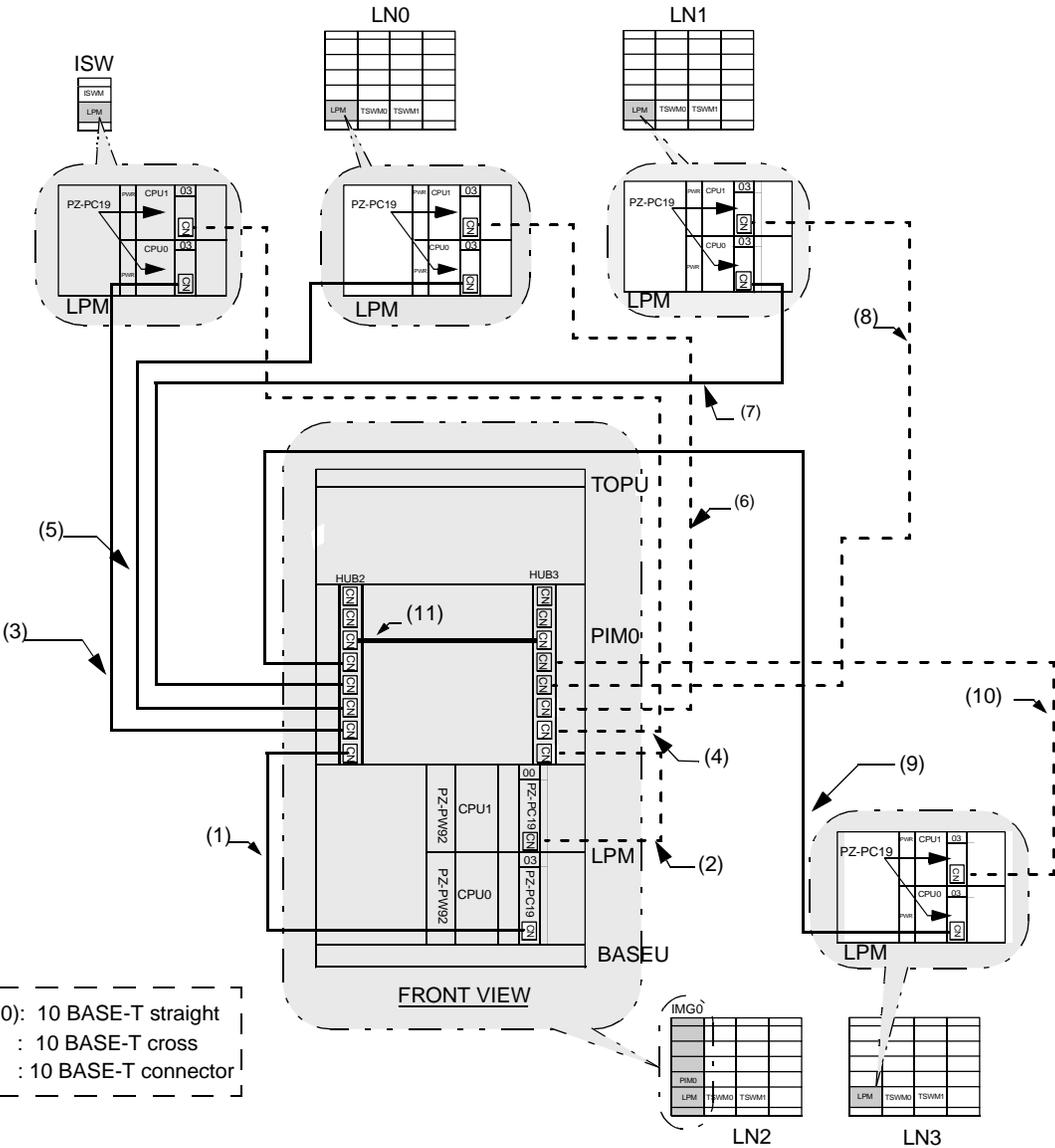
**Note:** PA-M96 (HUB) card can be mounted in any universal slot (Slot No. 04-12, 15-23) of a PIM.
