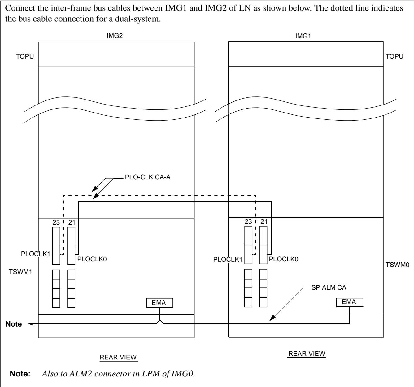
**Figure 010-24 Inter-frame Bus Cable Connection for IMG1-IMG2**
