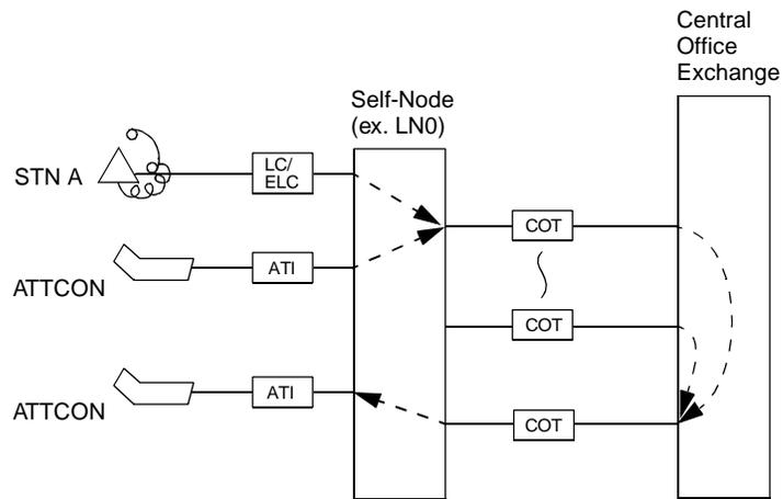
Figure 042-1 Overall Test for C.O. Line Outgoing Call (2/2)
