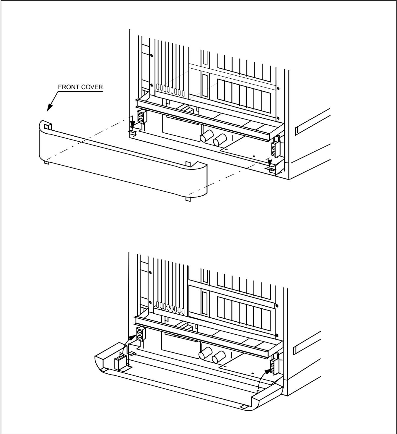
Figure 7-9 Front Cover Mounting Method (BASEU+LPM+PIM0)
