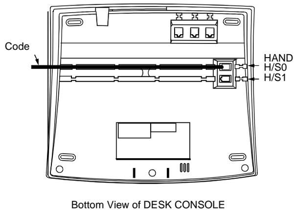
Figure 015-8 Mounting of Handset (Right side of DESK CONSOLE) (Continued)
