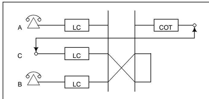
**Figure 031-1 COT Test Configuration**
