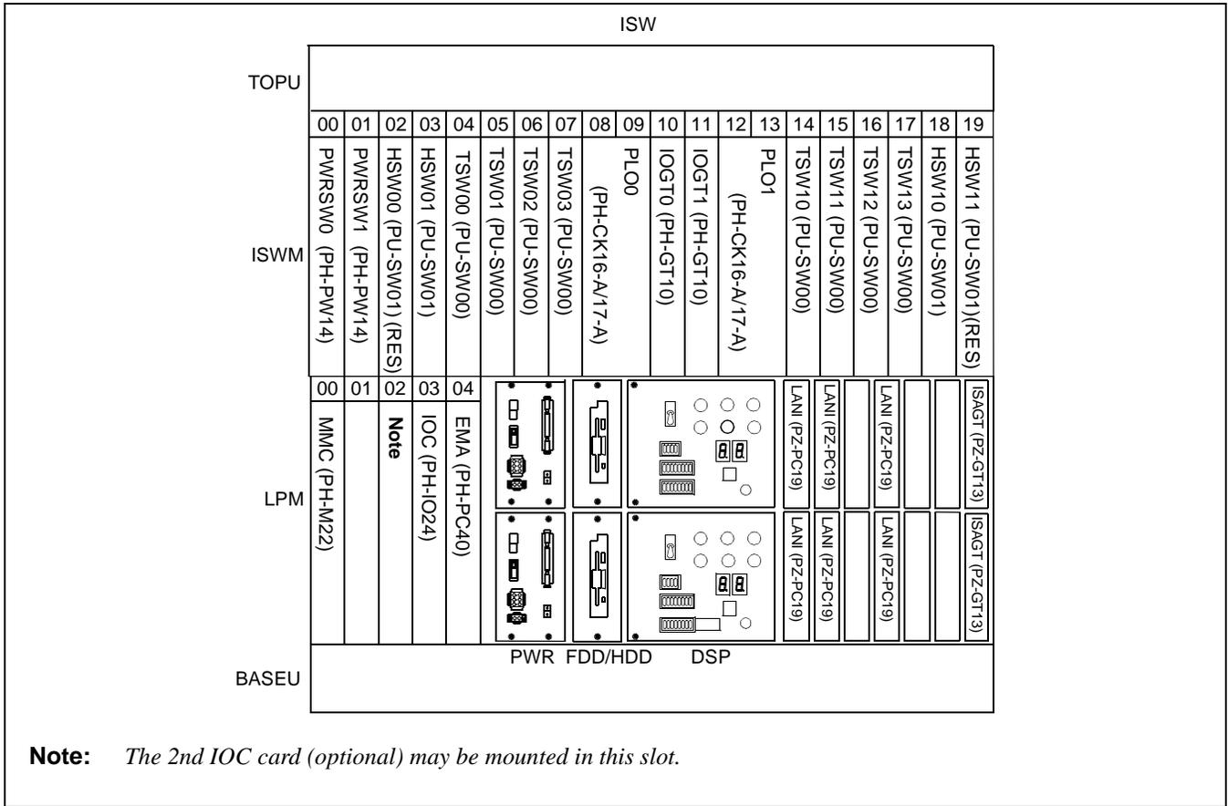
Figure 2-9 Face Layout of ISW
