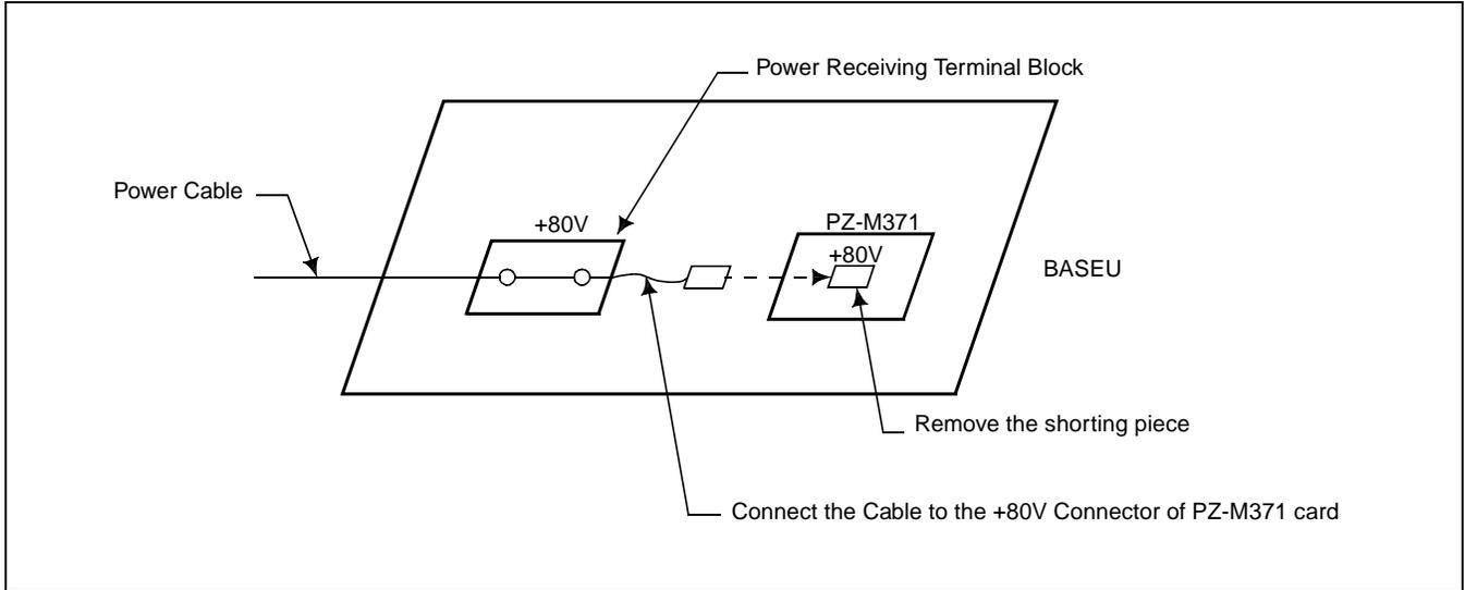
**Figure 008-4 Removal of Shorting Piece and Cable Connection**
