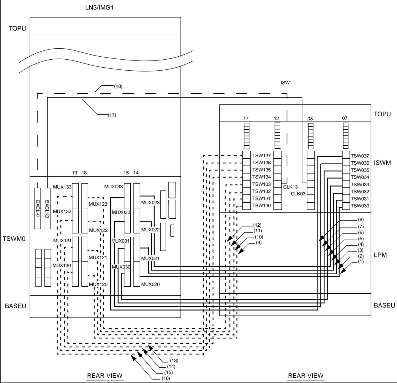
Figure 010-36 Inter-frame Bus Cable Connection for ISW-LN3, IMG1
