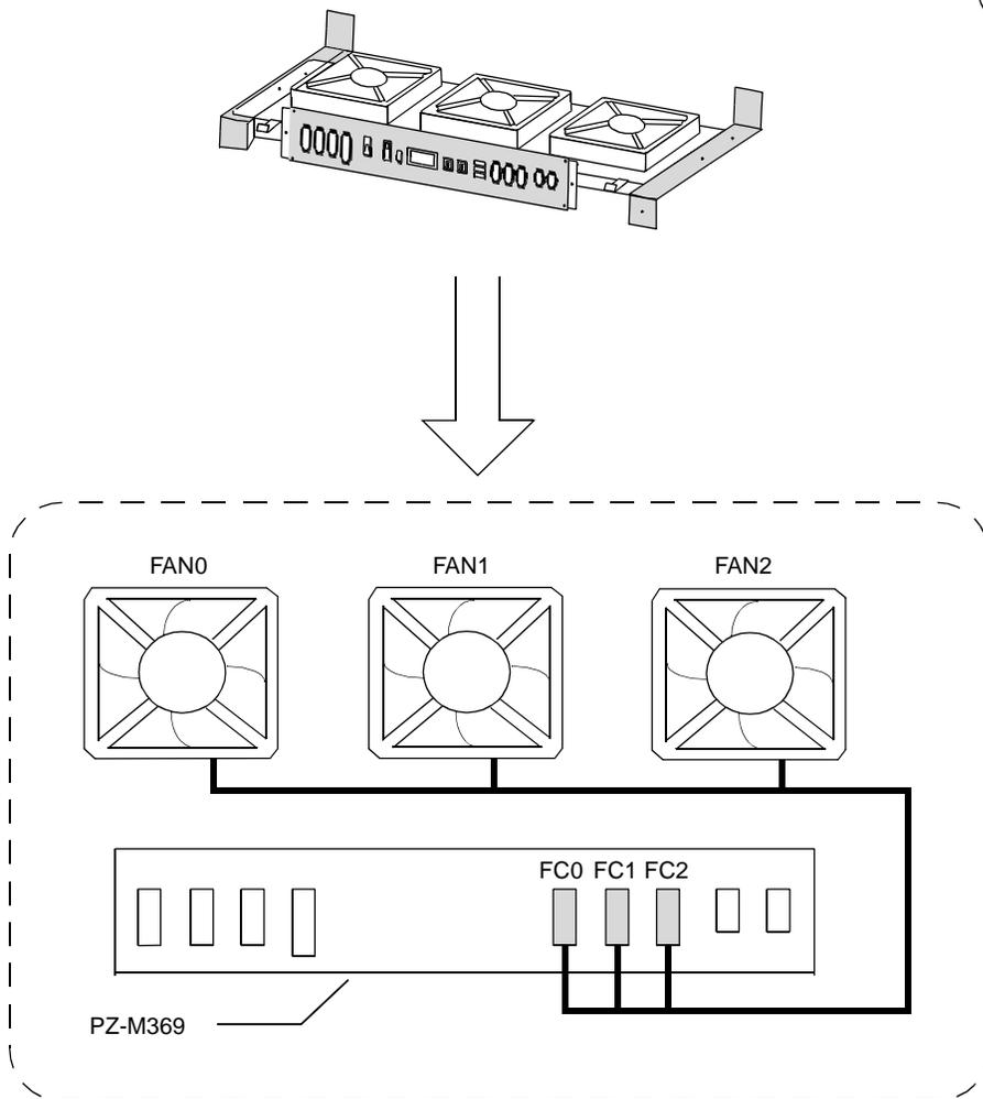
**Figure 005-9 FAN Cable Connections for FC0/FC1/FC2 Connectors**
