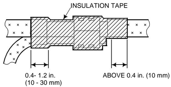
**Note:** *Taping should be done in two rounds with the tape overlapping half the tape width.*
