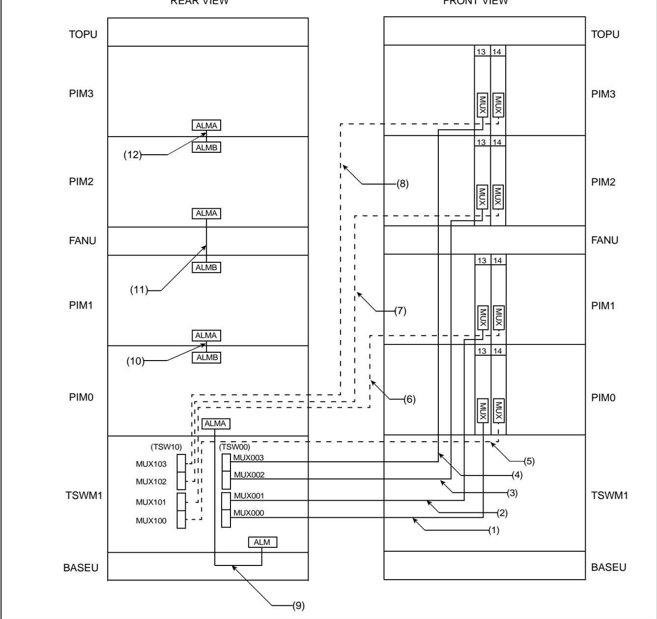
Figure 010-16 Internal Bus Cable Connection for IMG2
