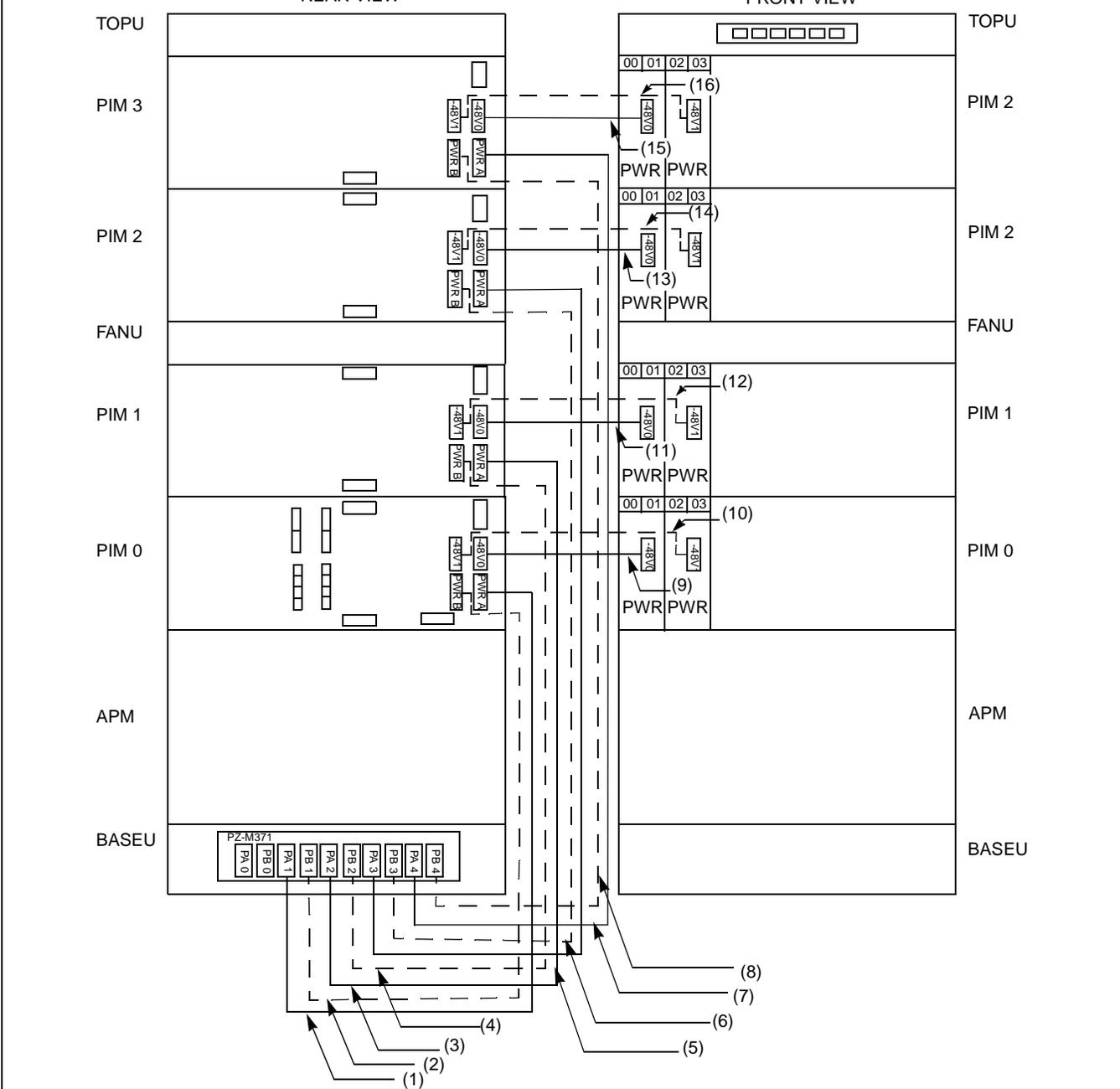
Figure 010-12 Internal Power Cable Connection for IMG3
