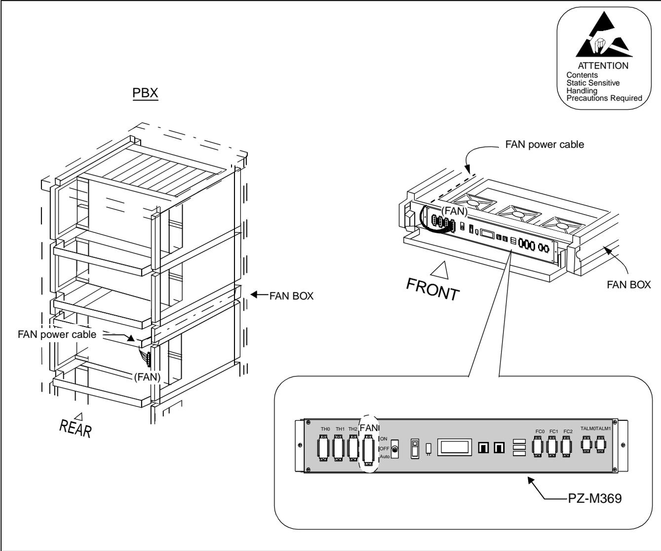
Figure 005-11 Connection of "FAN" Connector Cable (FAN BOX-PIM)
