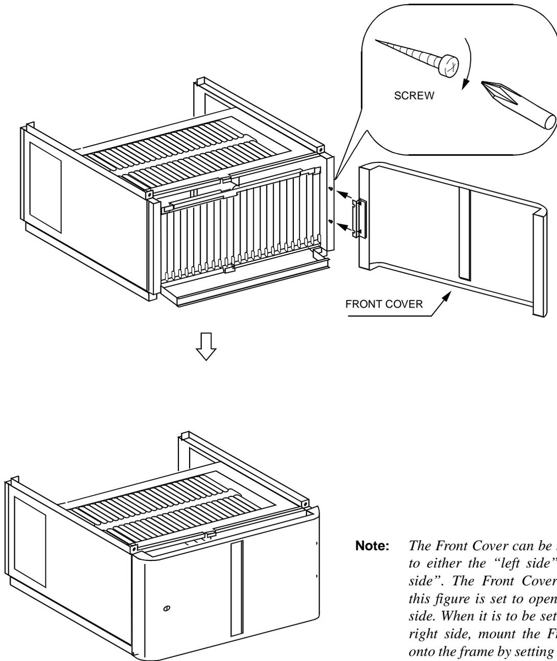
Figure 7-10 Front Cover Mounting Method (PIM)
