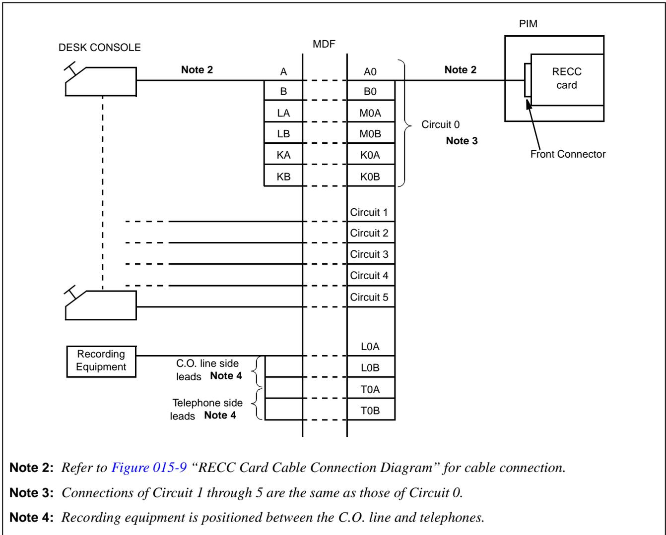
**Figure 015-11 Six DESK CONSOLES and One Recording Equipment**
