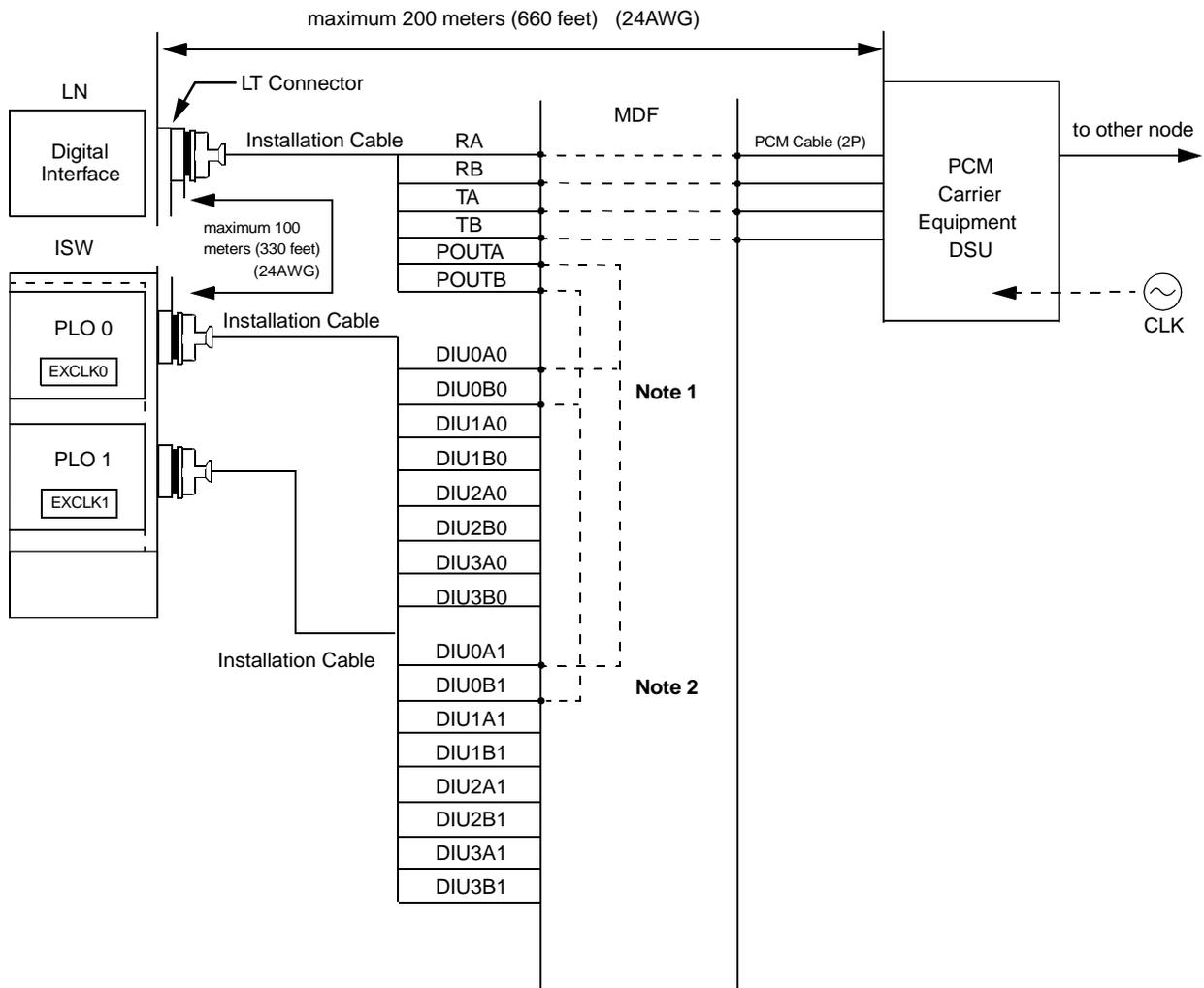
Figure 014-15 Cable Connection Diagram (ISW) for Distributing Clock from Digital Interface
