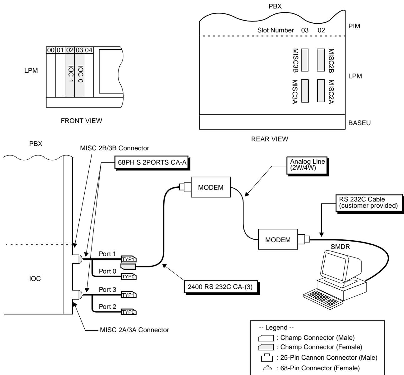
Figure 017-3 Connection of SMDR by Using MODEM
