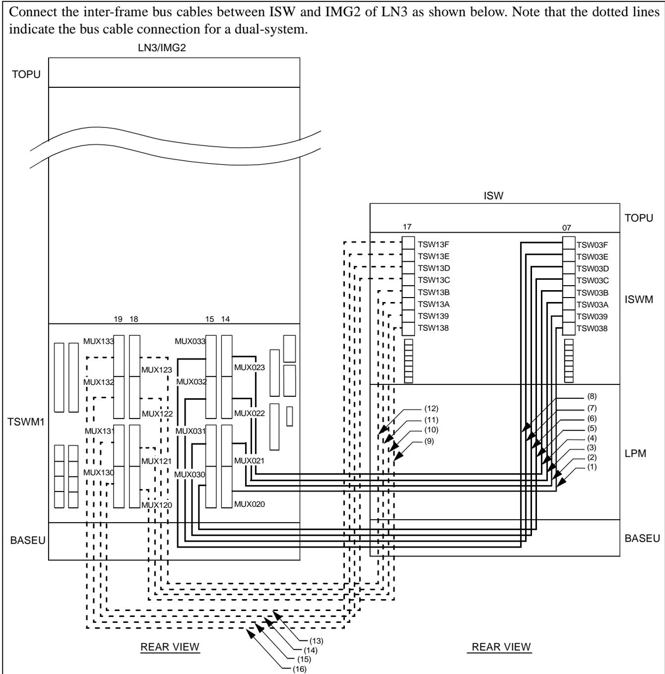
Figure 010-37 Inter-frame Bus Cable Connection for ISW-LN3, IMG2
