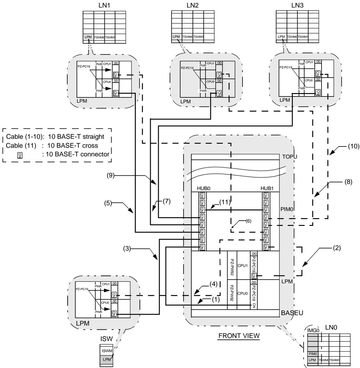
**Note:** HUB (PA-M96) card can be mounted in any universal slot (slot 04 - 12, 15 - 23) of a PIM.
