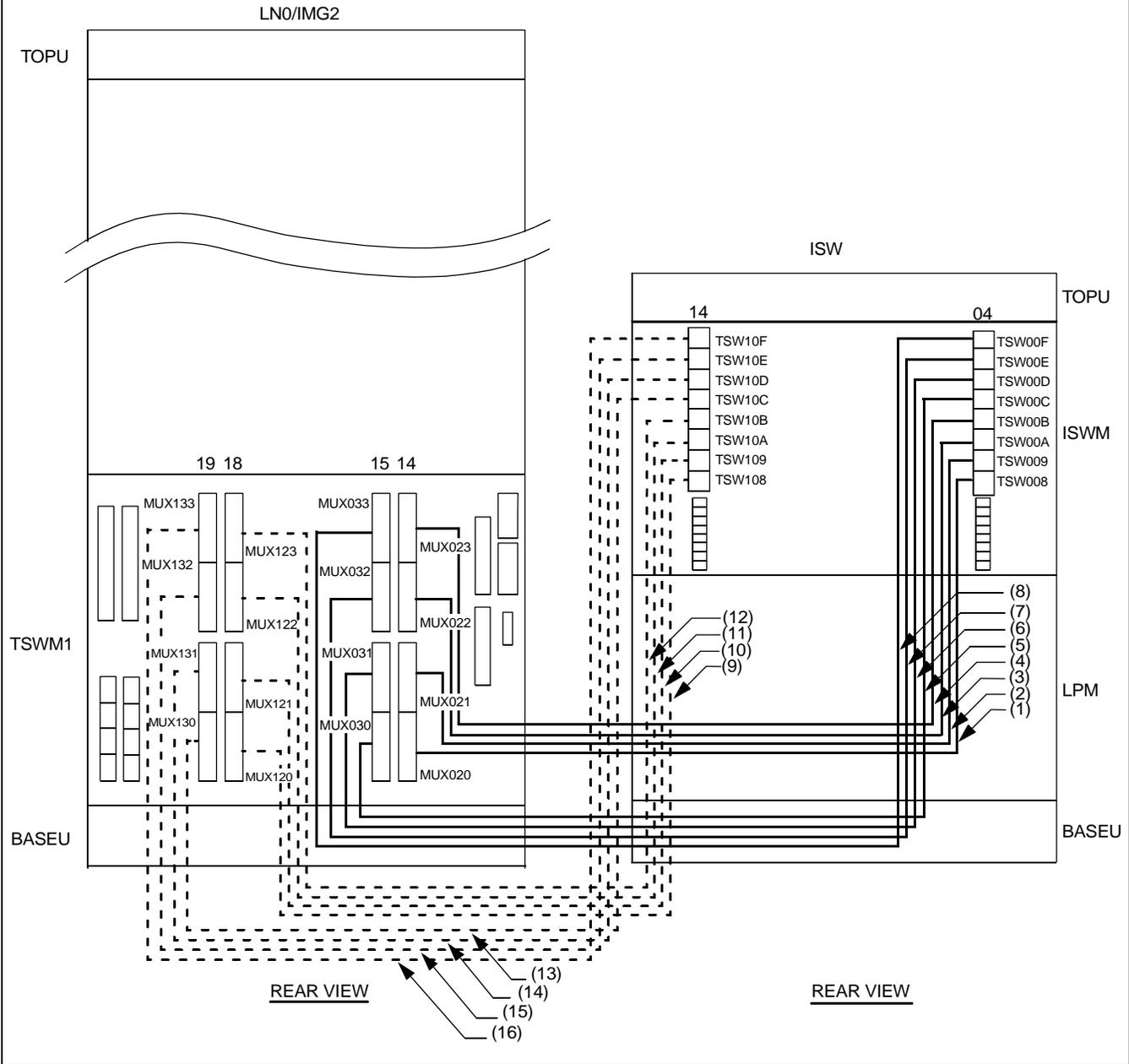
Figure 010-31 Inter-frame Bus Cable Connection for ISW-LN0, IMG2
