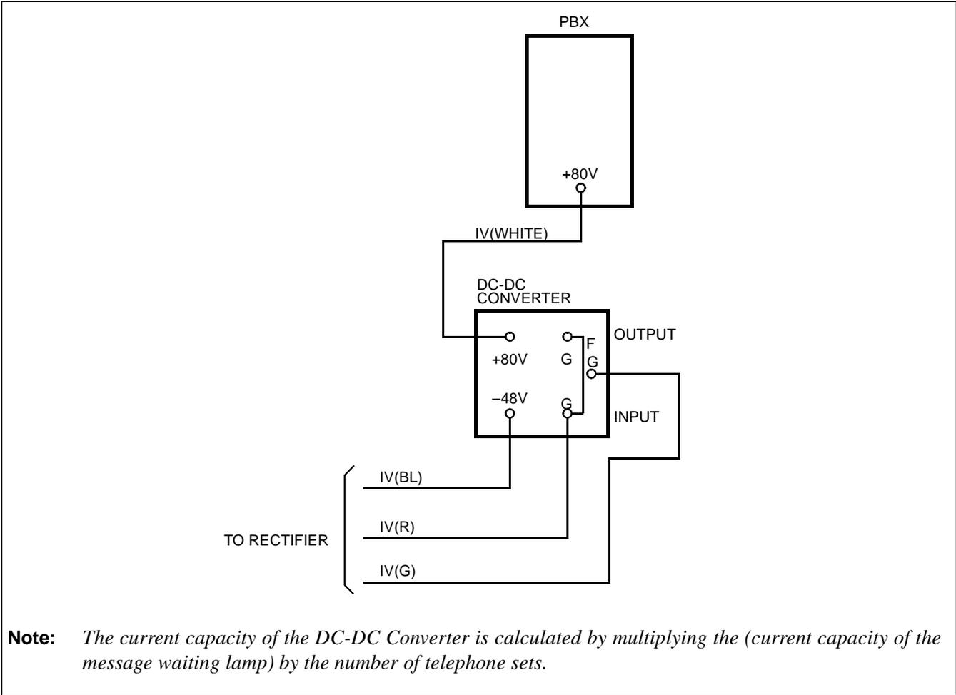
**Note:** *The current capacity of the DC-DC Converter is calculated by multiplying the (current capacity of the message waiting lamp) by the number of telephone sets.*
