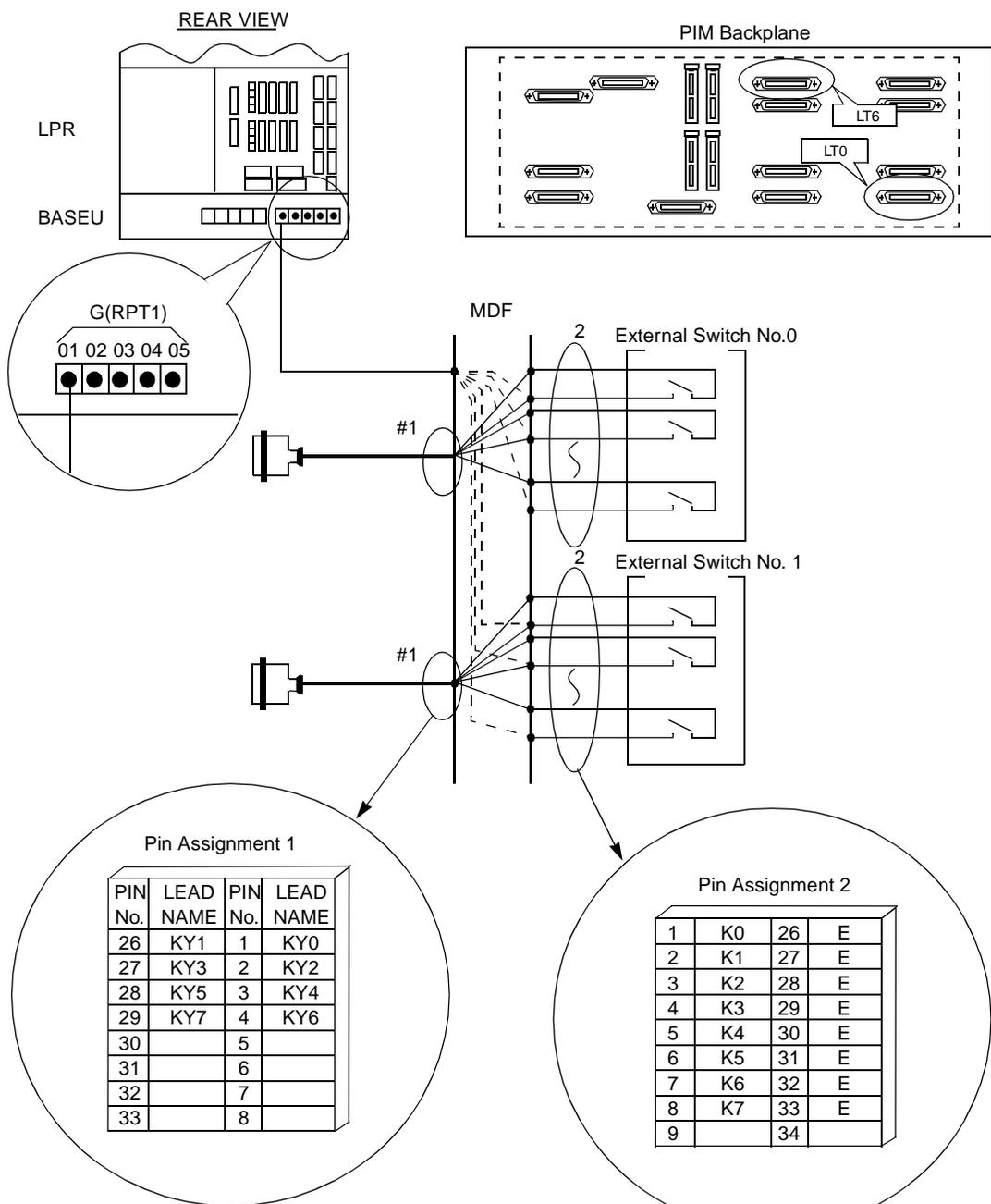
Figure 014-9 Connection of External Switches
