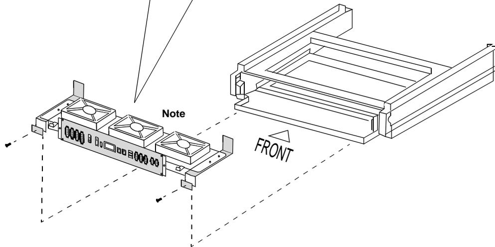
**Note:** Before inserting the FANU into the FAN BOX, connect the FAN cables for “FC0”, “FC1” and “FC2” connectors on the PZ-M369. Refer to [Figure 005-9](#) on the next page.
