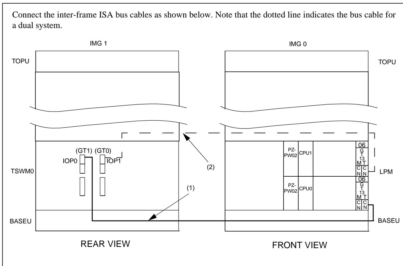
Figure 010-18 Inter-frame ISA Bus Cable Connection for IMG0-IMG1
