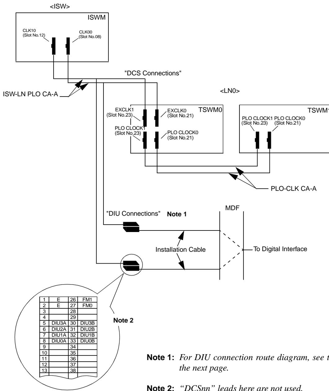
Figure 014-17 LT Connector Lead Accommodation of PLO (ISW-LN0)
