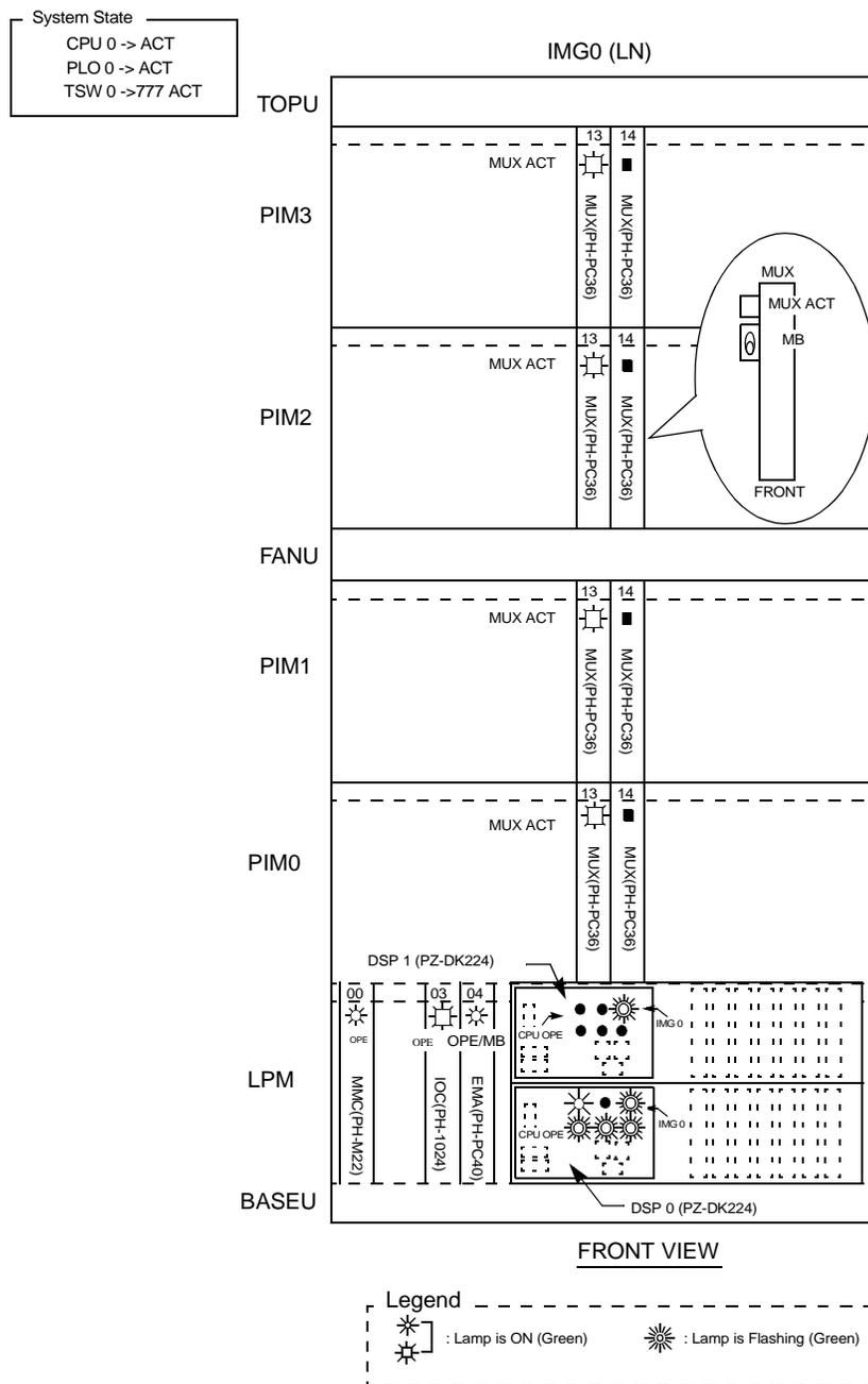
Figure 021-2 LED Indications of IMG0 in Normal Operation (example)
