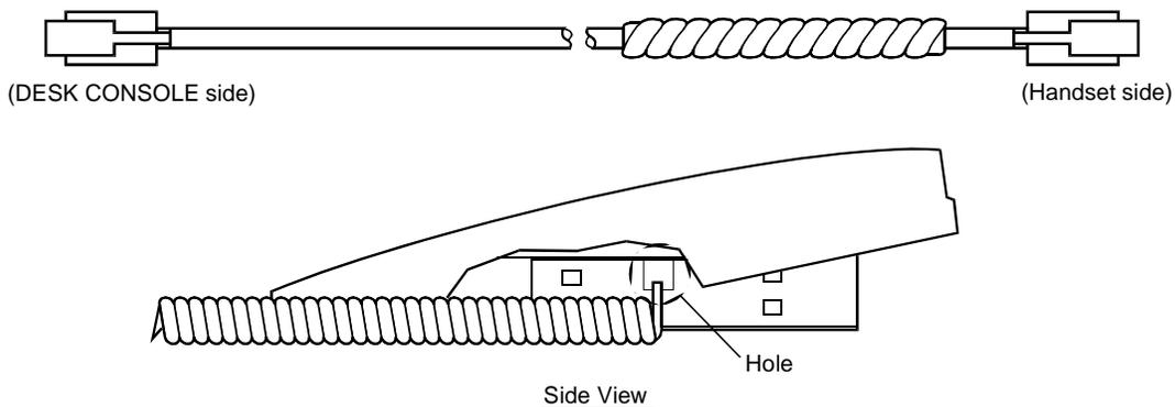
Figure 015-8 Mounting of Handset (Right side of DESK CONSOLE)
