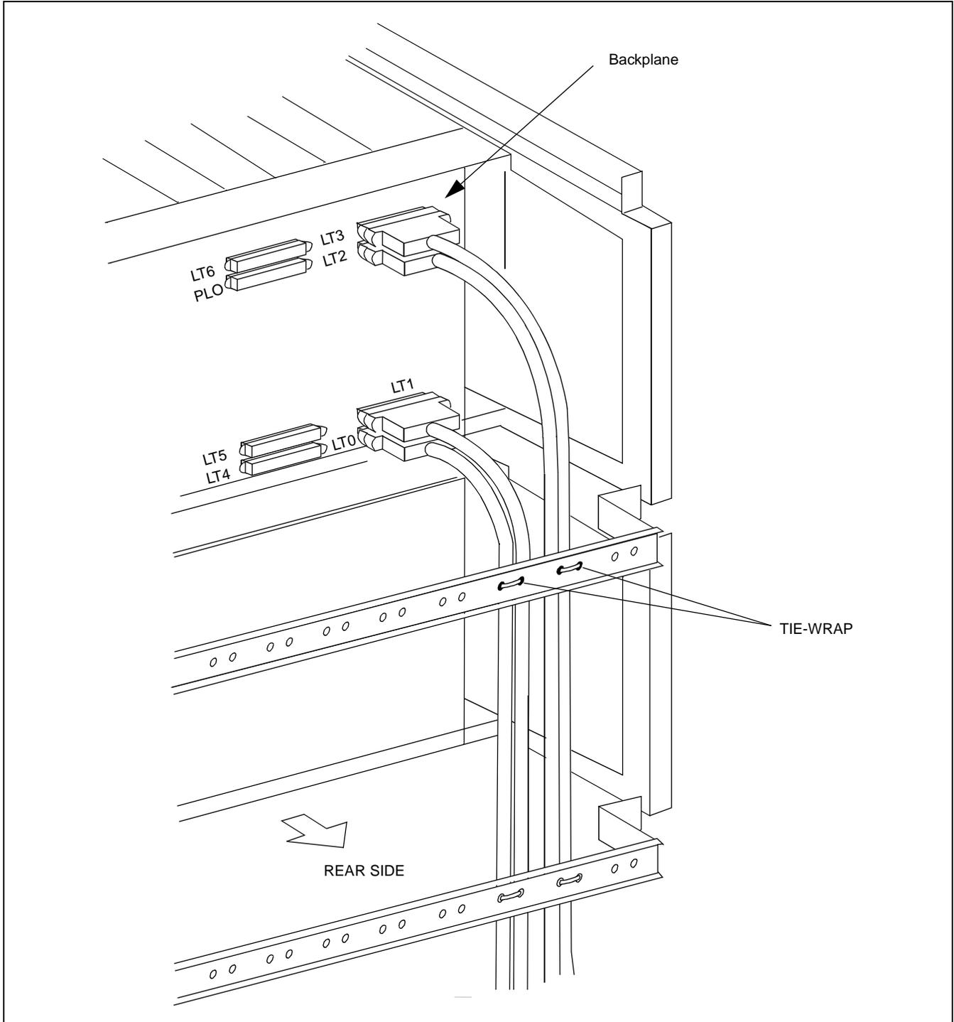
Figure 012-3 Example of Cable Tying Using Tie-Wrap
