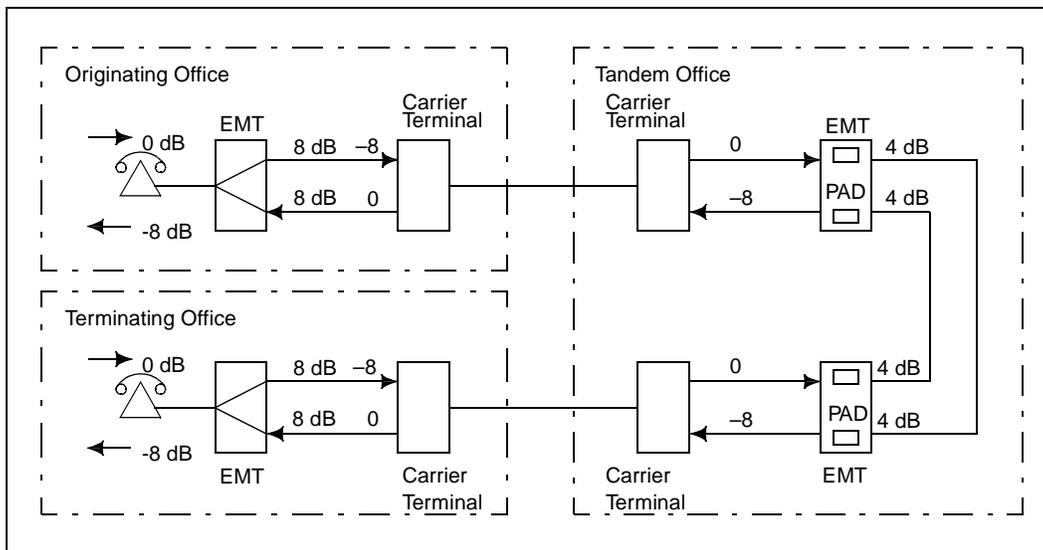
**Figure 049-1 Example of PAD Setting (Analog)**
