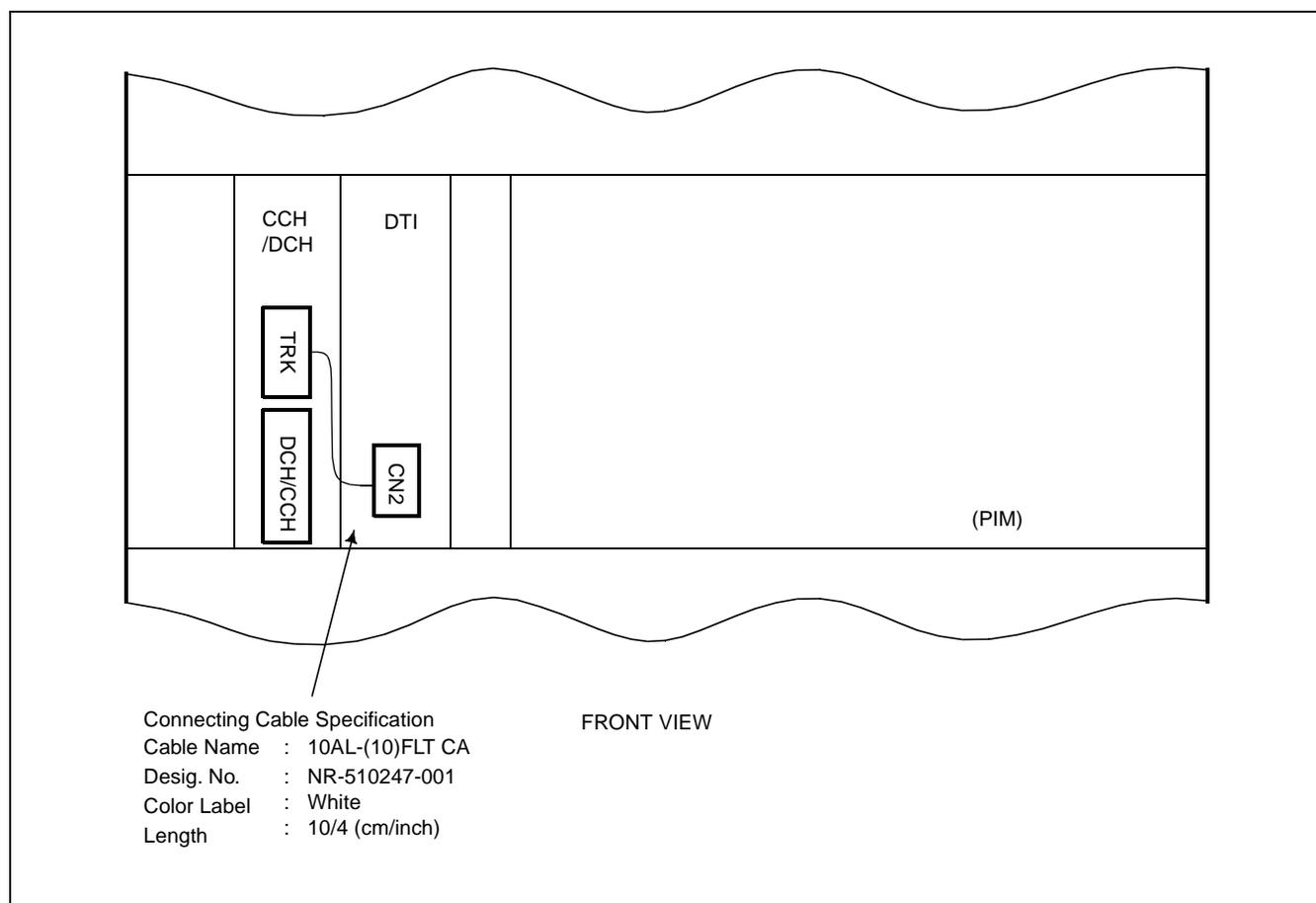
**Figure 011-1 Front Cable Connections between Circuit Cards for CCIS/ISDN**
