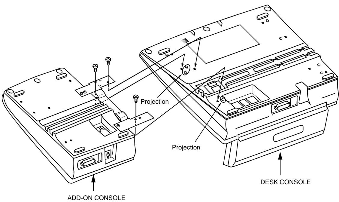
Figure 015-17 Mounting of Add-On Console (Left Side of DESK CONSOLE) (Continued)
