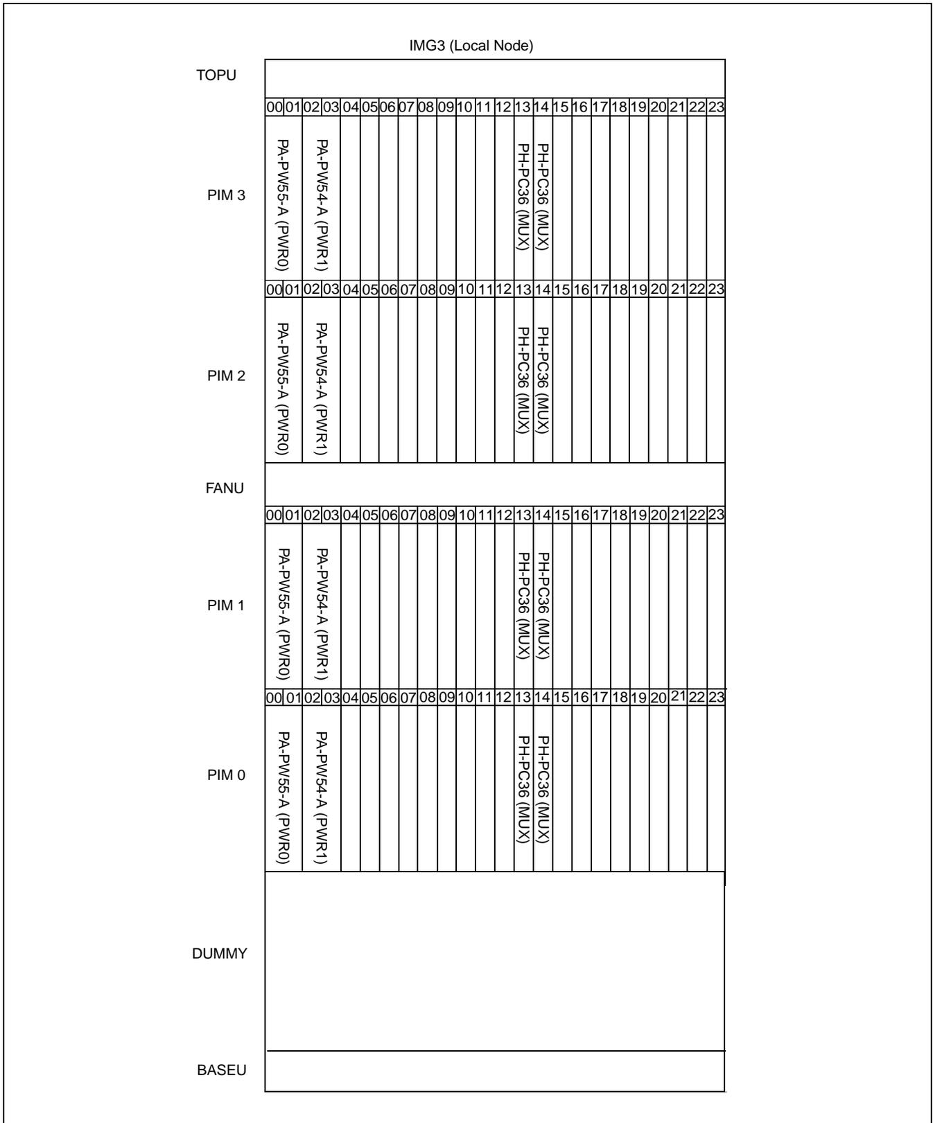
Figure 2-13 Face Layout of IMG3 (Local Node)
