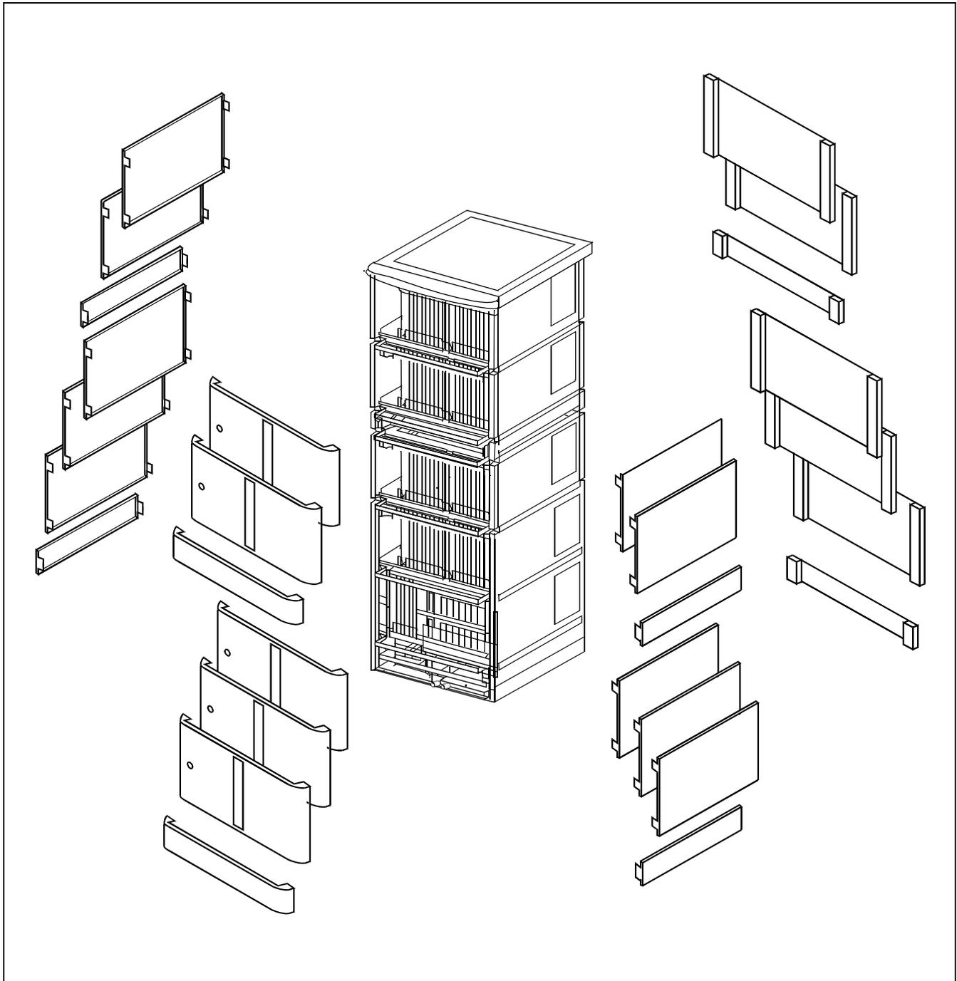
Figure 7-2 Mounting of the Covers
