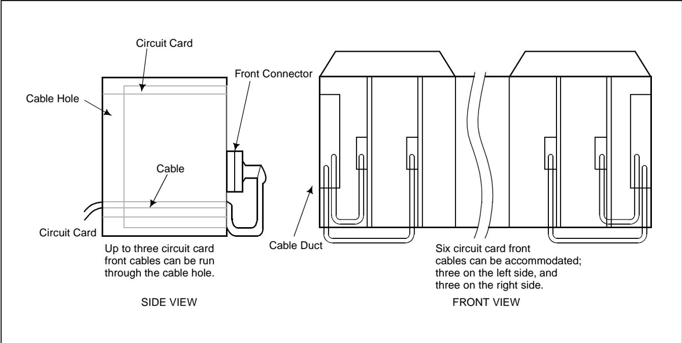
**Figure 012-2 Cable Routing of Circuit Card Front Cable**
