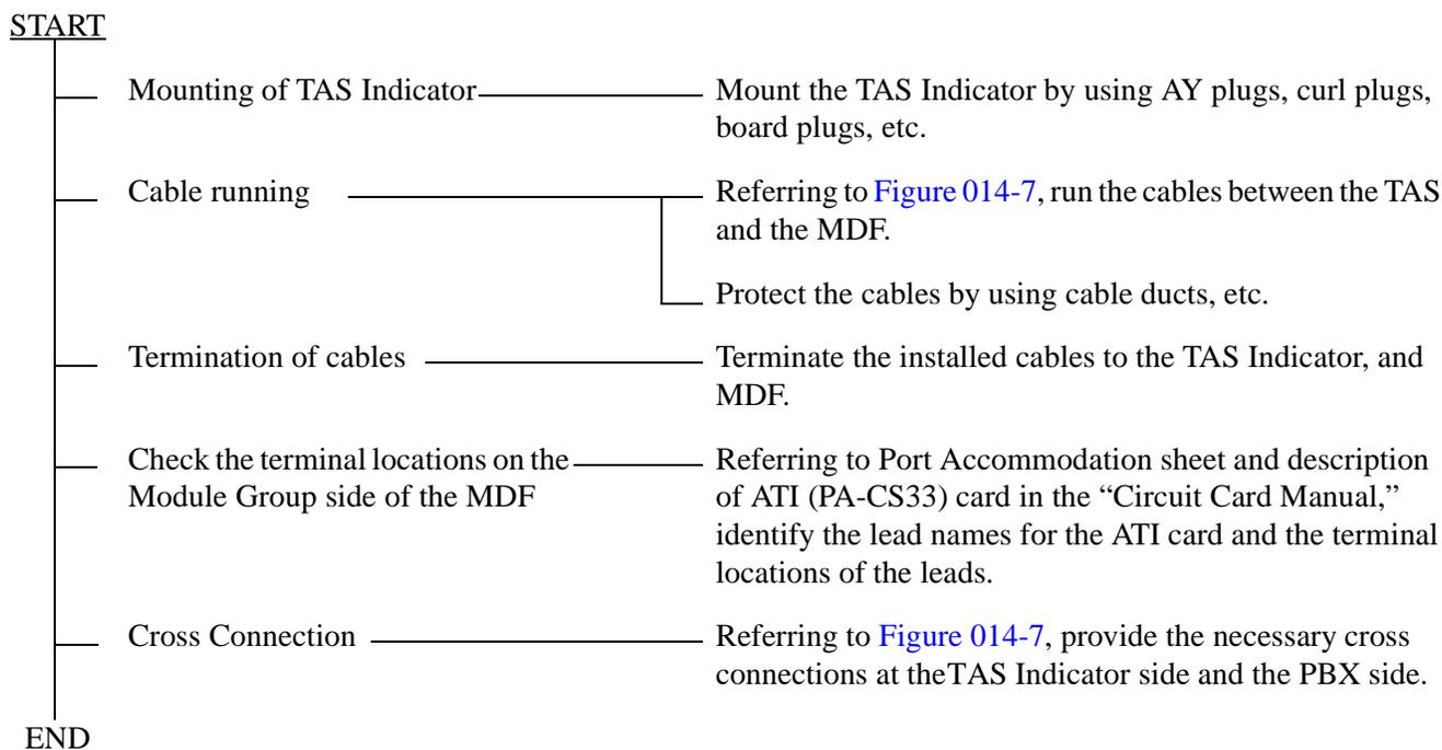
The PA-CS33 card is used as the interface card to connect TAS. The card may be mounted in slot No. 12 or in slot No. 23. The leads appear on LT5 and LT11 respectively.
