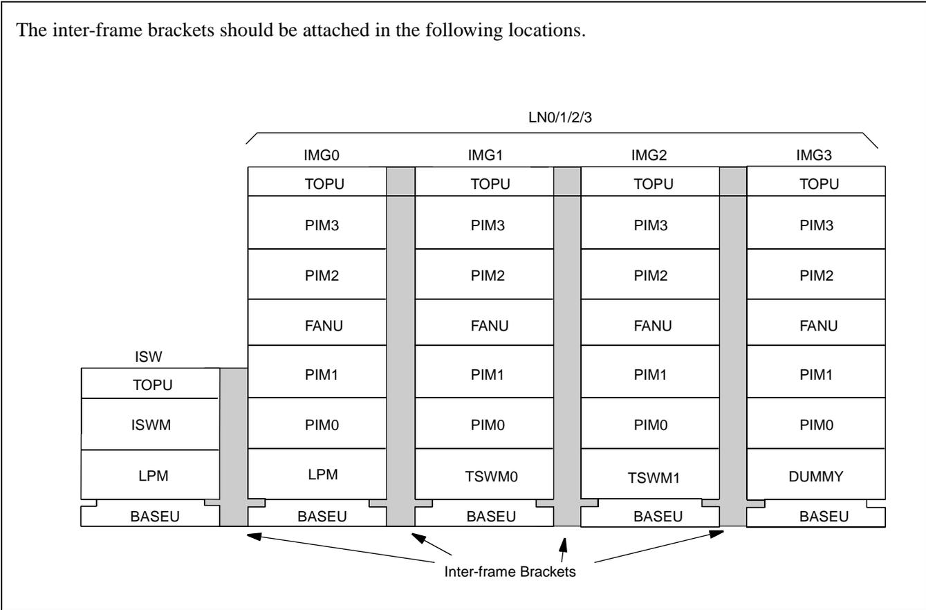
Figure 7-12 Locations of Inter-frame Brackets
