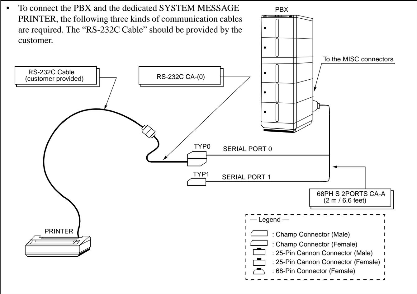
Figure 016-4 Connection of System Message Printer
