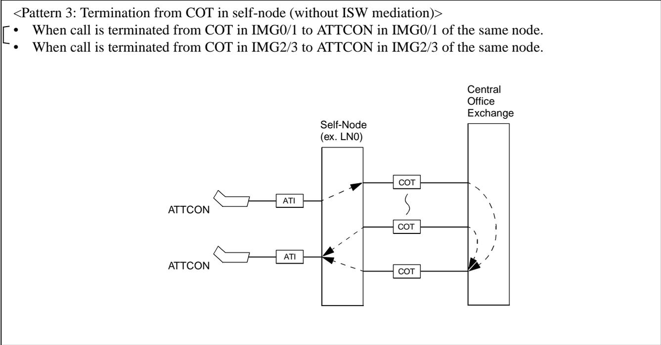
Figure 043-1 Overall Test for C.O. Line Incoming Call (2/2)
