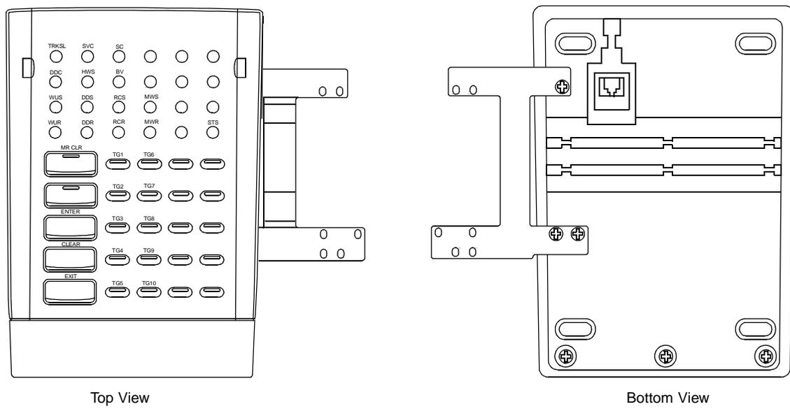
2. Mount the ADD-ON CONSOLE to DESK CONSOLE with three screws as shown below.
