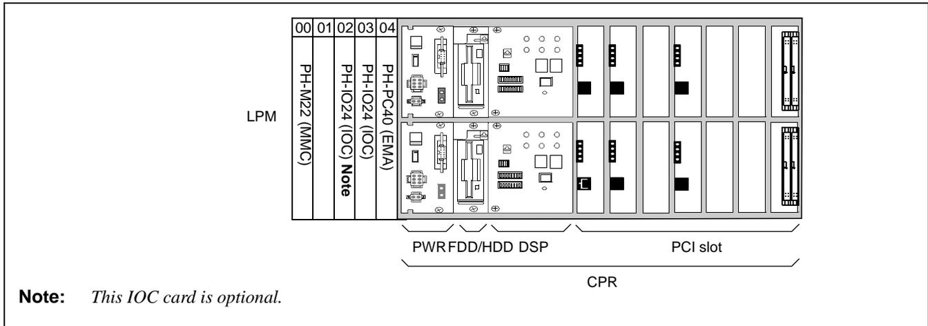
Figure 2-14 Controlling Circuit Cards in LPM (ISW)
