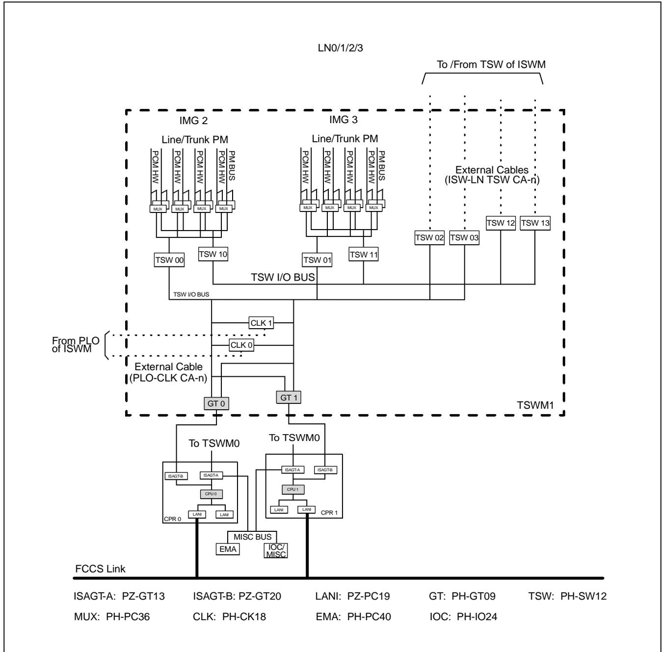
**Figure 025-7 System Block Diagram for LN Switching Network (2/2)**
