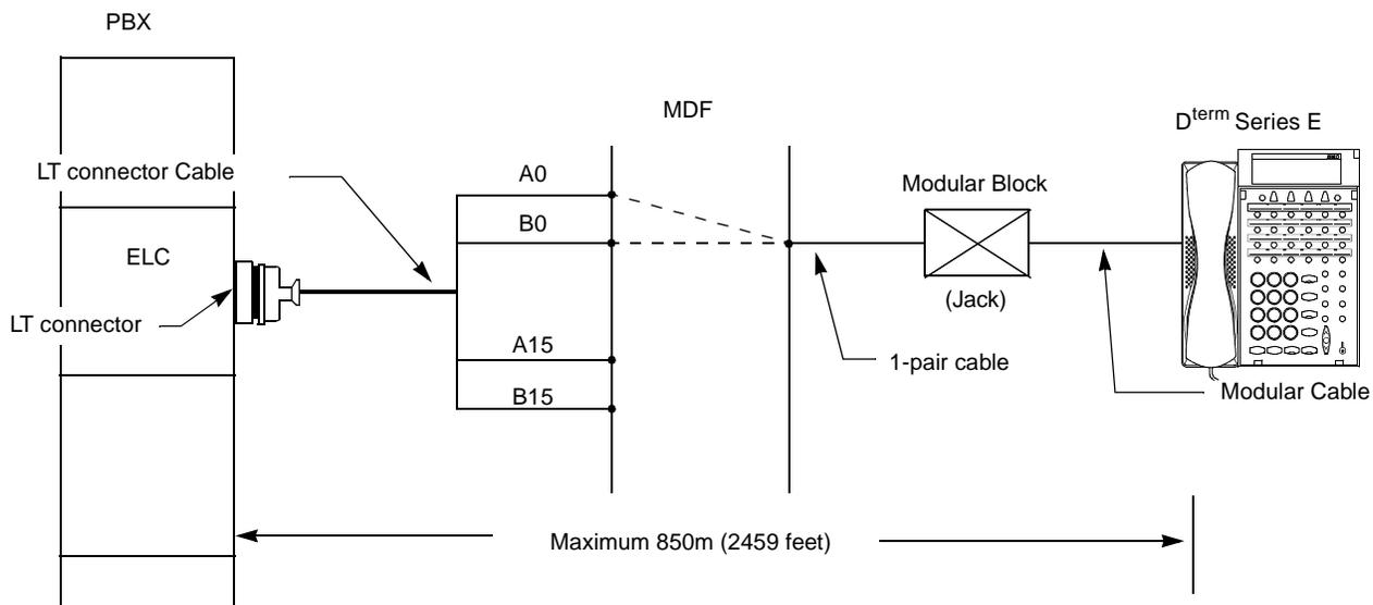
Figure 014-13 Cable Connection for D<sup>term</sup> Series E
