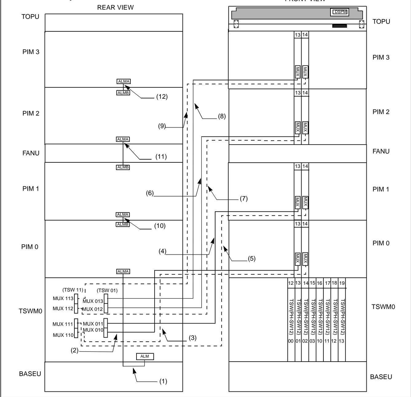
Figure 010-15 Internal Bus Cable Connection for IMG1
