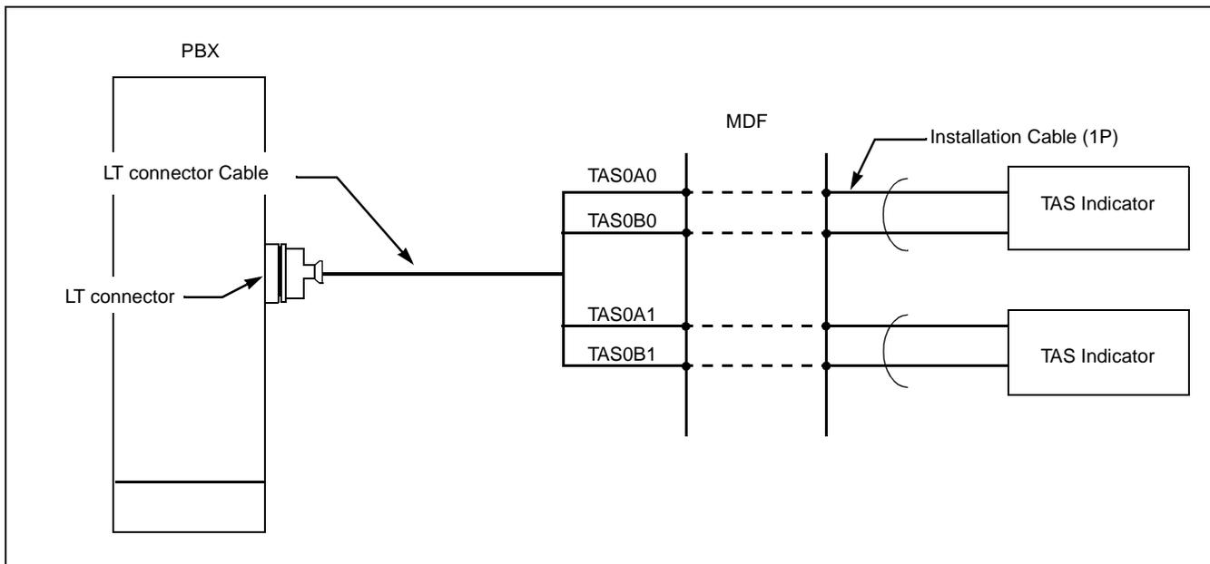
Figure 014-7 Cable Connection Diagram for TAS (Continued)
