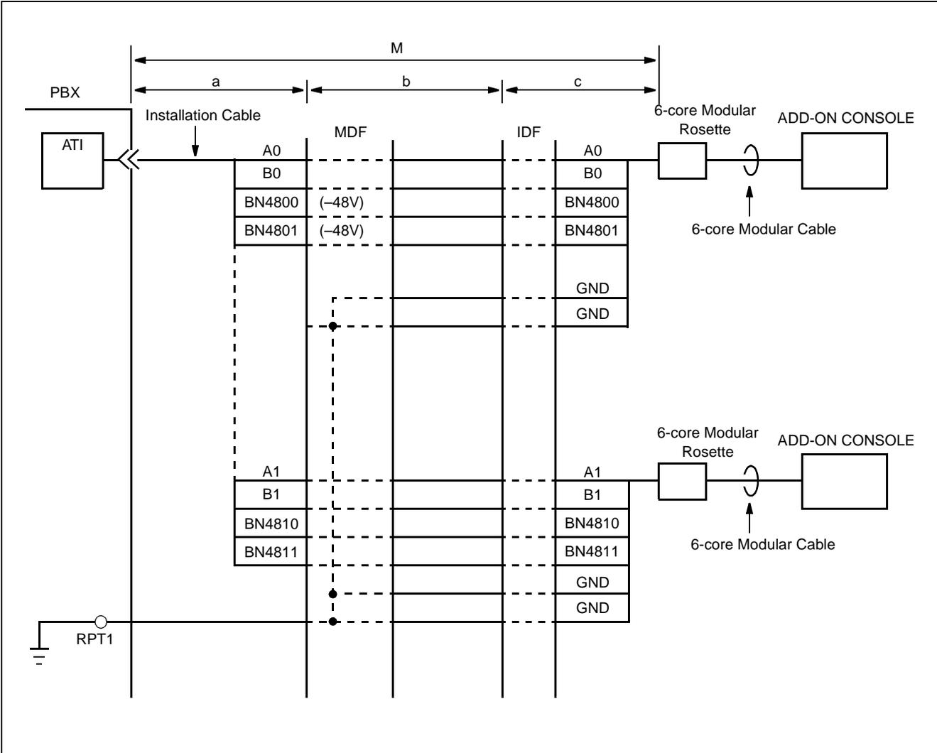
**Figure 015-14 Add-On Console Cable Connection Diagram (When the power is supplied from the PBX)**
