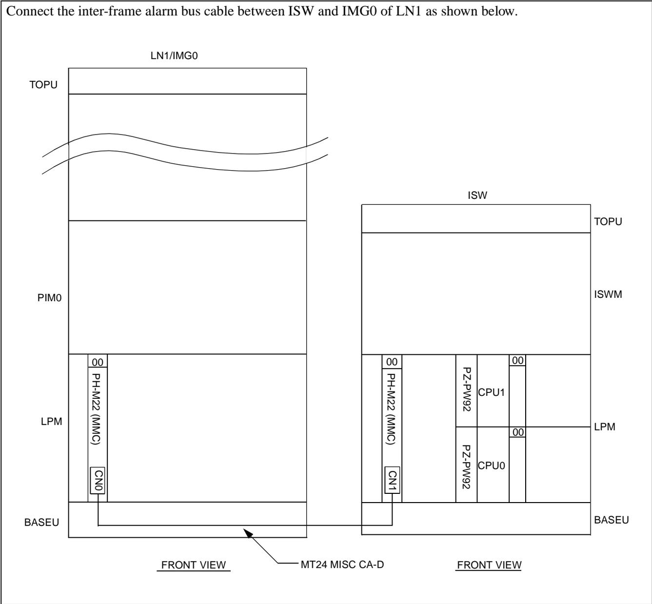
Figure 010-27 Inter-frame Cable Connection for ISW-LN1, IMG0
