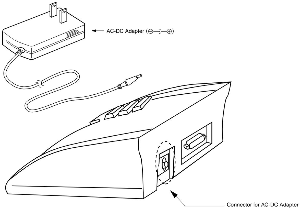
**Figure 015-18 Connection of AC-DC Adapter for Add-On Console**
