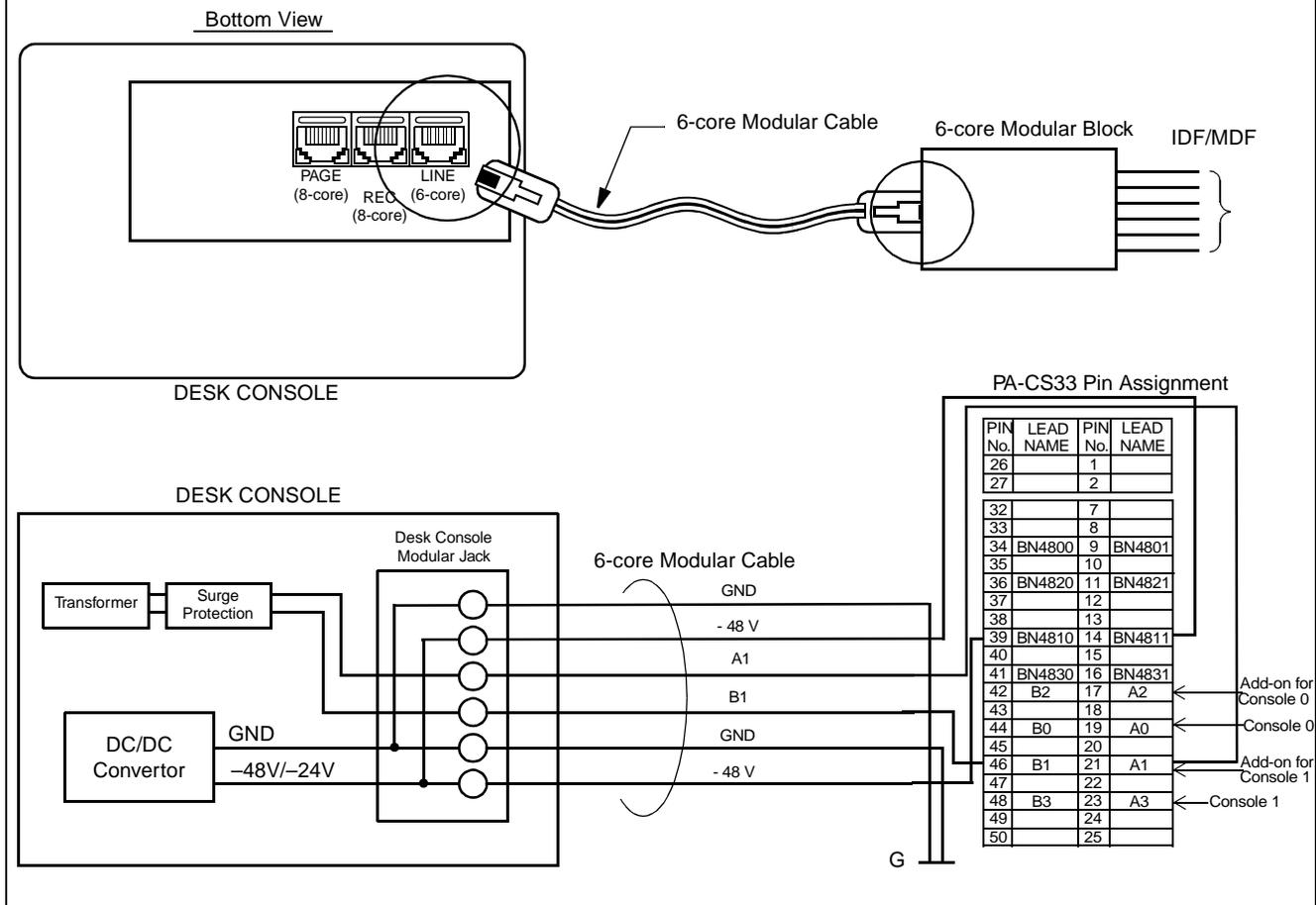
Figure 015-15 Cable Connection Diagram for Add-On Console Modular Block
