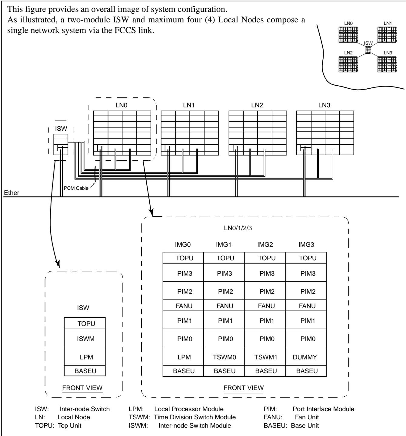
Figure 2-4 System Configuration
