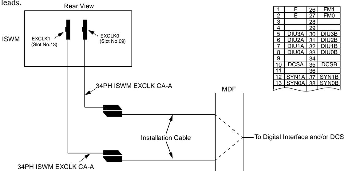
Figure 014-14 PLO Pin Assignment for Receiving Clock (ISW)
